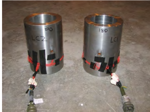
Fig. C.2 Load cells with 300 kip (1335kN) capacity each.
