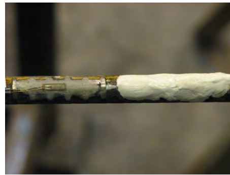
(b) Strain gages coated with wax (left) and SB tape (right)
