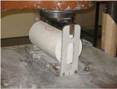
(a) Splitting strength test setup
