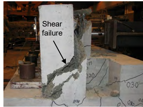
(f) At failure, west side
