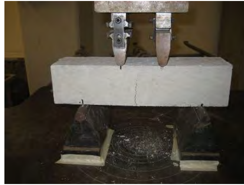
(b) Modulus of rupture test setup
