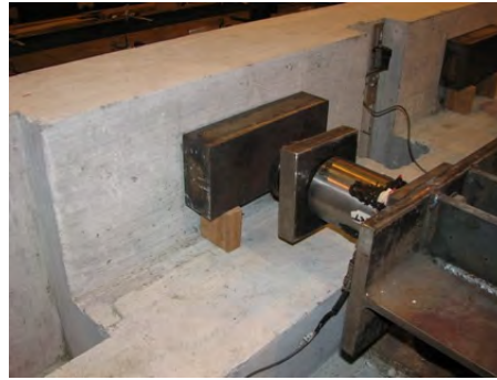
Fig. 6.1 Bearing plate detail of specimen S3.
