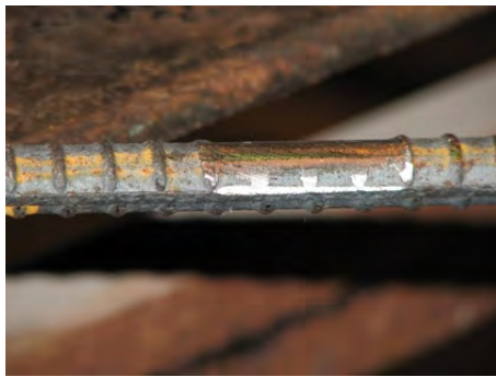
(a) Preparation of bar surface
