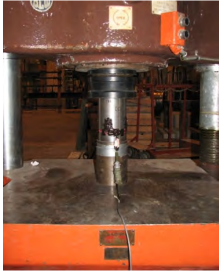
Fig. C.3 Load cell calibration setup.
