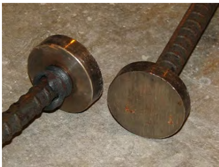
(a) Friction welded (#4 and larger bars)
