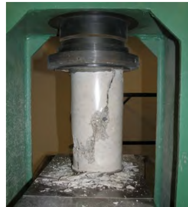
(b) Tested concrete cylinder
