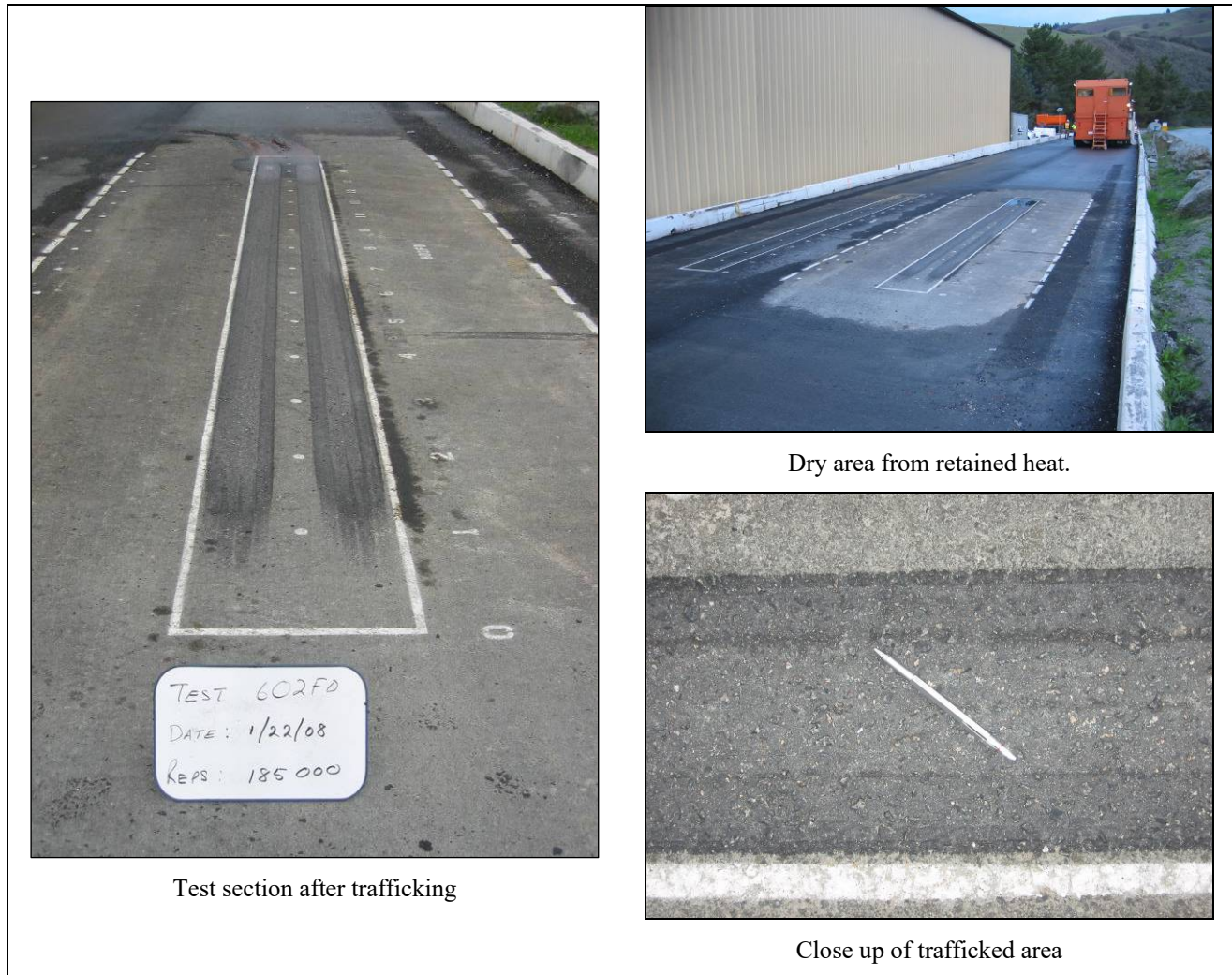
Figure 4.28: 602FD: Section photographs at test completion.
