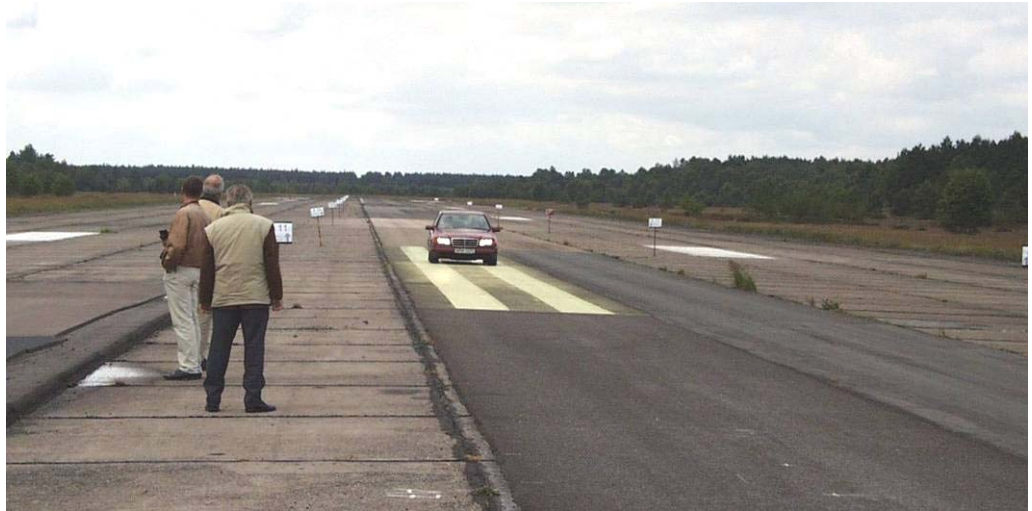
Figure 1.4. A Mercedes passenger car on the Sperenberg pavement test site with 46 different pavements on a closed military airport near Berlin in Germany.
