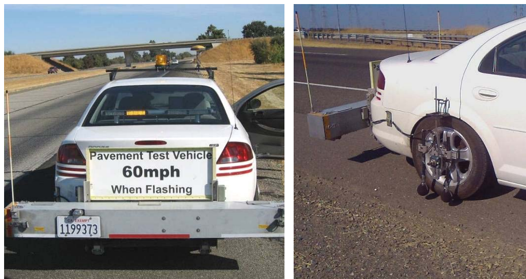
Figure 3.1. The UCPRC OBSI measurement vehicle.
