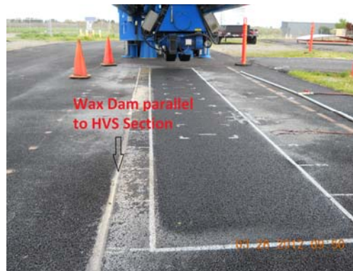
(b) Ponding of water with a wax dam parallel to the test section at the down slope side
