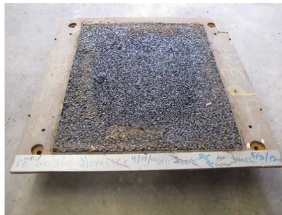
(b) Finished ingot specimen in the mold
