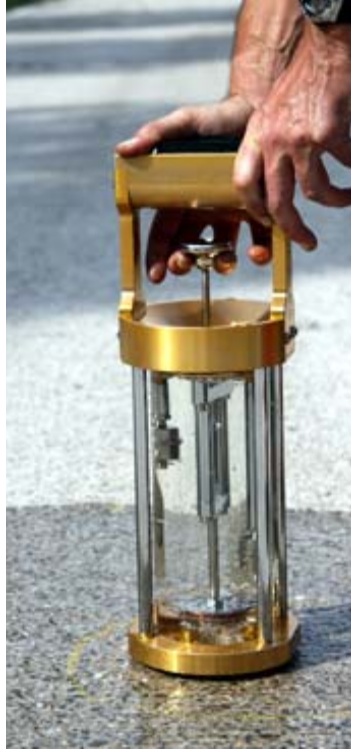
Figure 3.20: Outflow Meter. (Courtesy of KLARUW Systems.)
