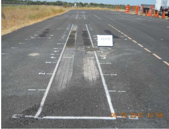
(a) Section 655HB, tested with dual wheels
