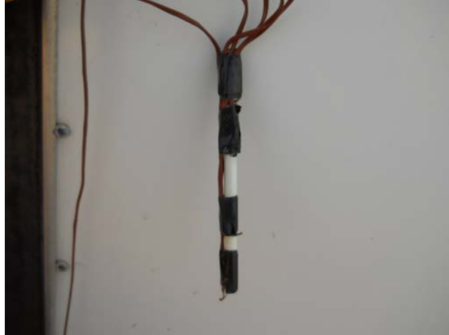
Figure 3.6: A “thermocouple tree” consisting of five Type-K thermocouples wrapped on a plastic dowel.
