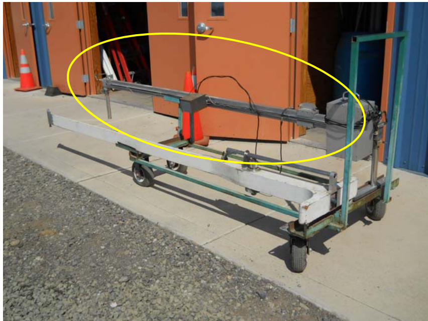
Figure 3.7: The laser profilometer.
