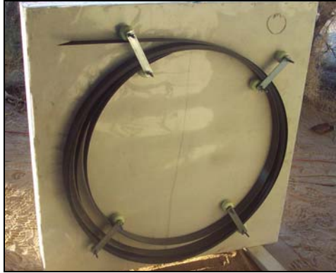
Figure 8.1. Pultruded CFRP Composite Roll
