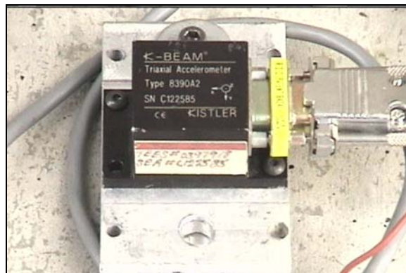
Figure 7.11. Accelerometer Attached to Watson Wash Bridge Structure
