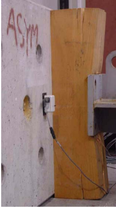
FIGURE 2-8 Component experiment on 4 foot long 12x12 in. timber corbel
