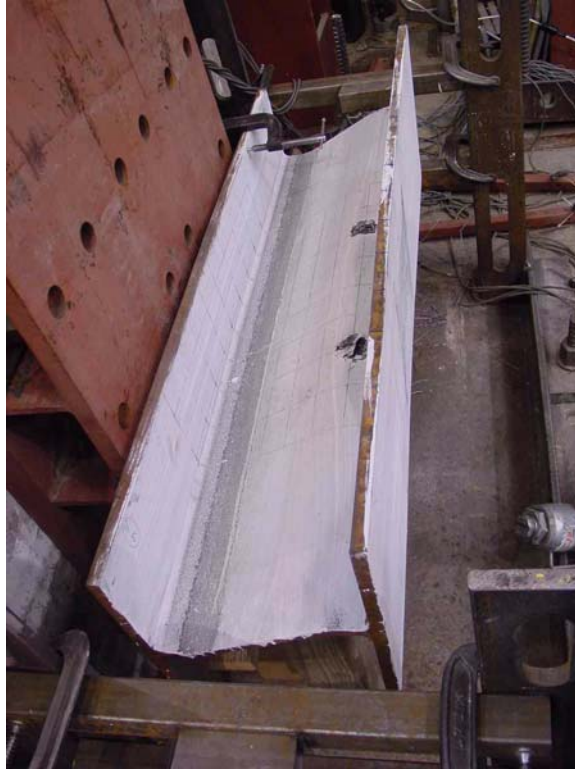
FIGURE 2-52 Lateral Buckling of 1490TPNBNCNRE0 - Beam 26
