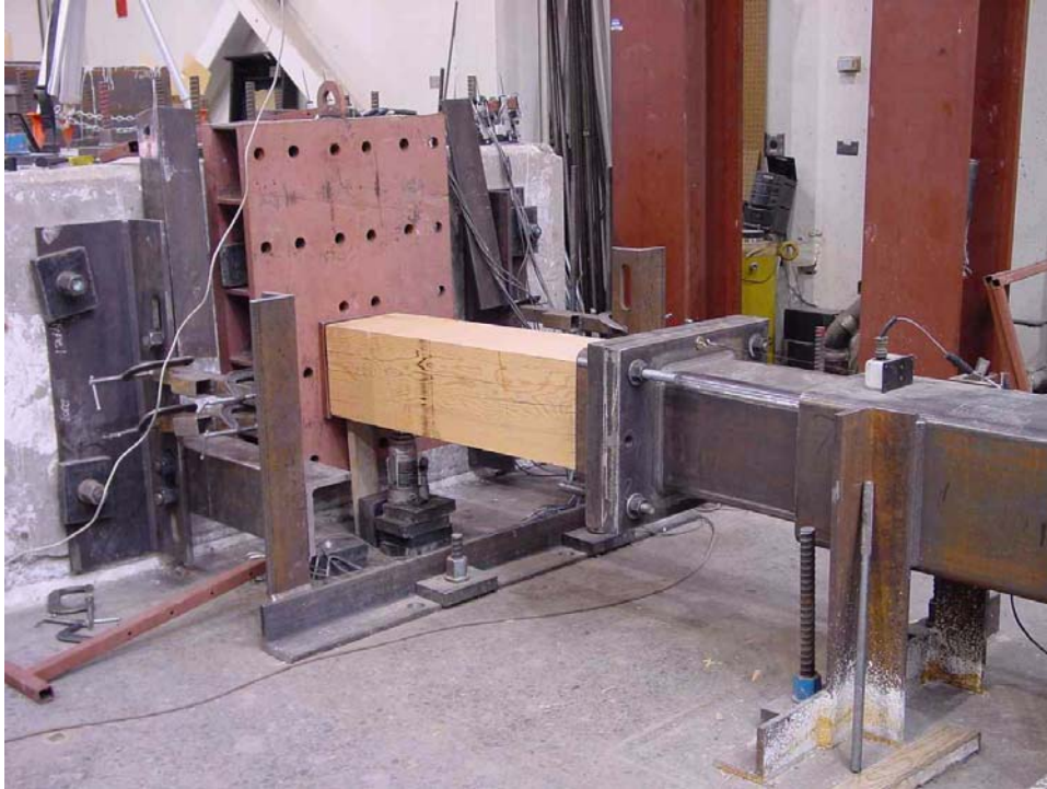
FIGURE 2-5 Component experiment on 4 foot long 12x12 in. Timber Post
