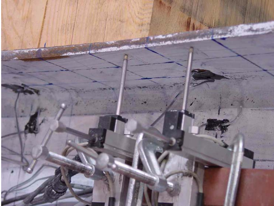
FIGURE 2-16 Strain gages on beam close to where flaking of lime paint is first observed
