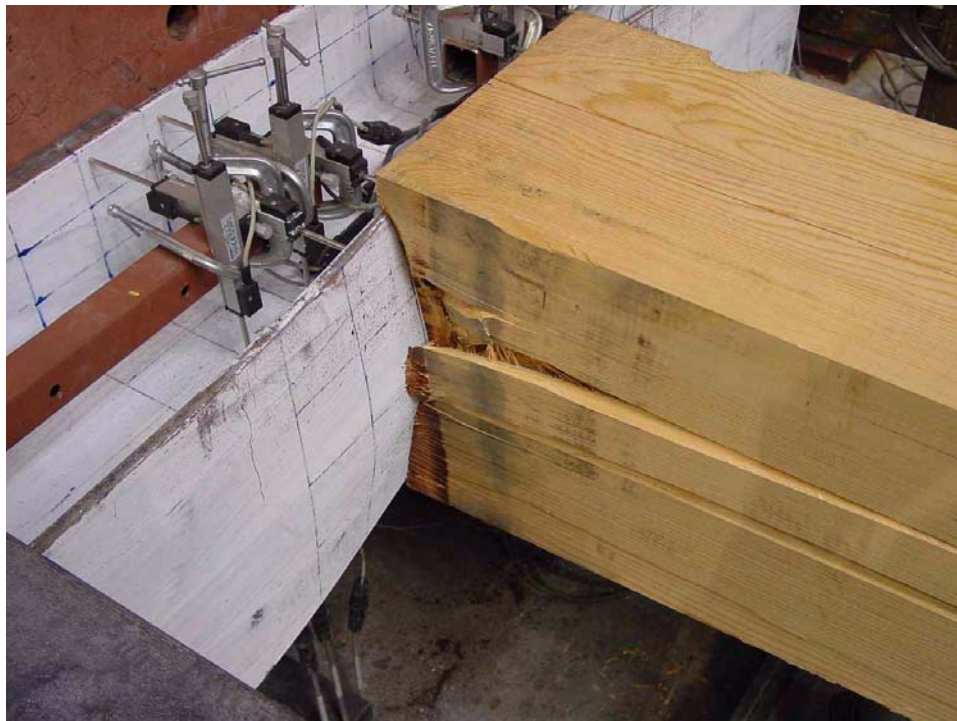
FIGURE 2-15 Flange bending and post deformation observed during loading of 1253TPNBSCRE0 - Beam 18
