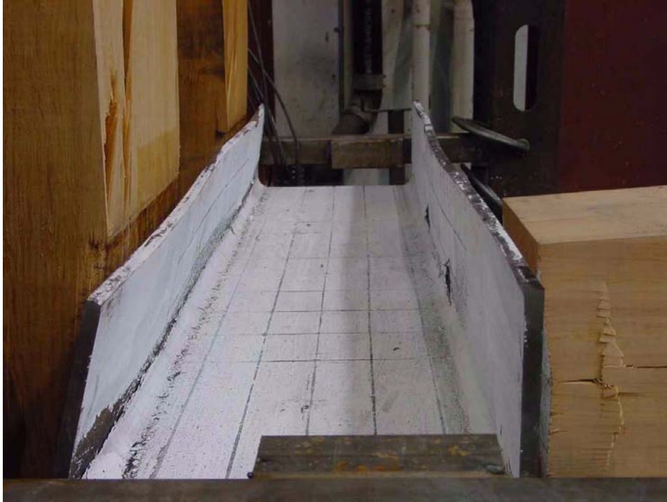
FIGURE 2-32 Corbel-flange bending, corbel crushing and post crushing after the completion of 1253TPNBTCRE0 - Beam 12
