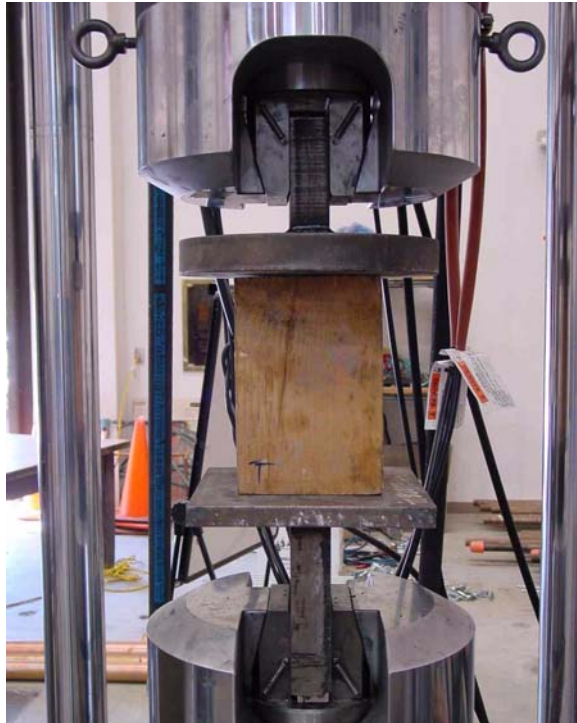
FIGURE 2-10 Component experiment on blocking in load frame
