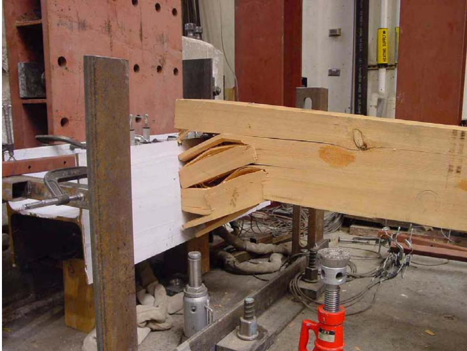
FIGURE 2-48 Failure of post during experiment on unrestrained beam 1473TPNBNCNRE6 - Beam 31
