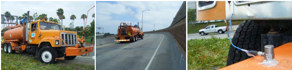
Figure 9. Water truck driven over the WSO bridge during the traffic controlled tests.
