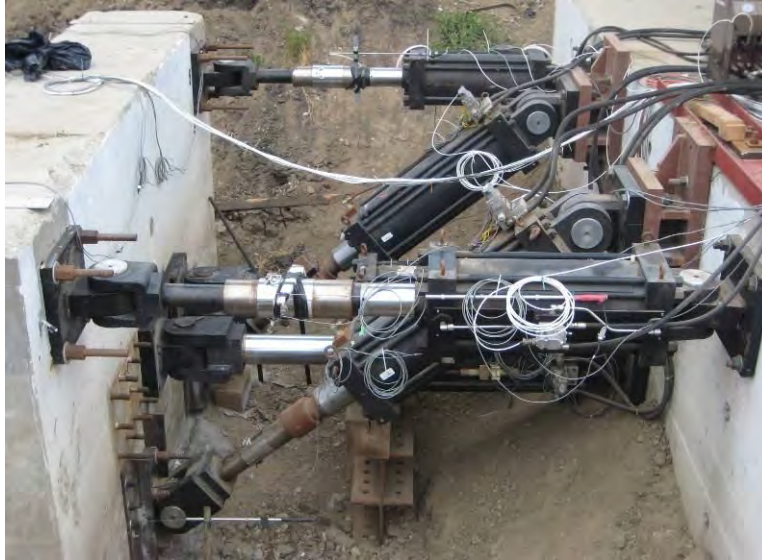
Figure 3.6 Photograph of actuator configuration (Elevation view from North)
