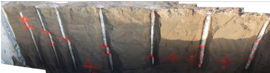
Figure 5. 38 Combined images of backfill excavation and gypsum column ruptures for T8.0-2
