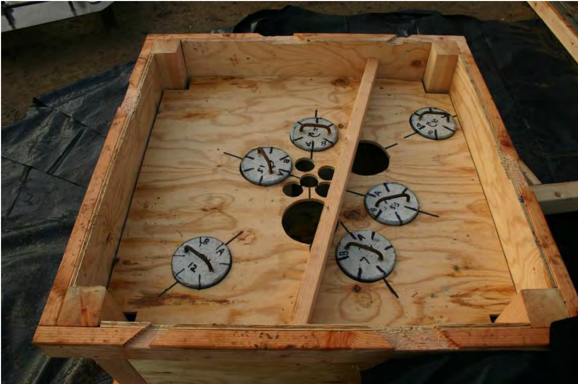
Figure 3.4 - Photograph of the Frame Apparatus used to Secure Cylindrical Test Cylinders
