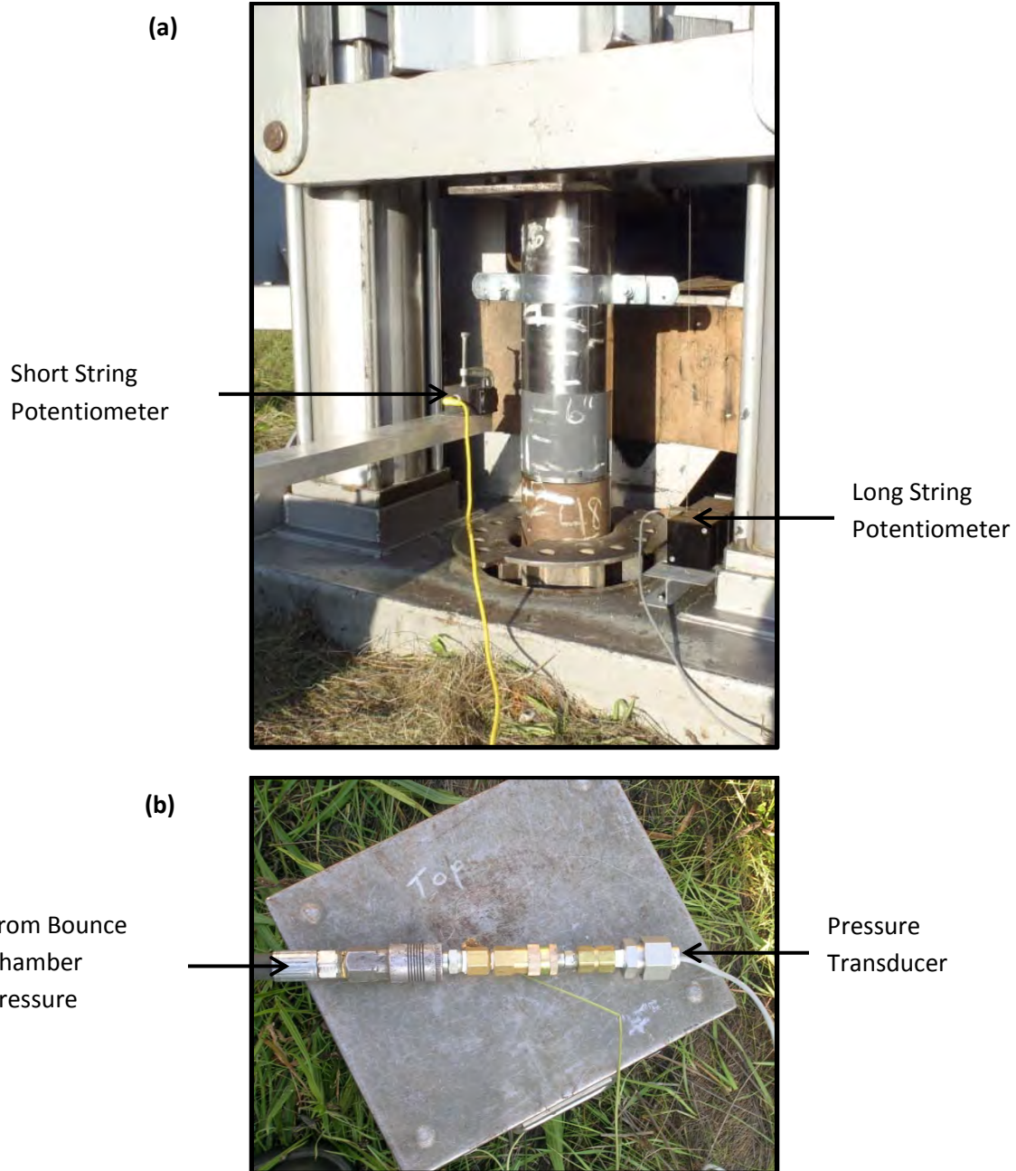
Figure 3.10: Pictures of above ground sensors in field applications. (a) String potentiometer mounting for pullout load testing and (b) connection between pressure transducer and bounce chamber.
