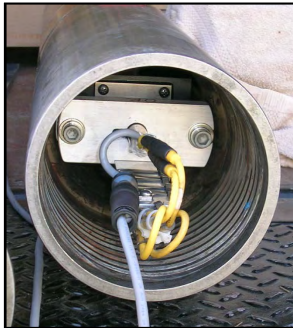
Figure 3.8: (a) Picture of GST units filled with epoxy and curing in the laboratory and (b) picture of GST module assembled inside the pipe section.
