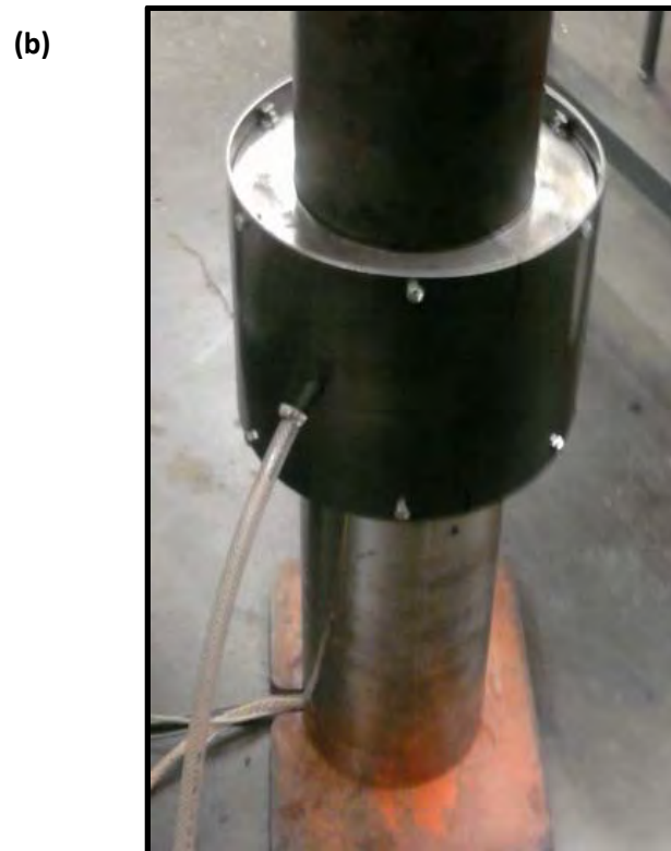
Figure 3.23: (a) Bladder and calibration chamber assembly on thin wall cylinder to calibrate radial stress measurement. Teflon sheet and baby powder used to reduce friction and apply uniform pressure. (b) Inner tube inflated to desired pressures through air pressure regulator.
