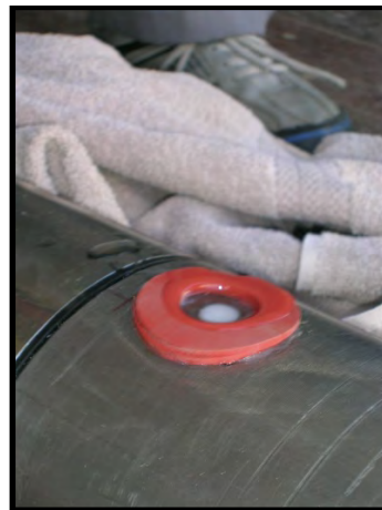
Figure 3.6: Pictures of porous filter saturation process before driving. (a) Porous hole of RTP unit is in upright position with a washer sealing, (b) silicon oil is filled in the cavity between pore pressure surface and RTP outer wall using a needle, (c) surface mount vacuum applied to remove air pockets, and (d) saturated porous stone in place.
