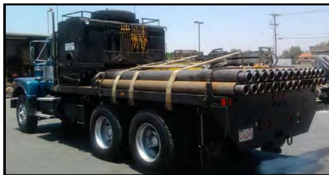
Figure 2.18: Becker hammer drill system (a) moving Becker drill rig, (b) Drill ring with driving hammer in upward right position, and (c) Becker pipes being transported to field site.
