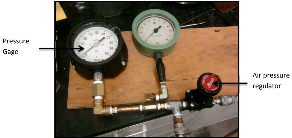
Figure 3.24: Air pressure regulator and measurement gauges used in the calibration process.
