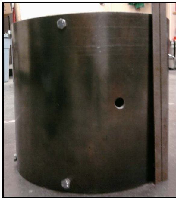
Figure 3.22: Radial stress calibration chamber that contains a bladder that expands between inner wall of the calibration chamber and RTP's thin wall cylinder for radial stress measurement. (a) Top view and (b) side view.
