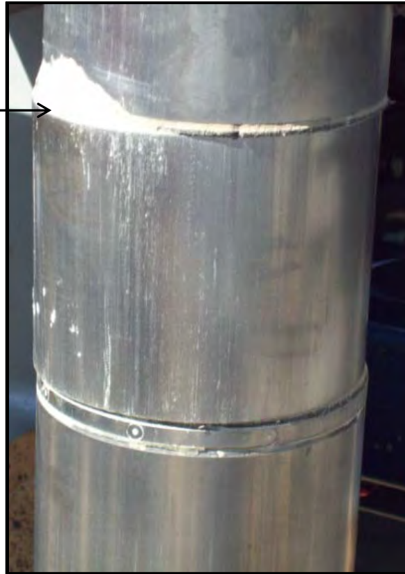
Figure 3.20: Picture of damaged thin walled cylinder of instrumented section after hard driving condition encountered at Fontana, CA test site.
