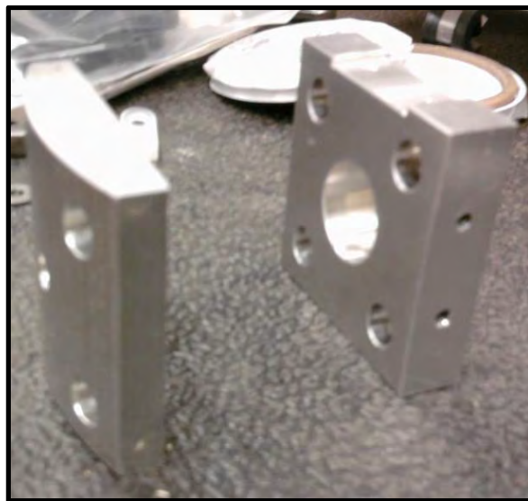
Figure 3.5: Acceleration and pore pressure mounting system. (a) Acceleration and pore pressure module assembly against inner RTP wall and (b) picture of bulkhead components.
