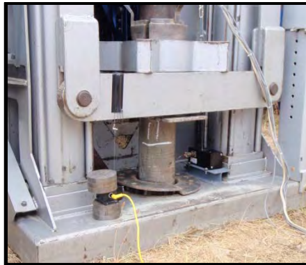
Figure 3.15: Pictures from field performance testing. (a) Hard wired RTP section connected to driving shoe, (b) driving shoe and RTP section assembly connected to regular Becker pipe section, (c) RTP string being driven into ground, and (d) pullout load testing in progress.
