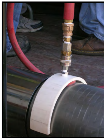
Figure 3.6: Pictures of porous filter saturation process before driving. (a) Porous hole of RTP unit is in upright position with a washer sealing, (b) silicon oil is filled in the cavity between pore pressure surface and RTP outer wall using a needle, (c) surface mount vacuum applied to remove air pockets, and (d) saturated porous stone in place.
