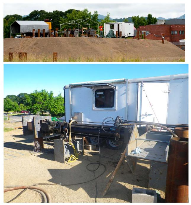
**Figure 4-18.** Top: Constructed Embankment and Test slope Bottom: Test Pile, Reaction Piles, and Hydraulic Actuator Set up
