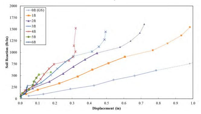
**Figure 12-2** Back-Calculated *p-y* Curves for the -Baseline Pile (P-2) with Lower Displacements Note: Dotted Lines Present Data after Initial Pile Yielding
