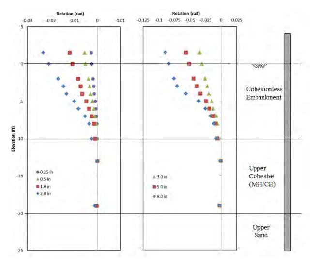
Figure 11-13 Rotation Results for the 0D Pile (P-9) at varying Displacements
