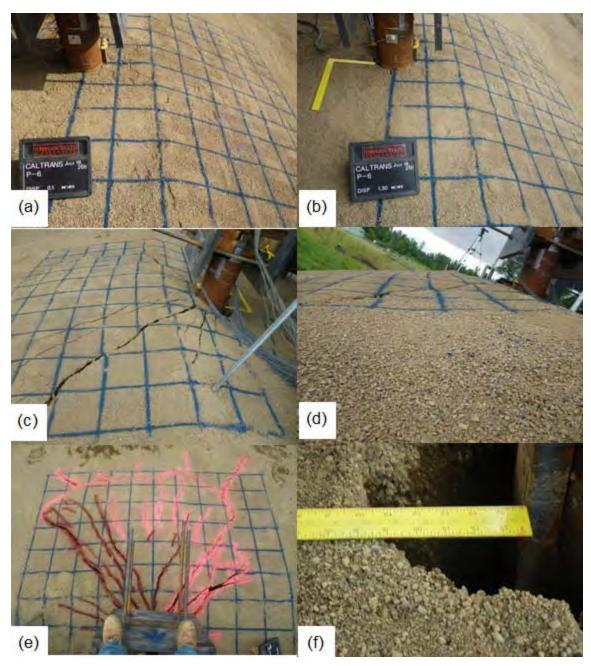
**Figure 10-2** Observations during lateral loading testing of pile P-5 (2D) a) Pile before loading b) Pile at 1.5" of displacement with cracks forming c) Pile at 8.0" of displacement with passive wedge cracking d) Passive wedge movement on slope e) Passive wedge movement in front of pile at end of testing f) Gap formation behind pile
