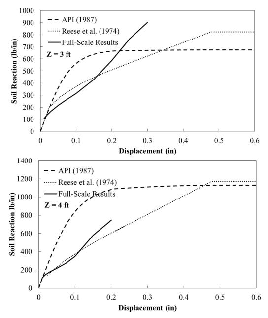
**Figure 13-8** Comparison of the API (1987), Reese et al. (1974) predicted baseline p-y curves with full-scale results at depths of 3 ft (top) and 4 ft (bottom)
