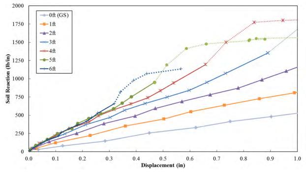
**Figure 12-14** Back-Calculated *p-y* Curves for the 0D Pile (P-9) Showing Lower Displacements Note: Dotted Lines Present Data after Initial Pile Yielding
