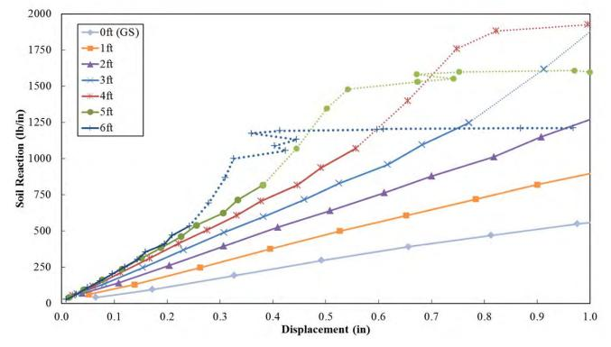
**Figure 12-10** Back-Calculated *p-y* Curves for the 2D Pile (P-6) Showing Lower Displacements Note: Dotted Lines Present Data after Initial Pile Yielding
