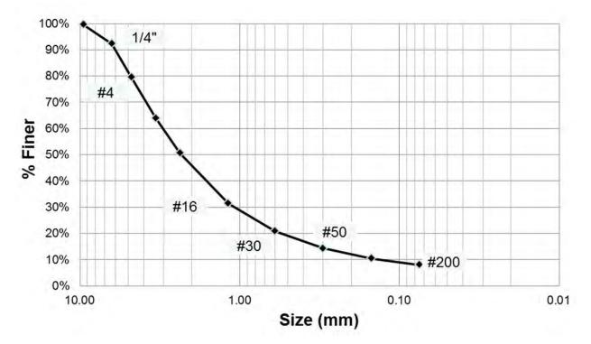
Figure 3-6. Gradation Curve of the Cohesionless Material used in Series-II
