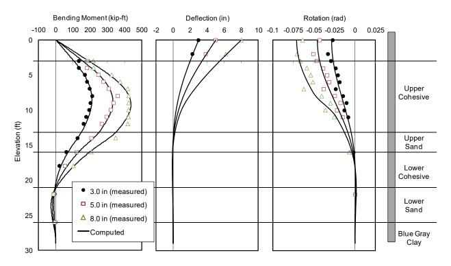
**Figure 7-17**. Comparison of Test Results and Analysis Using Back-Calculated *p-y* Curves for 0D Pile (I-7) for Pile Head Displacement of 3.0, 5.0 and 8.0 in.
