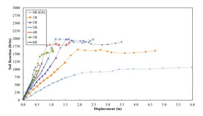
**Figure 12-13** Back-Calculated *p-y* Curves for the 0D Pile (P-9) (On Crest) Note: Dotted Lines Present Data after Initial Pile Yielding
