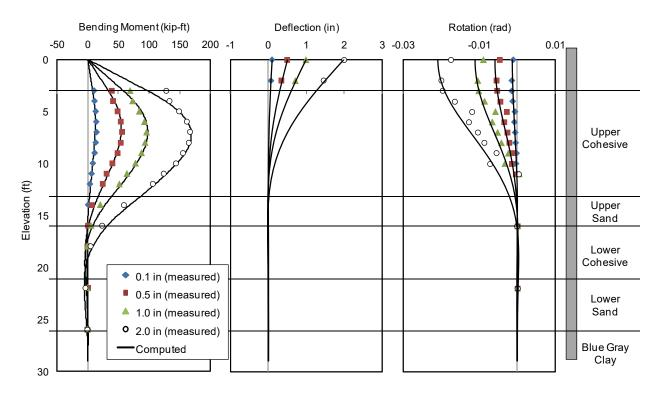
**Figure 7-12.** Comparison of Test Results and Analysis Using Back-Calculated *p-y* Curves for 4D Pile (I-5) for Pile Head Displacement of 0.1, 0.5, 1.0 and 2.0 in.
