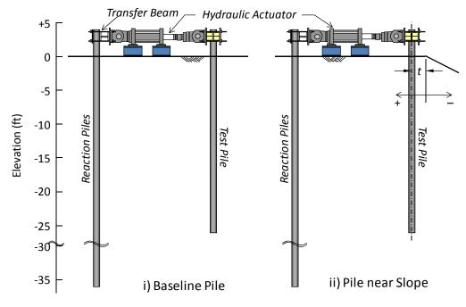
Figure 4-1. Transversal View of Test Set-Ups
