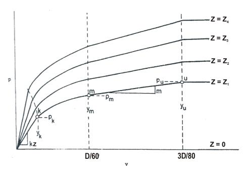
Figure 2-14 Characteristic Shapes of *p-y* Curves for Sand (Reese *et al.* 1974)
