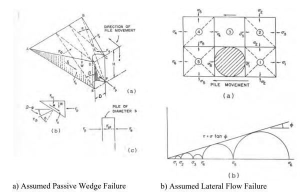
**Figure 2-13** Sand Failure Modes in Laterally Loaded Pile Problem a) Assumed Passive Wedge Failure; b) Assumed Lateral Flow Failure (after Reese *et al.* 1974)
