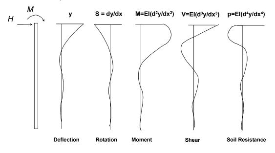
Figure 2-4 Methodology in Developing *p*-*y* Curves (after Reese and Van Impe 2001)
