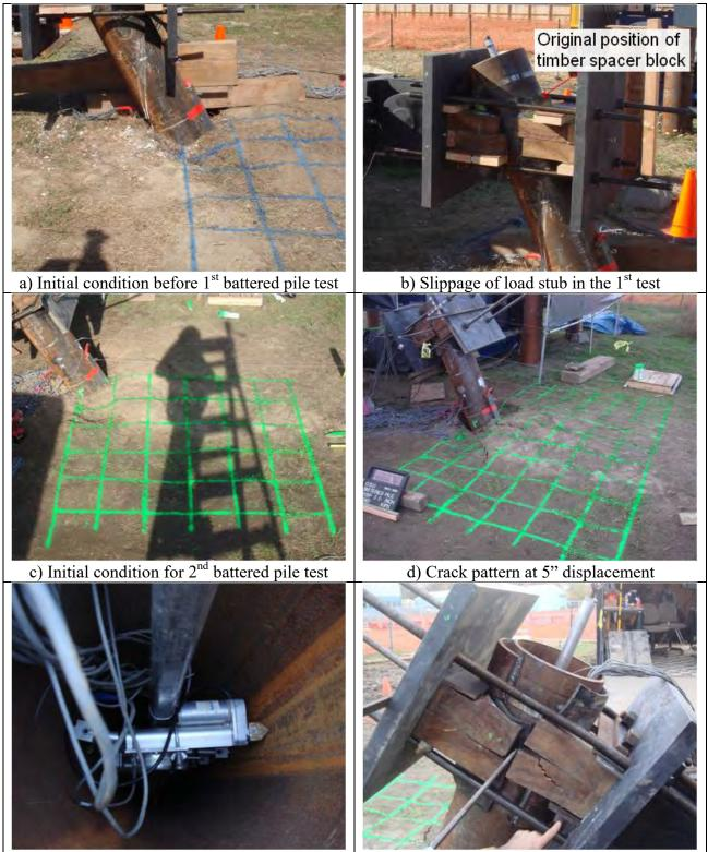
e) Bent actuator rod due to section deformation f) Significant cracks on timber spacer blocks Figure 5-8. Observations from Both Lateral Load Tests for Battered Pile (I-3)
