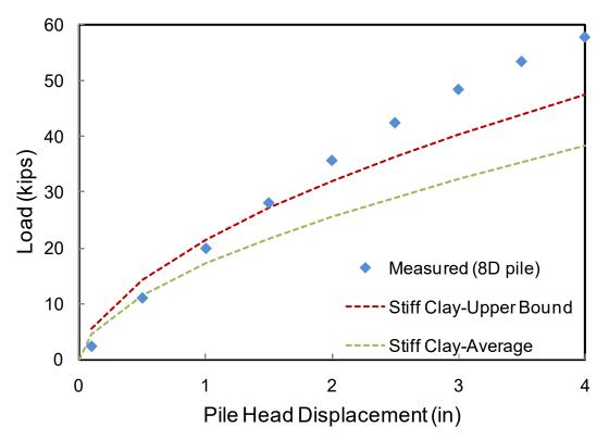
Figure 8-2. Comparison of Load-Displacement Curve Using Stiff Clay p-y Curves and Measured Results from 8D pile
