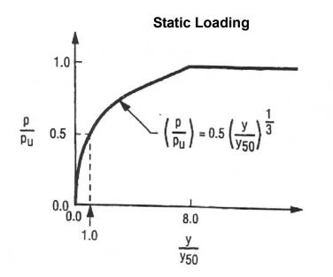
**Figure 2-8** Characteristic Shape of *p-y* Curve for Soft Clay for Static Loading (after Matlock 1970)
