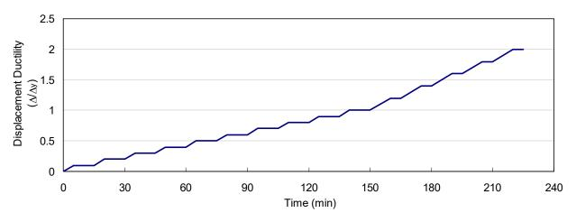
Figure 4-15. Load Protocol for Pseudo Static Lateral Load Tests
