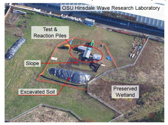
Figure 3-2. Aerial View of the Cohesive Test Site Relative to Hinsdale Wave Research Lab
