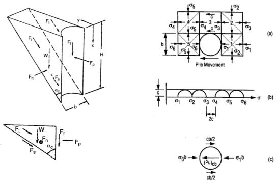
a) Assumed Passive Wedge Failure
