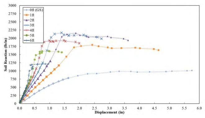
**Figure 12-9** Back-Calculated *p-y* Curves for the 2D Pile (P-6) Note: Dotted Lines Present Data after Initial Pile Yielding
