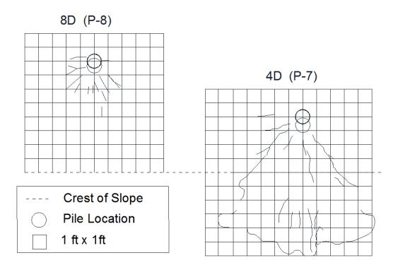
Figure 10-11 Cracking Patterns for the 8D And 4D Test Piles
