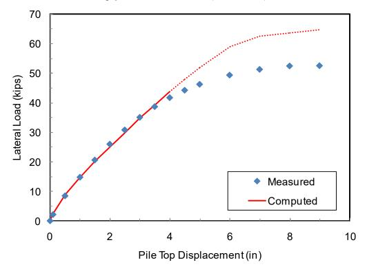
**Figure 7-15.** Comparison of Load-Displacement Curves from Test Results and Analysis Using Back-Calculated *p*-*y* Curves for 0D Pile (I-7)
