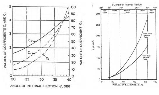
a) Coefficients as Function of  $\varphi$  for API Sand
