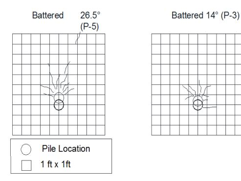
Figure 10-13Cracking Patterns for the +26° and +14° battered test piles
