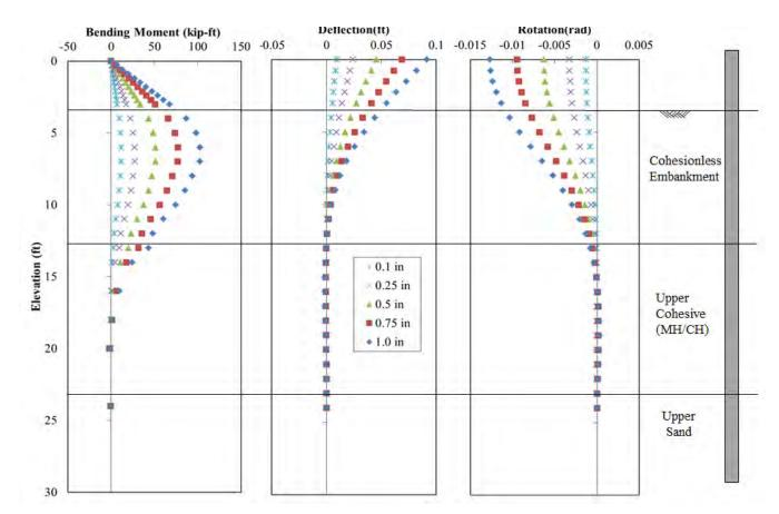
**Figure 12-11** Comparison of Test Results and Analysis Using Back-Calculated *p-y* Curves for the 2D (P-6) for Pile Head Displacement of 0.1, 0.25, 0.5 and 1.0 in.
