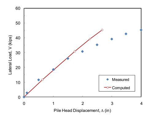
Figure 9-11 Comparison of Load-Displacement Curve from Test Results and FEM Analysis for the 2D Pile
