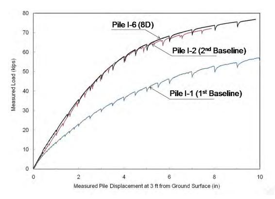
**Figure 6-1.** Comparison of Load-Displacement Curves between Baseline Piles (I-1 and I-2) and Pile at 8D from the Slope Crest (I-6)
