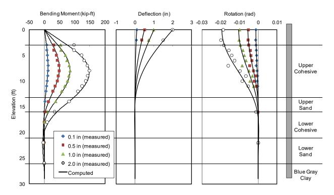
**Figure 7-16.** Comparison of Test Results and Analysis Using Back-Calculated *p-y* Curves for 0D Pile (I-7) for Pile Head Displacement of 0.1, 0.5, 1.0 and 2.0 in.
