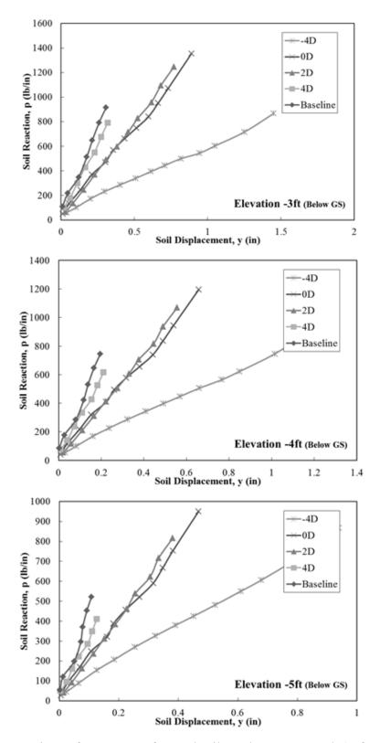
Figure 12-22 Comparison of *p*-*y* Curves for Each Pile at the Same Depth (-2ft to-5ft)
