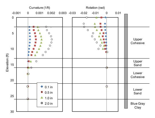
Figure 6-9. Test Results of 4D pile (I-5) for Pile Head Displacement of 0.1, 0.5, 1.0 and 2.0 in
