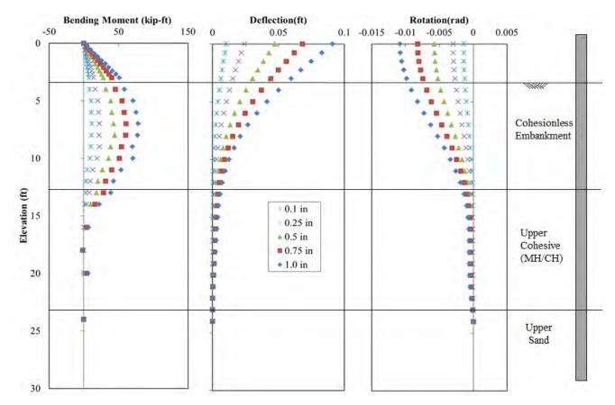
**Figure 12-19** Comparison of Test Results and Analysis Using Back-Calculated *p-y* Curves for the -4D (P-10) for Pile Head Displacement of 0.1, 0.25, 0.5 and 1.0 in.
