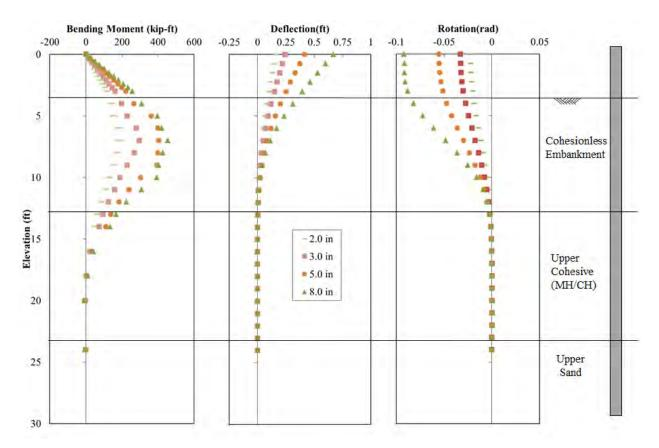
**Figure 12-16** Comparison of Test Results and Analysis Using Back-Calculated *p-y* Curves for the 0D Pile (P-9) for Pile Head Displacement of 2.0, 3.0, 5.0 and 8.0 in.
