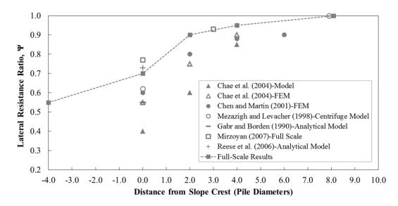
Figure 13-14 Comparison of resistance ratios presented by researchers as a function of distance from a slope crest with the findings from this study
