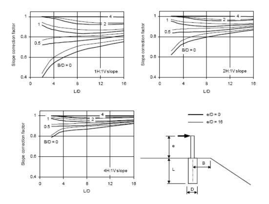
**Figure 2-25** Reduction Factors to Account for the Effect of a Slope on Pile Capacity: Frictionless pile, Weightless soil (from Stewart 1999)
