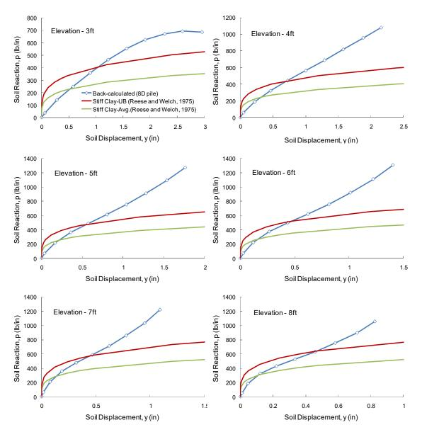
**Figure 8-1**. Comparison of Back-Calculated p-y Curves for 8D Pile (I-6) to Stiff Clay p-y Curves (Reese and Welch, 1975) for Elevation 3ft (GS) to 8ft
