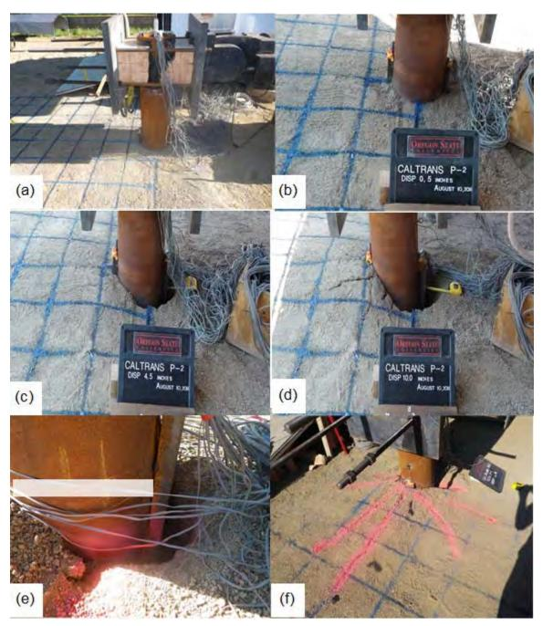
Figure 10-1 Observations during load test of first and second baseline piles a) Pile before loading b) Pile at 0.5" of displacement c) Pile at 4.5" of displacement d) Pile at end of testing e) Gap formation behind pile f) Heave and cracking in front of pile
