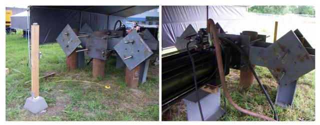
Figure 4-7. Actual test setup – Three-in-a-row Reaction Pile Arrangement
