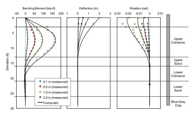
**Figure 7-4.** Comparison of Test Results and Analysis Using Back-Calculated *p*-*y* Curves for 8D Pile (I-6) for Pile Head Displacement of 0.1, 0.5, 1.0 and 2.0 in.
