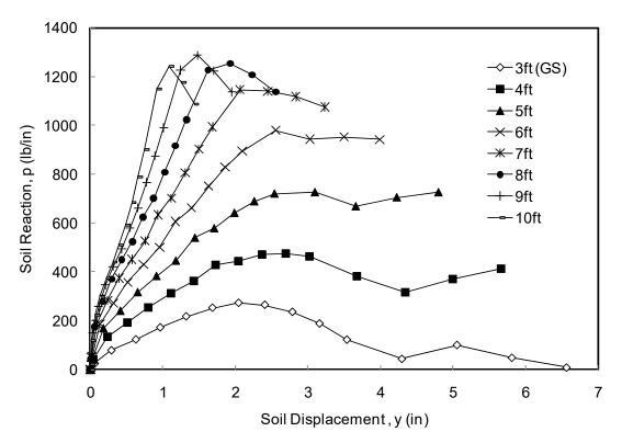
Figure 7-14. Back-Calculated *p*-*y* Curves for 0D Pile (on the crest)
