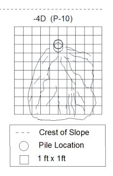
Figure 10-15 Cracking Patterns for the -4D (on slope) Pile
