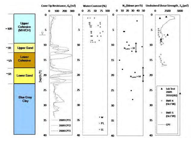
**Figure 3-4.** Summary of Site Specific Explorations for Caltrans Pile Load Study (as of March 31, 2010)
