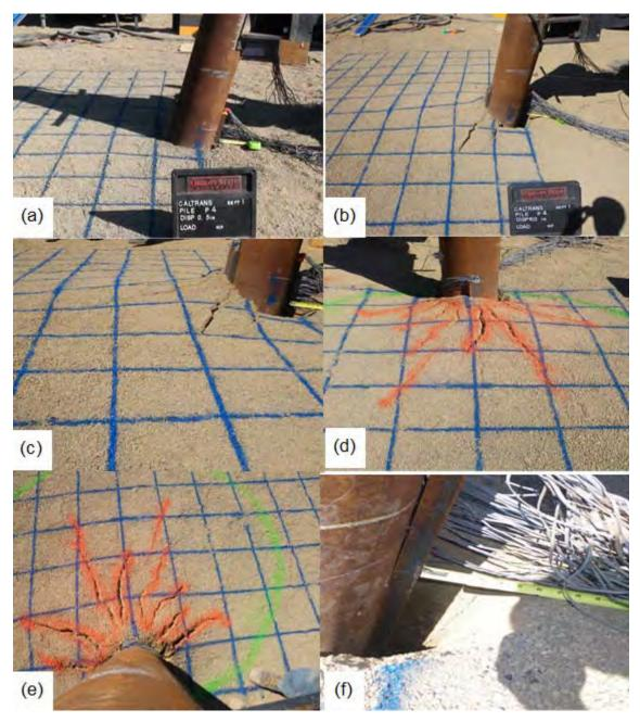
**Figure 10-8** Observations during Lateral Loading Testing of Pile P-3 (+14 Batter) a) Pile before loading b) Pile at end of testing c) Soil heave at end of testing d) Soil heave at end of testing e) Extensive cracking and heave f) Gap formation behind pile
