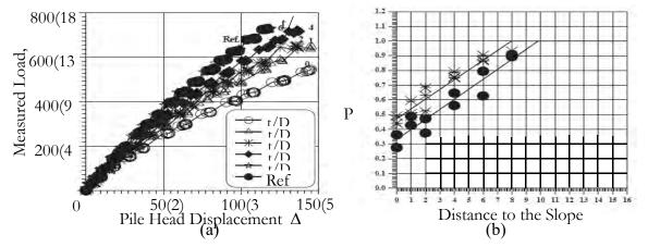
**Figure 2-22** Load Displacement Curves (a) and Recommended  $p_{mult}$  (b) for Centrifuge Tests (after Mezazigh and Levacher 1998)
