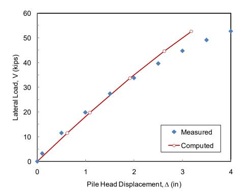
Figure 9-13 Comparison of Load-Displacement Curve from Test Results and FEM Analysis for the 4D Pile
