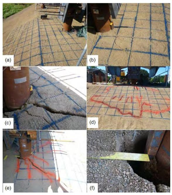
Figure 10-3 Observations during lateral loading testing of pile P-6 (4D) a) Pile before loading b) Pile at 3.5" of displacement with large cracking c) Pile at 8.0" of displacement with passive wedge cracking d) Passive wedge cracking on slope e) Passive wedge movement in front of pile f) Gap formation behind pile
