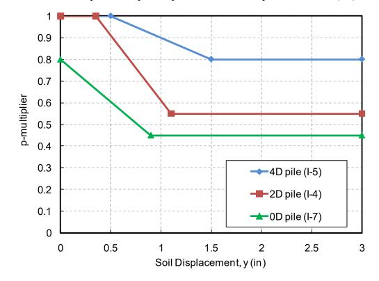
Figure 7-23. Proposed p-multiplier for Piles at Different Distances from the Slope Crest
