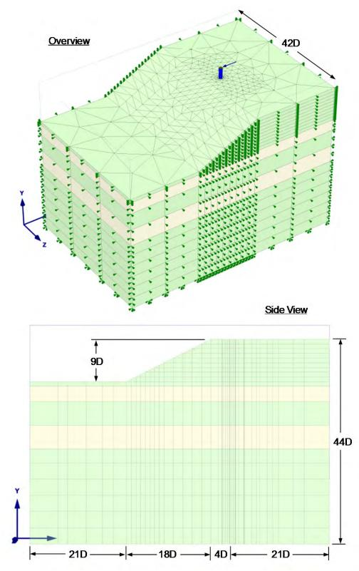
Figure 9-6 Finite Element Mesh for the 4D Pile
