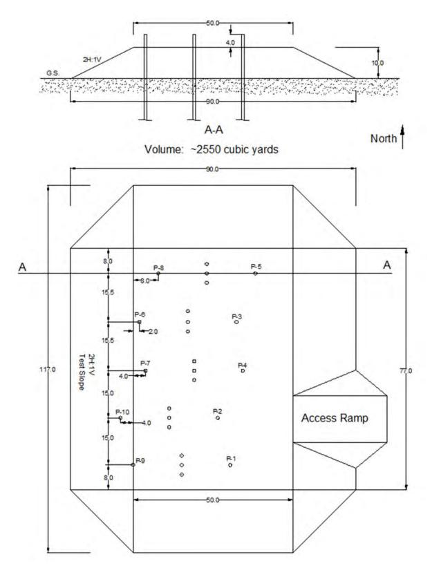
Figure 4-17. Plan and Cross-Sectional Views of the Series-II Cohesionless Embankment
