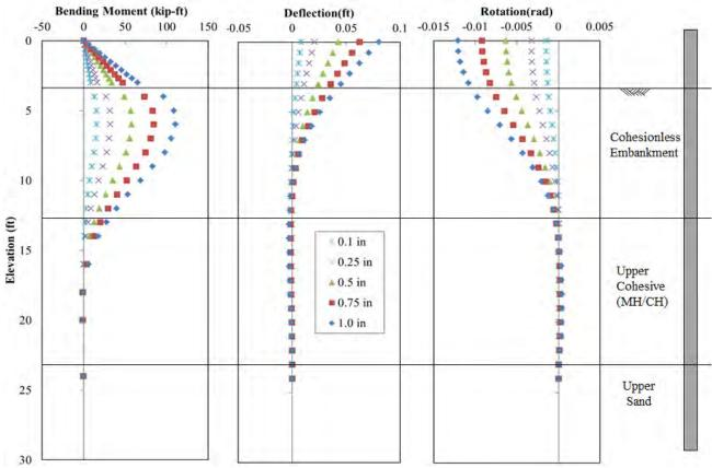
**Figure 12-3** Comparison of Test Results and Analysis Using Back-Calculated p-y Curves for the  $2^{nd}$  Baseline Pile (P-2) for Pile Head Displacement of 0.1, 0.25, 0.5 and 1.0 in.
