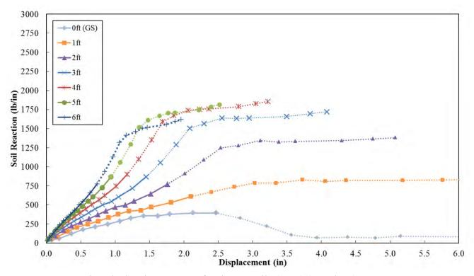
**Figure 12-17** Back-Calculated *p-y* Curves for the -4D Pile (P-10) (On Slope) Note: Dotted Lines Present Data after Initial Pile Yielding
