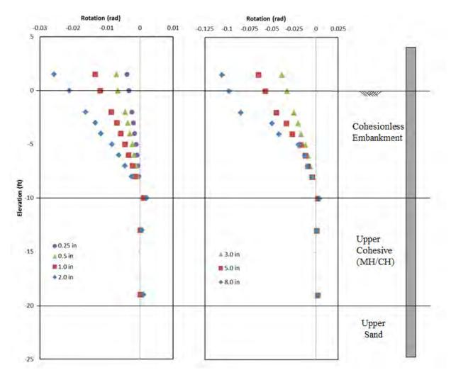
Figure 11-7 Rotation Results for the 4D Pile (P-7) at varying Displacements
