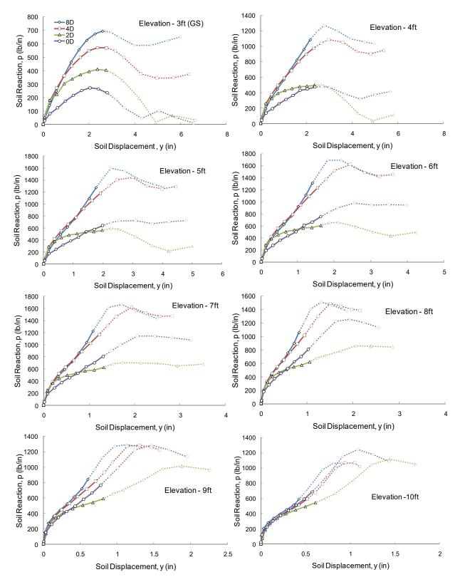
**Figure 7-18.** Comparison of *p*-*y* Curves for Piles at Different Distance from Slope Crest at Various Depths
