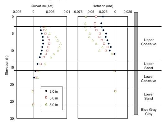
Figure 6-10. Test Results of 4D pile (I-5) for Pile Head Displacement of 3.0, 5.0 and 8.0 in
