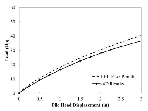
Figure 13-5 Comparison of the -4D (on slope) full-scale results with the LPILE prediction using the proposed p-multipliers for a pile on a slope
