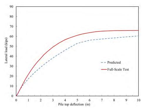
Figure 13-9 LPILE predicted 0D (slope crest) load-displacement curve with the full-scale test results
