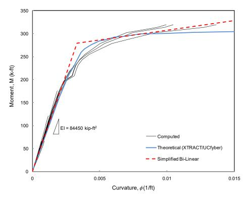
Figure 4-4. Comparison of Computed and Theoretical Moment-Curvature Relationship
