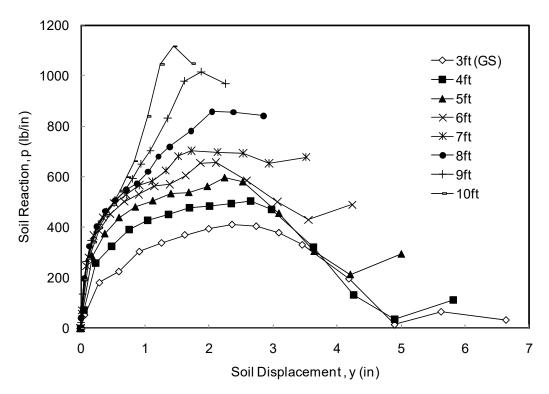
Figure 7-6. Back-Calculated *p*-*y* Curves for 2D Pile (I-4) (2D from crest)
