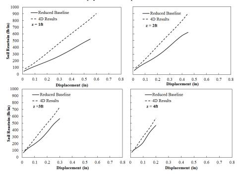
Figure 13-12 Reduced baseline (with Mezazigh and Levacher (1998) reduction coefficients) and 4D p-y curve comparison
