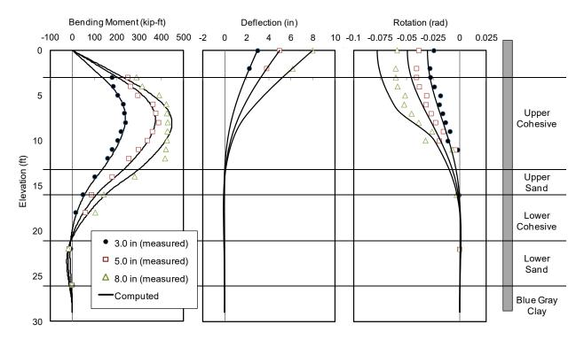
**Figure 7-13.** Comparison of Test Results and Analysis Using Back-Calculated *p-y* Curves for 4D Pile (I-5) for Pile Head Displacement of 3.0, 5.0 and 8.0 in.
