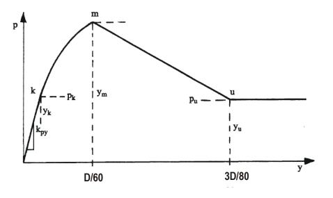
**Figure 2-18** Characteristic Shape of *p*-y Curve for  $c-\phi$  Soil (Reese and Van Impe 2001)
