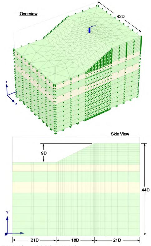
Figure 9-4 Finite Element Mesh for the 0D Pile
