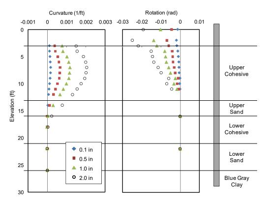
Figure 6-3. Test Results of 8D pile (I-6) for Pile Head Displacement of 0.1, 0.5, 1.0 and 2.0 in
