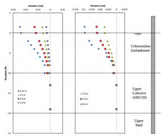
Figure 11-10 Rotation Results for the 2D Pile (P-6) at varying Displacements
