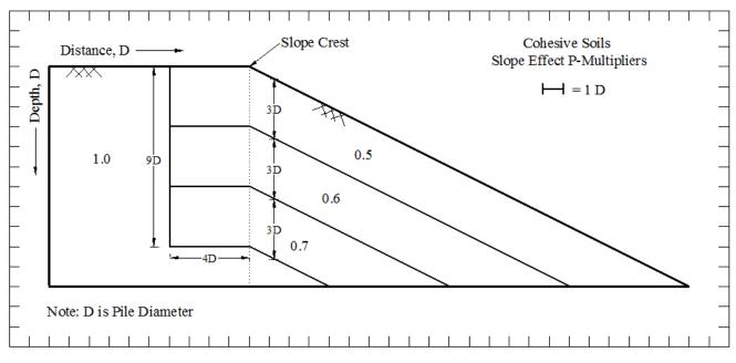
Figure 14-1 Recommended p-Multipliers for a Generalized Cohesive Slope
