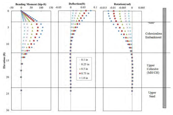
**Figure 12-7** Comparison of Test Results and Analysis Using Back-Calculated *p*-*y* Curves for the 4D Pile (P-7) for Pile Head Displacement of 0.1, 0.25, 0.5 and 1.0 in.
