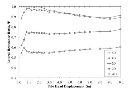
Figure 13-13 Lateral resistance ratios as a function of displacement
