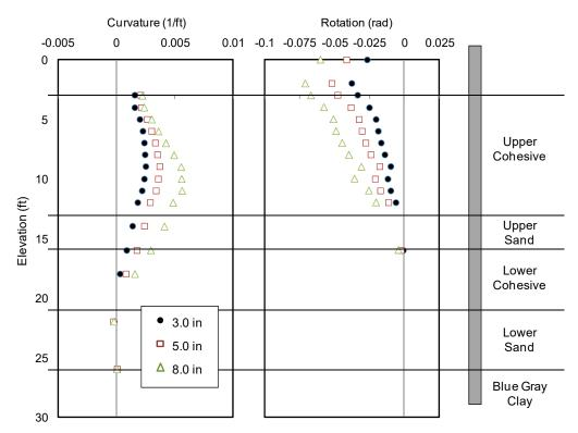
Figure 6-7. Test Results of 2D pile (I-4) for Pile Head Displacement of 3.0, 5.0 and 8.0 in
