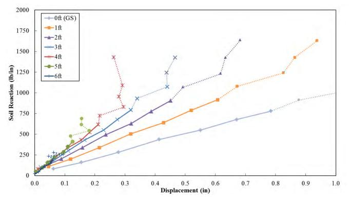
**Figure 12-6** Back-Calculated *p-y* Curves for the 4D Pile (P-7) Showing Lower Displacements Note: Dotted Lines Present Data after Initial Pile Yielding
