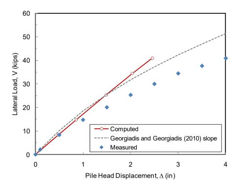
Figure 9-9 Comparison of Load-Displacement Curve from Test Results and FEM Analysis for the 0D Pile
