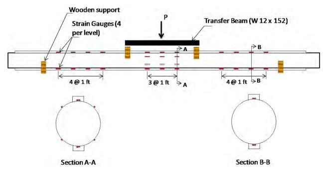
Figure 4-3. Test Set-Up for Calibration Pile
