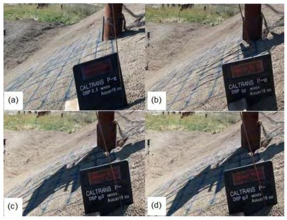
**Figure 10-6** Observations during lateral loading testing of pile P-10 (-4D) a) Pile eat 0.5" of displacement b) Pile at 5.0" of displacement c) Pile at 10.0" of displacement with passive wedge cracking d) Passive wedge movement on slope
