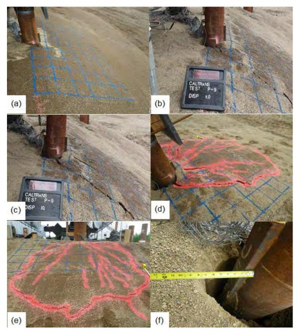
Figure 10-5 Observations during lateral loading testing of pile P-9 (0D) a) Pile before loading b) Pile at 5.0" of displacement with cracks forming c) Pile at 10.0" of displacement with passive wedge cracking d) Passive wedge movement on slope at end of testing e) Passive wedge movement at end of testing f) Gap formation behind pile
