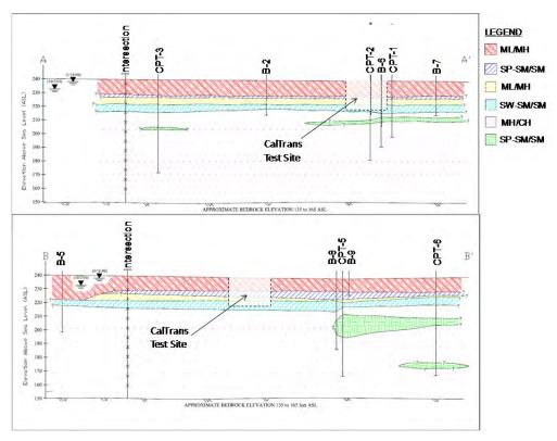
**Figure A-2**. Location of Caltrans Section Projected onto Cross Section A-A' and B-B' (modified from Dickenson, 2006)
