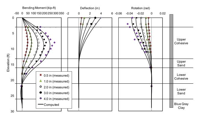
Figure 7-29. Comparison of Test Results and Analysis Using Recommendation for 0D Pile (I-7)
