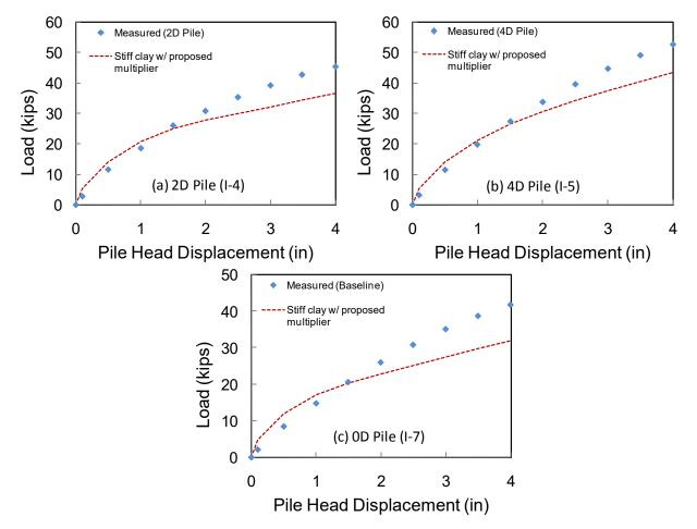
**Figure 8-3.** Computed Load Displacement Curves using Stiff Clay *p-y* Curve (Reese and Welch, 1975) and Proposed Recommendation Compared to Measured Response (a) 2D Pile (I-4), (b) 4D Pile (I-5) and 0D Pile (I-7)
