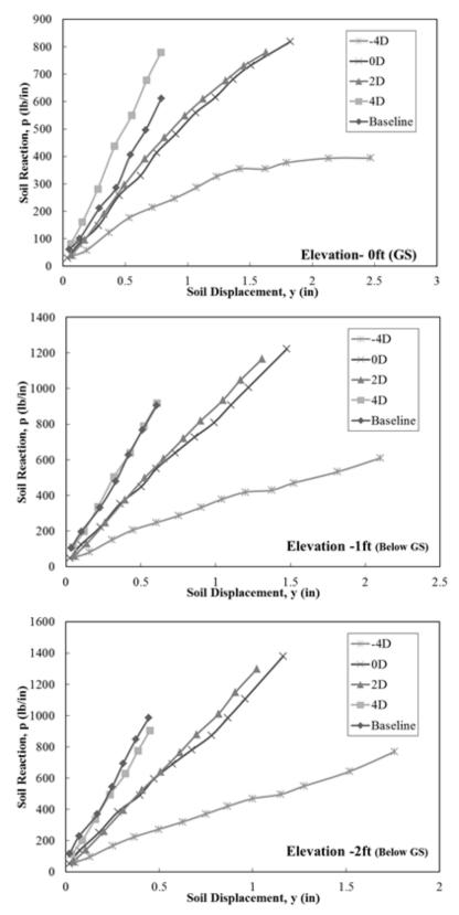
Figure 12-21 Comparison of *p*-*y* Curves for Each Pile at the Same Depth (GS to -2ft)
