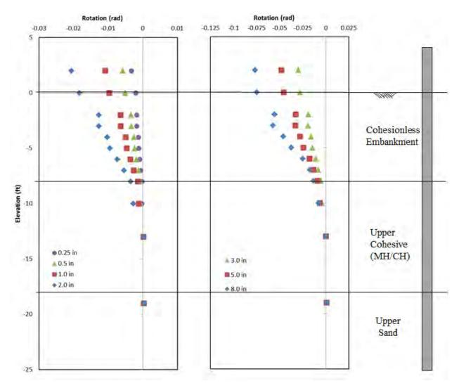
Figure 11-16 Rotation Results for the -4D Pile (P-10) at varying Displacements
