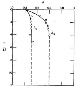
**Figure 2-10** Value of Constant A for *p*-*y* Curves for Stiff Clay Below Water Table (after Reese *et al.* 1975)
