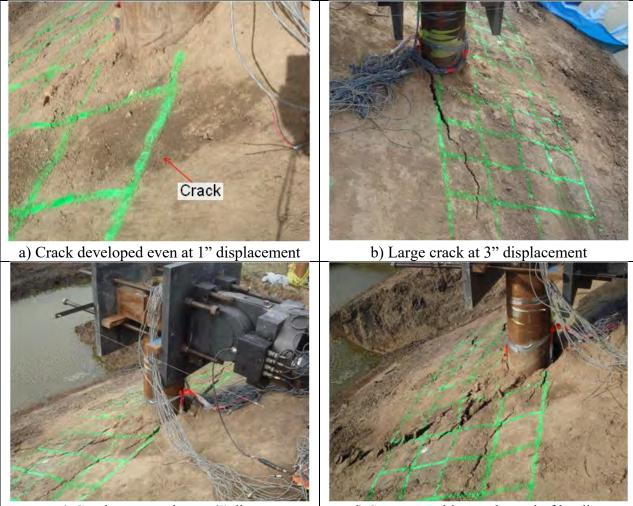
c) Crack propagation at 4" disp.d) Severe cracking at the end of loadingFigure 5-6. Observations from Lateral Load Test for -4D Pile (I-8)
