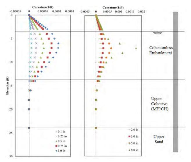
Figure 11-12 Curvature Results for the 0D Pile (P-9) at varying Displacements
