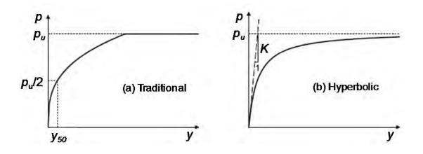
Figure 2-7 Typical Shapes of *p*-*y* Curves (after Georgiadis and Georgiadis 2010)
