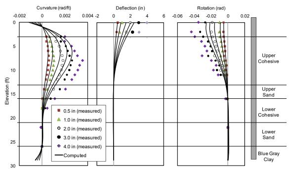
Figure 9-10 Comparison of Test Results and FEM Analysis for the 0D Pile
