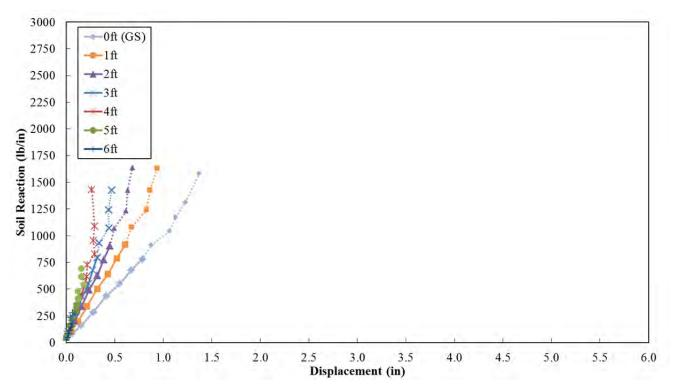
**Figure 12-5** Back-Calculated *p-y* Curves for the 4D Pile (P-7) Note: Dotted Lines Present Data after Initial Pile Yielding
