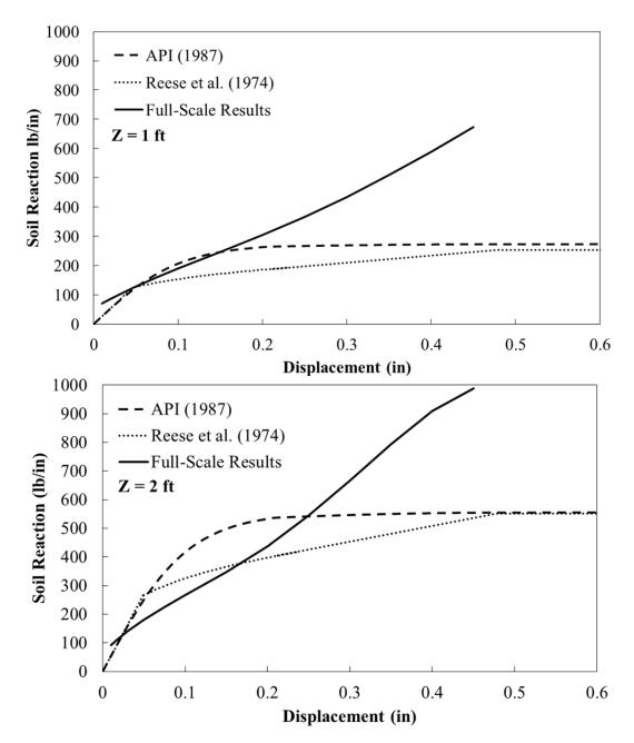
Figure 13-7 Comparison of the API (1987), Reese et al. (1974) predicted baseline p-y curves with full-scale results at depths of 1 ft (top) and 2 ft (bottom)
