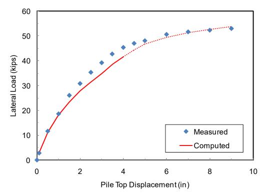
**Figure 7-7.** Comparison of Load-Displacement Curves from Test Results and Analysis Using Back-Calculated *p*-*y* Curves for 2D Pile (I-4)
