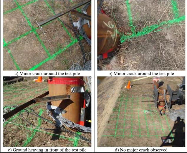
c) Ground heaving in front of the test piled) No rFigure 5-4. Observations from Lateral Load Test for 8D Pile (I-6)
