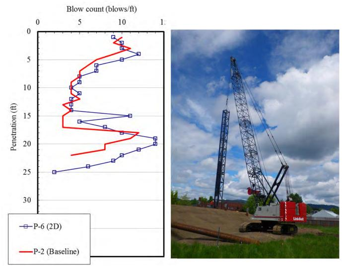
Figure 4-16. Pile Driving Logs for Baseline Piles for Series-II
