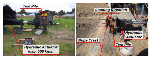
**Figure 4-6.** Actual test setup – Baseline Pile Test (left) and Pile Located at 2D from the Slope Crest (right)
