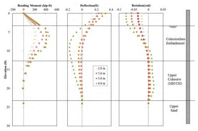
**Figure 12-4** Comparison of Test Results and Analysis Using Back-Calculated p-y Curves for the  $2^{nd}$  Baseline Pile (P-2) for Pile Head Displacement of 2.0, 3.0, 5.0 and 8.0 in.
