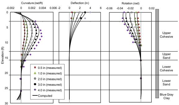
Figure 9-14 Comparison of Test Results and FEM Analysis for the 4D Pile
