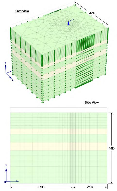
Figure 9-3 Finite Element Mesh for the Baseline Pile
