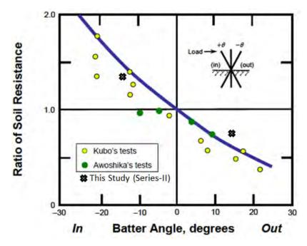
**Figure 11-20** Model used for LPILE Battered Pile Predictions with the +14° and -14° Battered Pile Results from this Study (Series-II) (after Reese et al., 2004)
