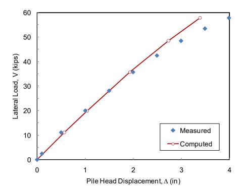
Figure 9-7 Comparison of Load-Displacement Curve from Test Results and FEM Analysis for the Baseline Pile
