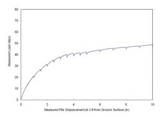
Figure 6-15. Load-Displacement Curve for -4D Pile (I-8)
