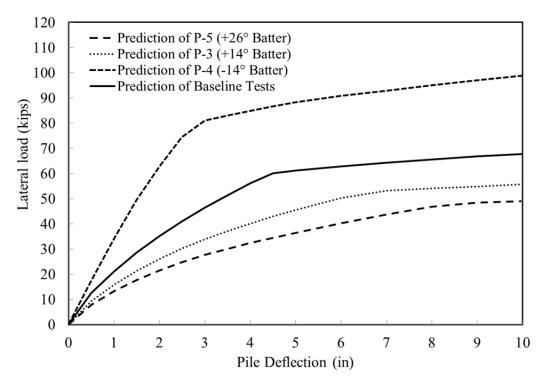
**Figure 11-19** Predicted Load-Displacement Curves for the Battered Pile and Baseline Piles from LPILE
