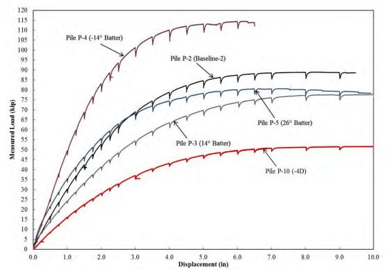
**Figure11-18** Comparison of Load-Displacement Curves between the Baseline Pile (P-2), Pile P-10 (-4D) and Battered Piles
