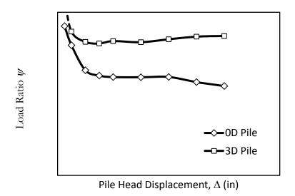
Figure 2-24 Load Ratio for Piles Near Sand Slope (after Mirzoyan 2004)
