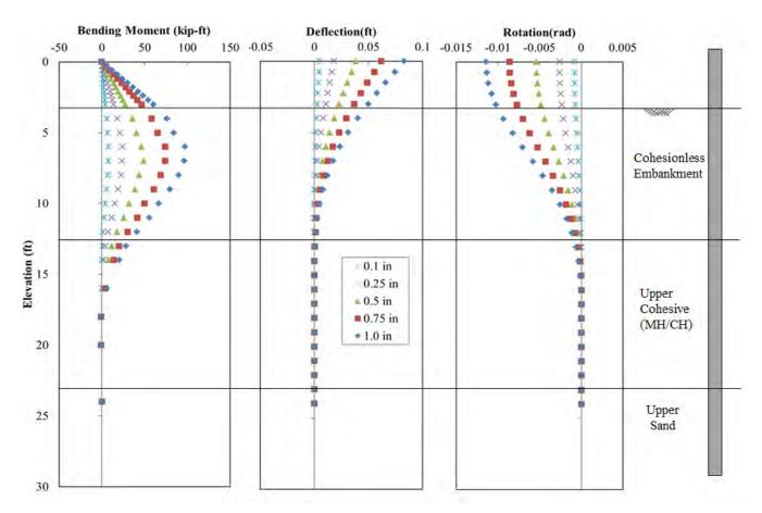
**Figure 12-15** Comparison of Test Results and Analysis Using Back-Calculated *p-y* Curves for the 0 (P-9) for Pile Head Displacement of 0.1, 0.25, 0.5 and 1.0 in.
