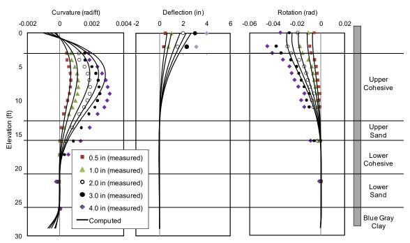
Figure 9-12 Comparison of Test Results and FEM Analysis for the 2D Pile
