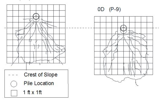
Figure 10-12 Cracking Patterns for the 2D and 0D Test Piles
