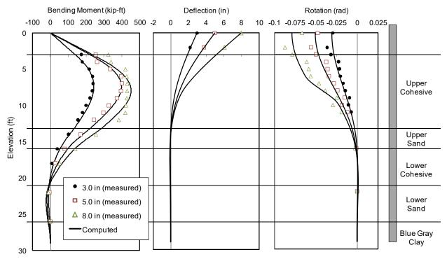
**Figure 7-5.** Comparison of Test Results and Analysis Using Back-Calculated *p*-*y* Curves for 8D Pile (I-6) for Pile Head Displacement of 3.0, 5.0 and 8.0 in.
