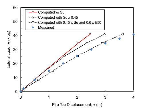
Figure 9-15 Comparison of Load-Displacement Curves from Sensitivity Analysis and the Measured Results for the 0D Pile
