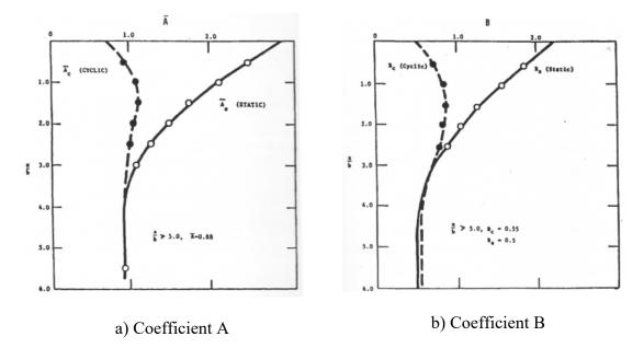
**Figure 2-15** Values of Coefficients Used for Developing *p-y* Curves for Sand a) Coefficient A; b) Coefficient B (after Reese *et al.* 1974)
