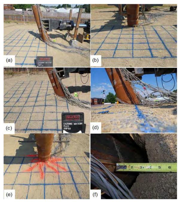
**Figure 10-7** Observations during Lateral Loading Testing of Pile P-4 (-14 Batter) a) Pile before loading b) Front of pile before loading c) Pile at 10.0" of displacement d) Soil heave at end of testing e) Soil cracking at end of testing f) Gap formation behind pile
