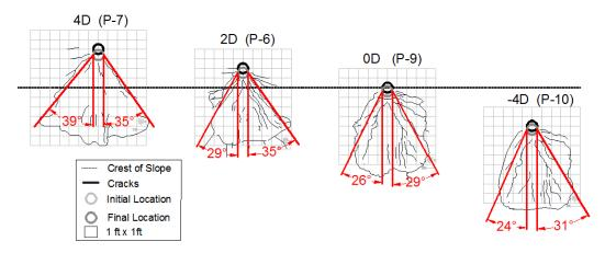
Figure 10-10 The Shear Failure Angle,  $\Omega$ , for the Near Slope Tests
