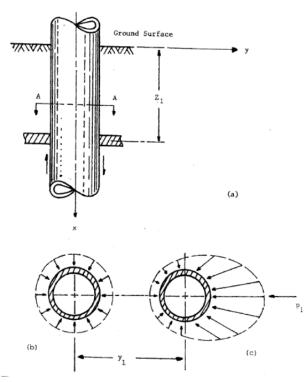
**Figure 2-2** Distribution of Soil Pressure against the Pile before and after Lateral Loading: a) Elevation View of Pile; b) Soil Pressure at Rest; c) Soil Pressure after Lateral Loading (after Reese *et al.* 2006)
