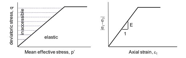
**Figure 9-1** Deviatoric Stress-Mean Effective Stress Relationship and Stress-Strain Relationship in Elastic-Perfectly Plastic Model (after Brinkgreve and Swolfs 2007)
