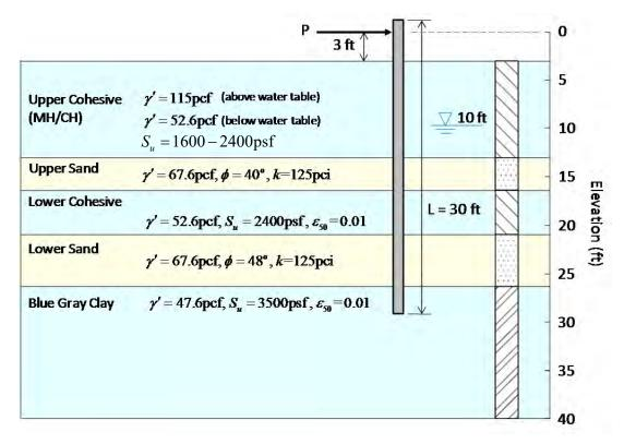
Figure 7-1. Idealized Soil Profile for Lateral Load Analyses
