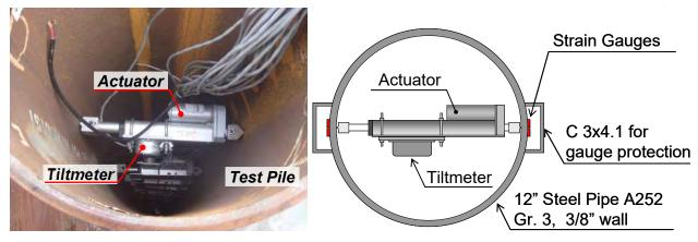
Figure 4-13. Cross-section view of test pile showing tiltmeter arrangement
