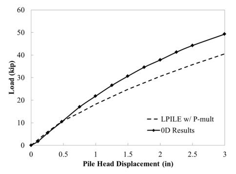
Figure 13-4 Comparison of the 0D full-scale results with the LPILE prediction using the proposed p-multipliers for a pile on a slope crest
