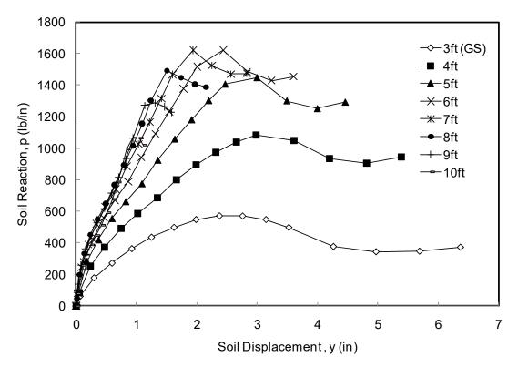
Figure 7-10. Back-Calculated *p*-*y* Curves for 4D Pile (I-5)
