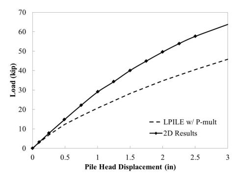
Figure 13-3 Comparison of the 2D full-scale results with the LPILE prediction using the proposed p-multipliers for a pile 2D from a slope crest
