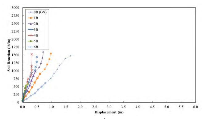
**Figure 12-1** Back-Calculated *p-y* Curves for the 2<sup>nd</sup> Baseline Pile (P-2) Note: Dotted Lines Present Data after Initial Pile Yielding
