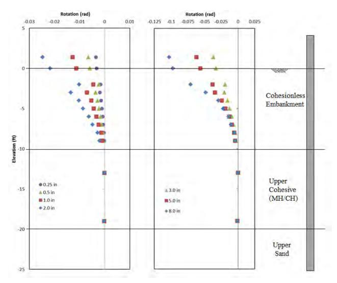
Figure 11-4 Rotation Results for Baseline Pile (P-2) at varying Displacements
