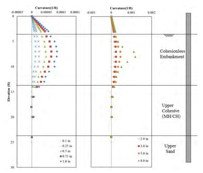
Figure 11-15 Curvature Results for the -4D Pile (P-10) at varying Displacements
