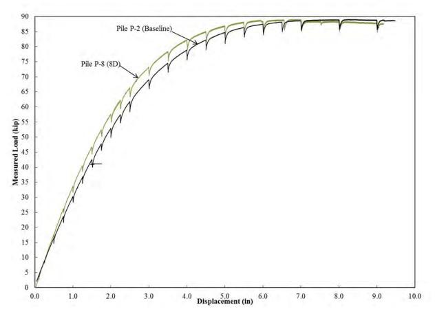
**Figure 11-1** Comparison of Load-Displacement Curves between the Baseline Pile (P-2) and the 8D Pile (P-6)
