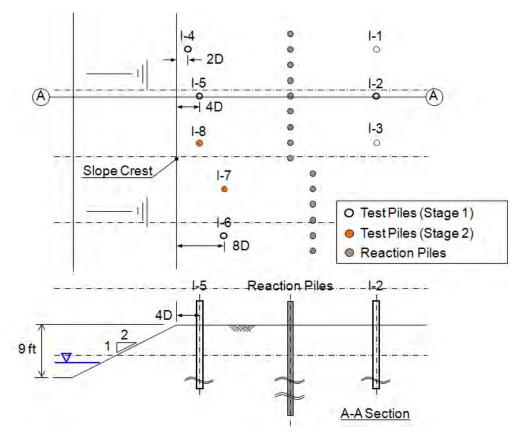
Figure 4-5. Plan View for Test Stage I with location of Test Piles, Reaction Piles and Slope 1
