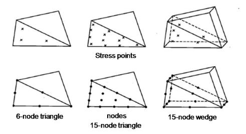
**Figure 9-2** Distribution of Nodes and Stress Points in a 15-Node Wedge Element (after Brinkgreve and Swolfs 2007)
