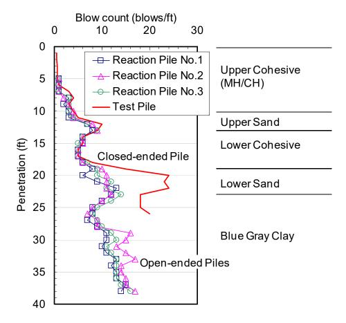
Figure 4-12. Pile Driving Logs for Baseline Pile (I-1) and Reaction Piles for Series-I
