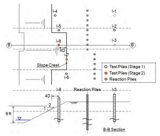
Figure 4-9. Plan View for Test Stage I with Location of Slope 2
