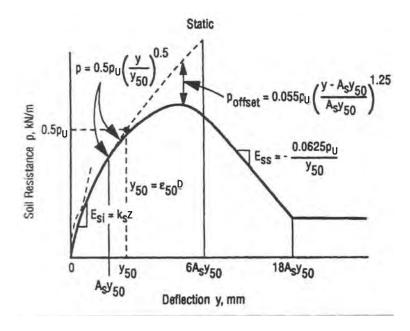
**Figure 2-9** Characteristic Shape of *p*-*y* Curve for Stiff Clay below Water Table for Static Loading (after Reese *et al.* 1975)
