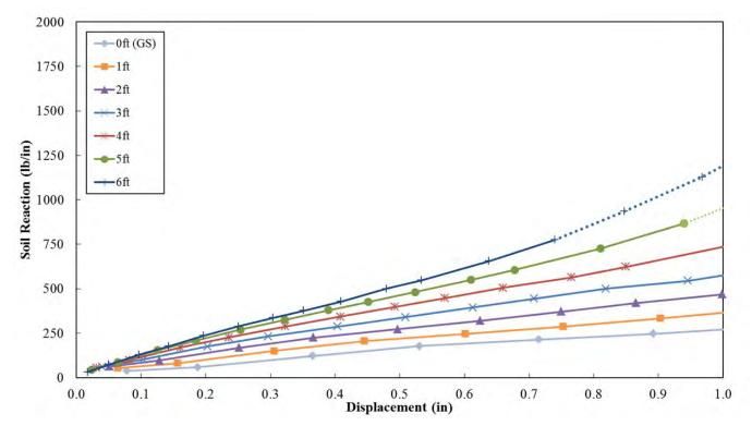
**Figure 12-18** Back-Calculated *p*-*y* Curves for the -4D Pile (P-10) With Lower Displacements Note: Dotted Lines Present Data after Initial Pile Yielding
