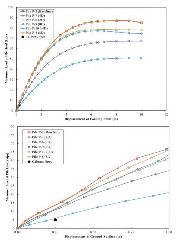
Figure 11-17 Top: Load Displacement Curve at Ground Surface with Caltrans Spec Bottom: Load-Disp with Caltrans Spec up to 1 in. of Displacement
