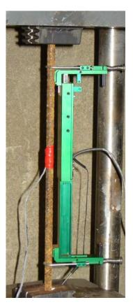
Figure 5.2.2. Typical Steel Tension Test
