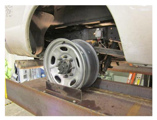
Figure 3.3.5. Restraint System for Truck without Tires
