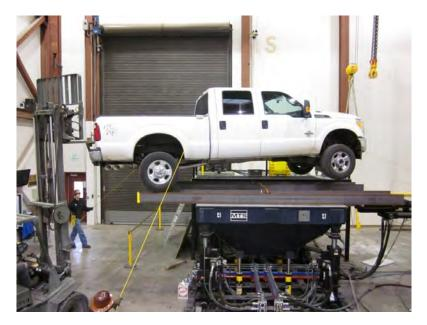
Figure 3.3.3. Truck Placement on Shake Table
