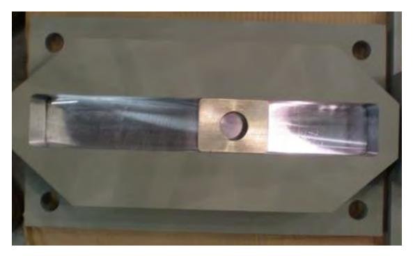
Figure 4.4.3. Bottom Half of the Shear Key Assembly Showing Pin in Bushing Located in Longitudinal Slot
