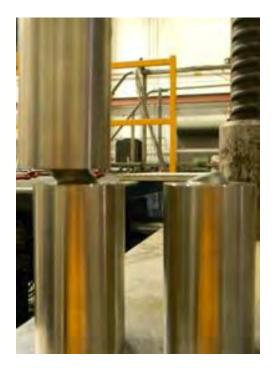
Figure 4.4.5. Left: Plastic Shear Distortion in Shear Pin Right: Lower Half of Failed Shear Pin
