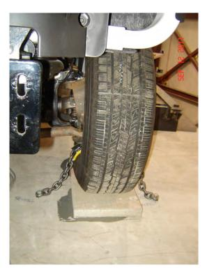
Figure 4.6.7. Wheel Restraint
