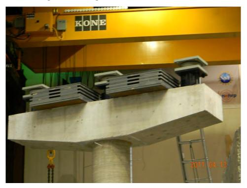
Figure 4.5.10. Added Weight, Load Cells, and Bearings on a Bent Cap
