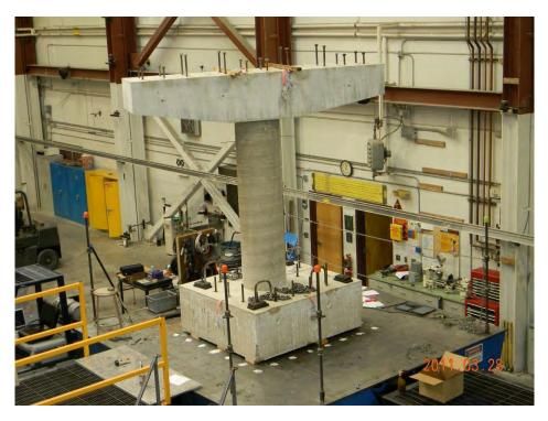
Figure 4.5.9. Single-Column Bent on Shake Table
