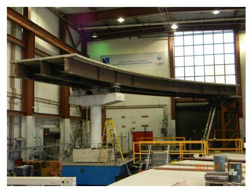
Figure 4.5.13. North Segment of Superstructure in Place
