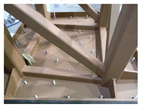
Figure 4.5.8. Anchorage of Abutment Tower on North Shake Table
