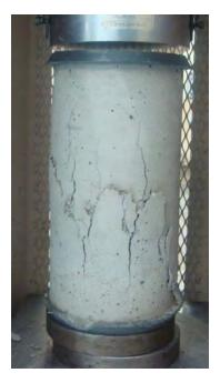
Figure 5.2.1. Typical Concrete Compression Test
