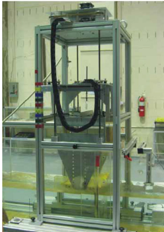
Figure 7. Experimental setup to measure the hydrodynamic loads on inundated bridge decks (Kerenyi et al. 2009).
