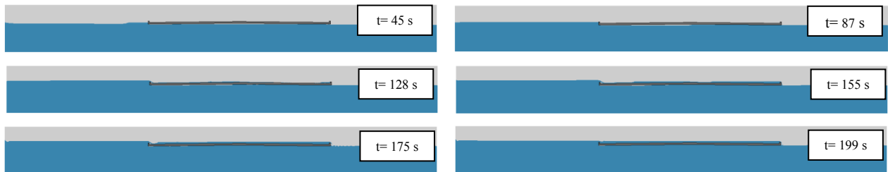
Figure 26. Screen captures of Agua Hedionda Lagoon Bridge, Water surface elevation 5 ft above bridge elevation, Initial impact time period.
