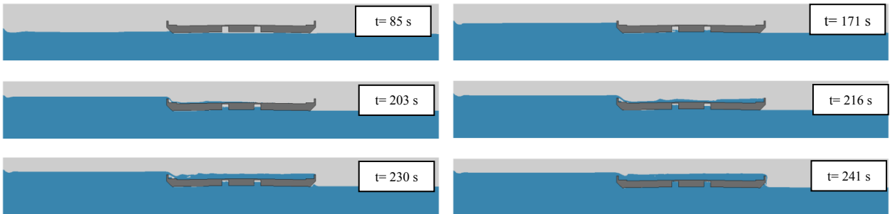
Figure D-17. Screen captures of Malibu Lagoon Bridge, Water surface elevation 10 ft above bridge elevation, Initial impact time period.
