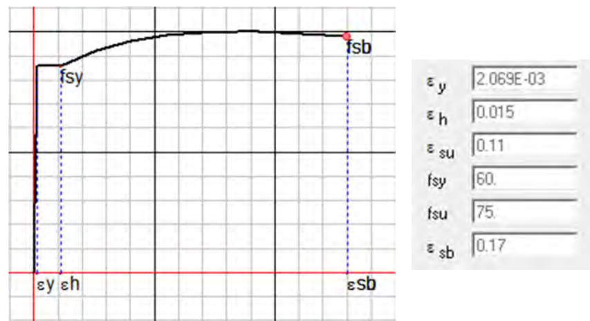
Figure C-4 Steel stress-strain curve considering the strain hardening
