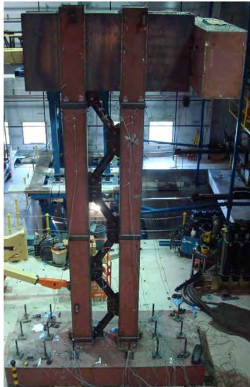
Figure A-9 Twin Column Specimen S2-1 with BRBs Prior to Testing (El-Bahey and Bruneau, 2010)
