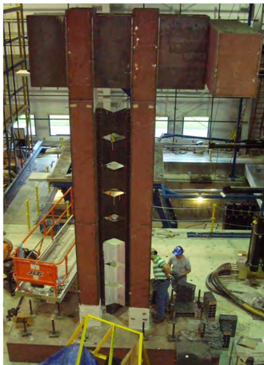
Figure A-58 Specimen Setup With SPSLs (El-Bahey and Bruneau, 2010)
