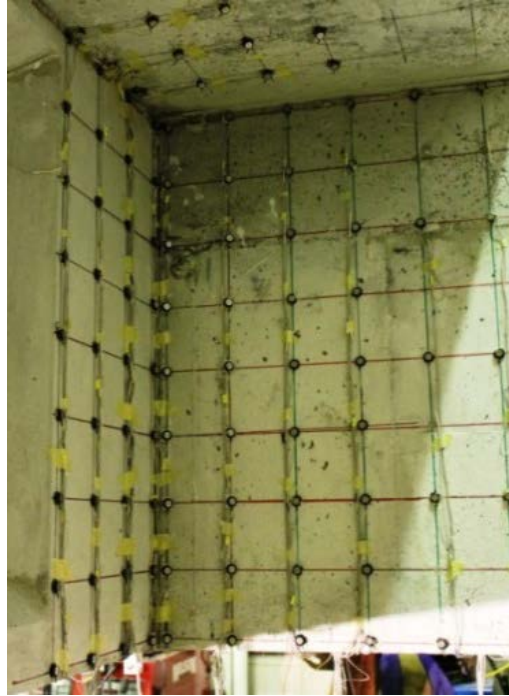
Figure 3.16: LED indicators to record position during experimental testing
