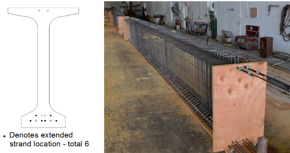
Figure 4.13: Girder strand layout and rebar cage
