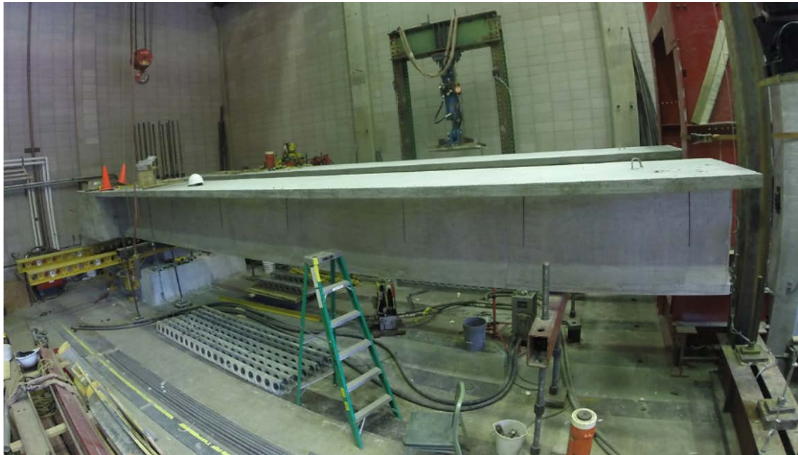
Figure 5.9: Third test unit with the ESMS and ESLS connections
