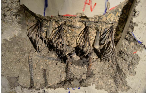
Figure 4.51: Mushrooming of extended strands in ESSP connection
