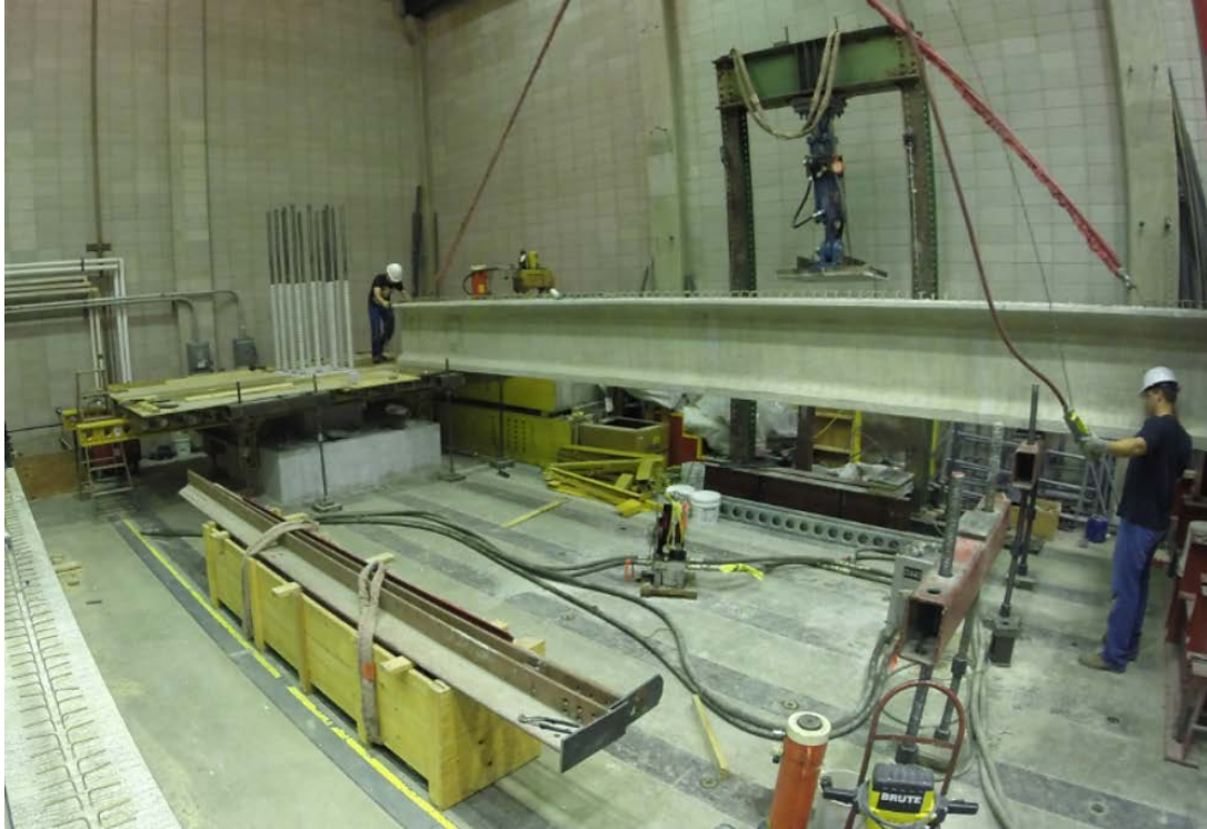
Figure 5.5: Place the girder on temporary falsework
