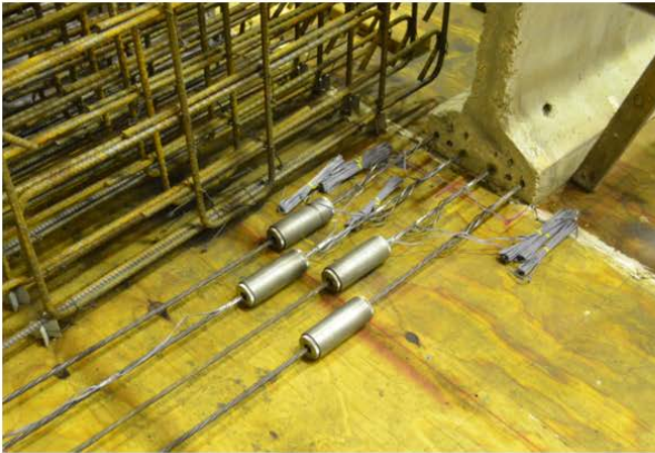
(a) Spliced strands in ESMS detail
