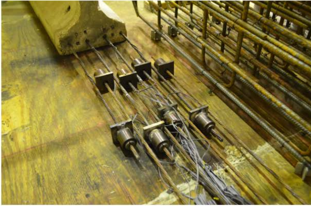
(b) Anchored strand lap splices in ESLS detail
