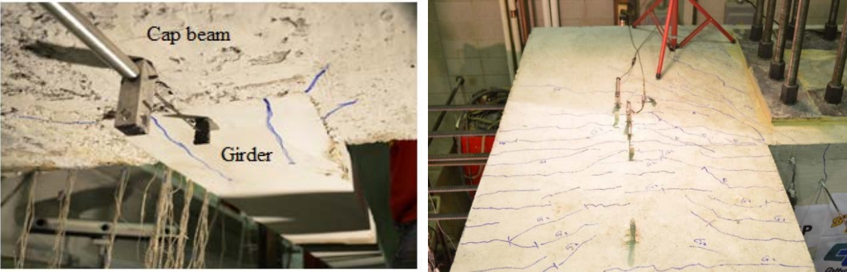
Figure 4.25: DCDT's on underside (left) and top of girder (right)
