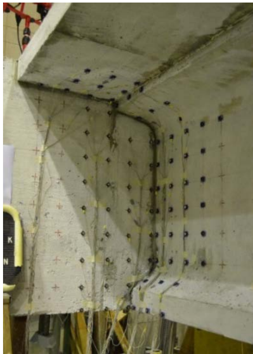
Figure 4.28: LED configuration at connection region
