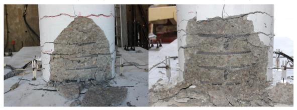
(c) north face at Cycle 10b ( $\mu = 6$ ) (d) south face at Cycle 11b ( $\mu = 7$ ) Figure 4.16 – Evolution of damage at the base of the column of Specimen #3
