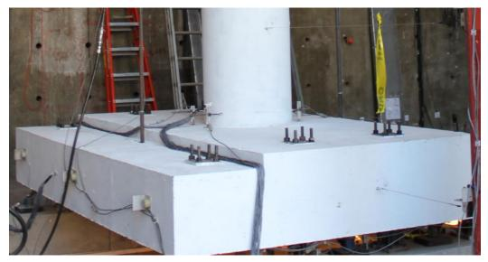
Figure 3.4 – Slab with drop cap in Specimen #3
