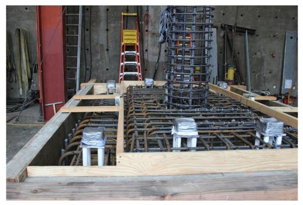
Figure 3.15 – Picture of slab and column reinforcement of Specimen #3 prior to casting
