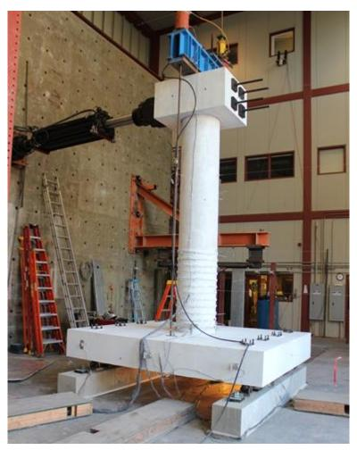
Figure 3.3 – Picture of test setup (Specimen #1)
