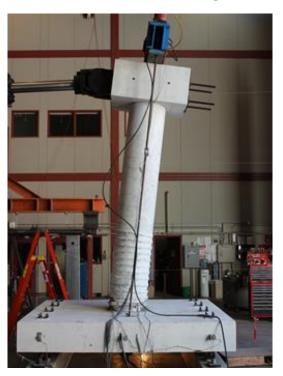
Figure 4.2 – Deflected shape of Specimen #1 at ductility 6
