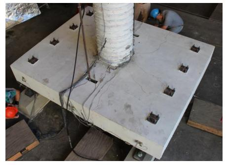
Figure 4.8 – Damage at the bottom face of the slab (top face in the specimen) of Specimen #1 at the end of testing
