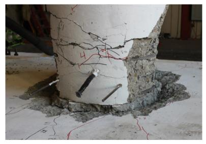
Figure 4.18 – Damage at the slab-column interface after the testing of Specimen #3
