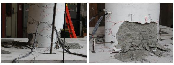
(c) east face at Cycle 10a ( $\mu = 6$ ) (d) north face at Cycle 10a ( $\mu = 6$ ) Figure 4.11 – Evolution of damage at the bottom of the column of Specimen #2
