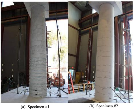
Figure 4.4 – Flexural cracks at the south face of the columns of Specimens #1 and #2 at Cycle 4 ( $1^{st}$  yield)
