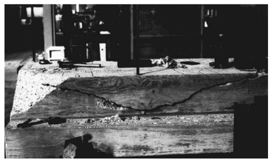
Figure 2.5 – Concrete Breakout failure in a shallow embedment test (De Vries et al. 1999)
