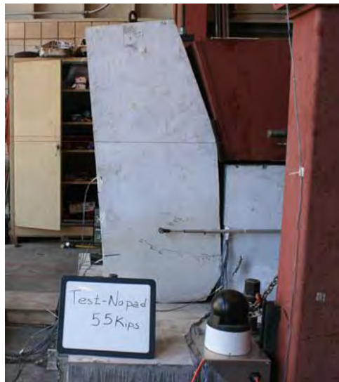
Figure 7.36 Displacement of shear key block at a horizontal load of 55 kips in Test 5
