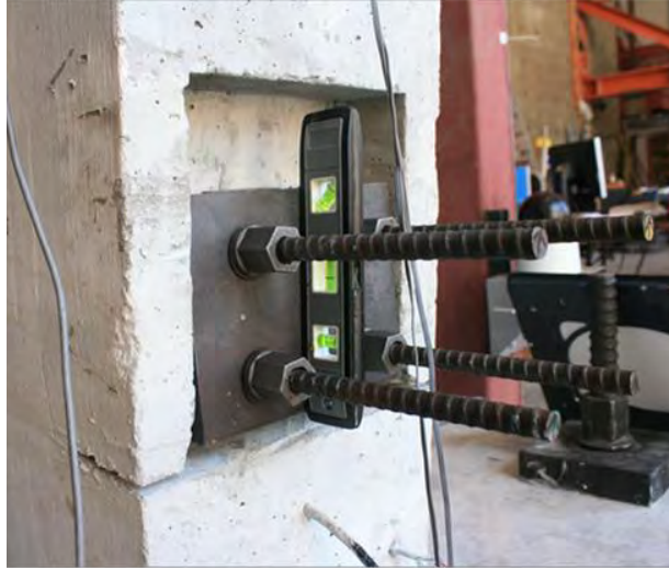
Figure 7.35 Monitoring the rotating plate in Test 5
