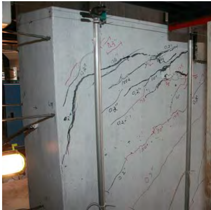
Figure 6.74 Sliding plane from the east face of shear key 9B
