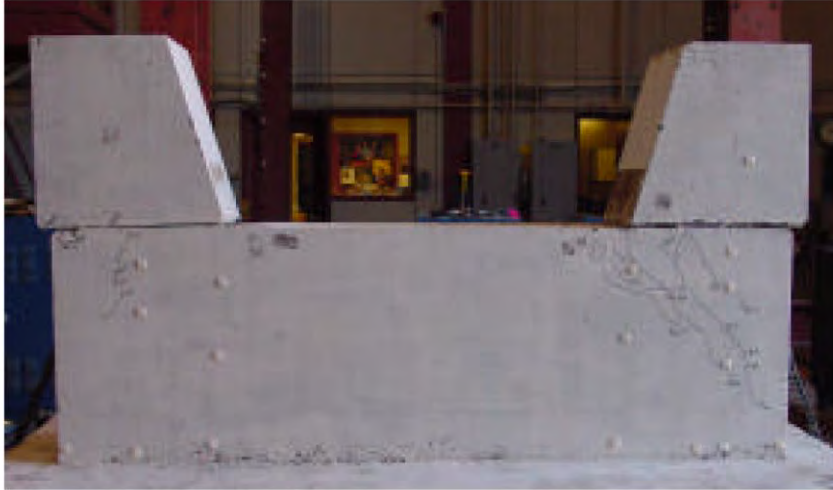
Figure 2.14 Displaced positions of shear key 5A (left) and 5B (right) at the end of the tests (from Borzozzadeh et al. 2006)
