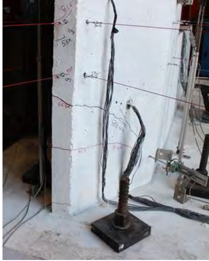
Figure 8.32 Cracks on the southeast side propagating to the northwest side (left) and cracks on the northwest side of shear key 12B at a horizontal load of 88 kips
