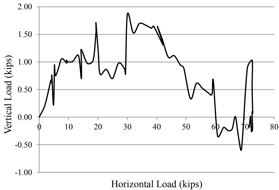
Figure 8.22 Measured vertical force on shear key 12A
