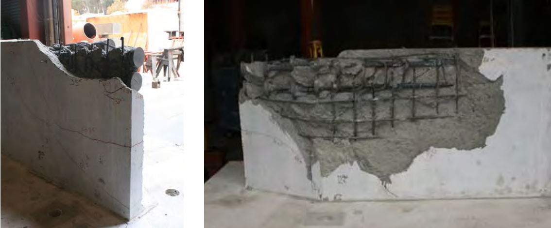
Figure 8.34 Shear plane from the southeast side (left) and from the northwest side (right) after removing shear key 12B
