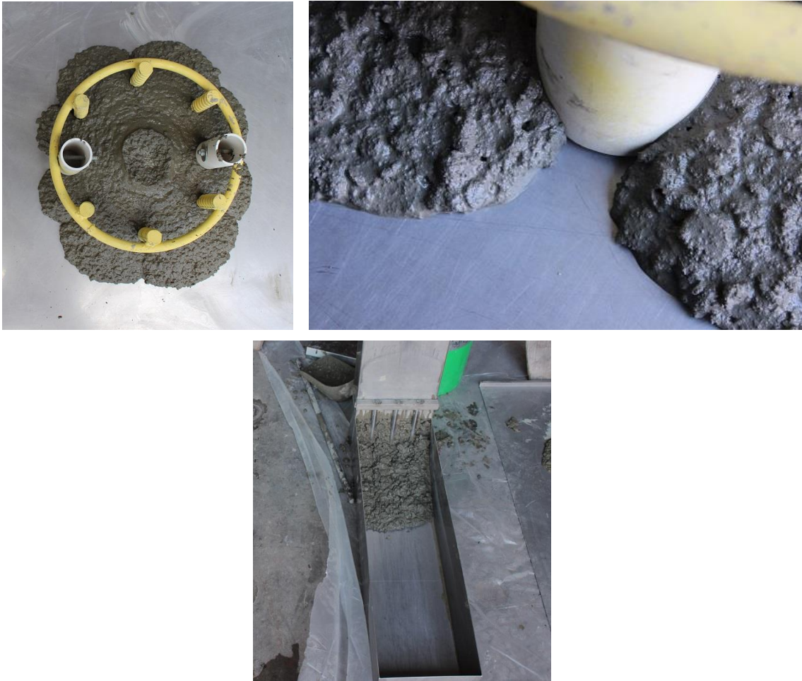
Figure 2.2 – C-Bar and L-Box tests for Mix 4, Trial Batch on 10/23/15
