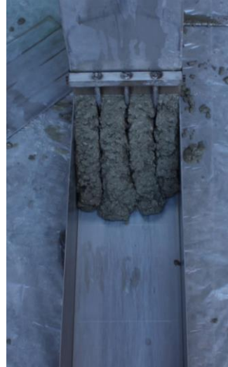
Figure 3.1 – C-Bar and L-Box Tests on Mix 4 for Pile Specimens #1 and #2
