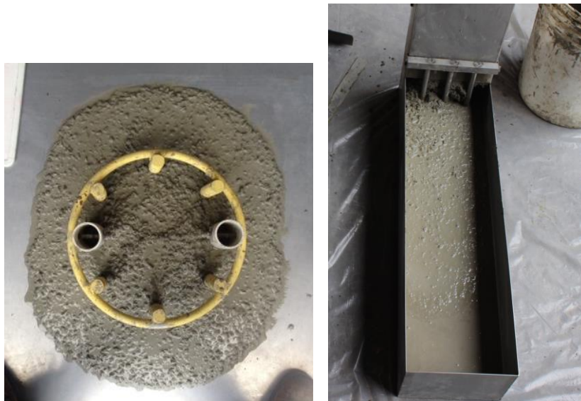
Figure 3.16 – C-Bar and L-Box tests on Mix 2 for Pile Specimens #9 and #10
