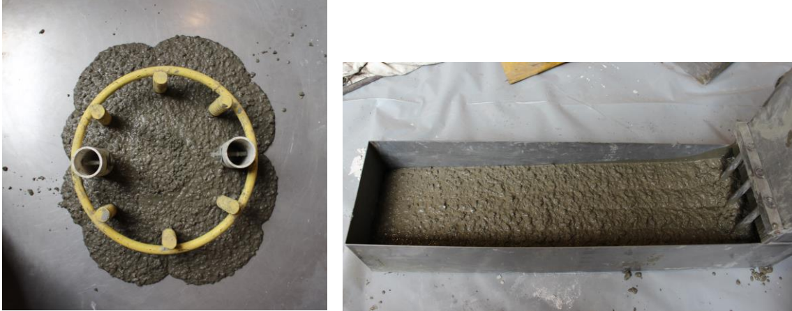
Figure 3.8 – C-Bar and L-Box tests on Mix 2 for Pile Specimens #5 and #6
