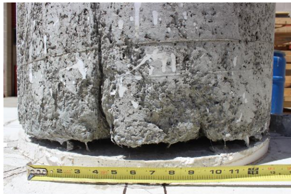
Figure 3.19 – Bottom of Pile Specimen #9 showing gap at base
