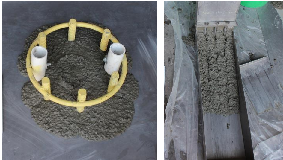
Figure 2.3 – C-Bar and L-Box tests for Mix 5, Trial Batch on 7/17/15
