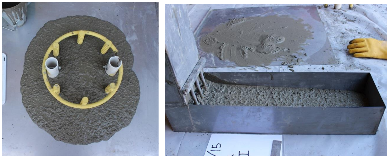
Figure 2.4 – C-Bar and L-Box tests for Mix 2, Trial Batch on 12/17/15
