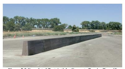
Figure 2-9 Completed Test Article: Concrete Barrier Type 60
