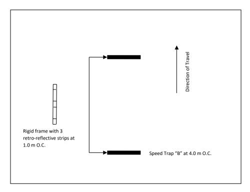
Figure 7-8 Speed Trap Tape Layout
