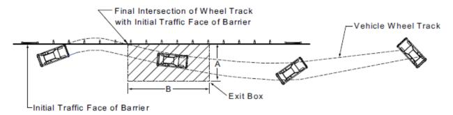
Figure 5-18. Exit Box for Longitudinal Barriers
