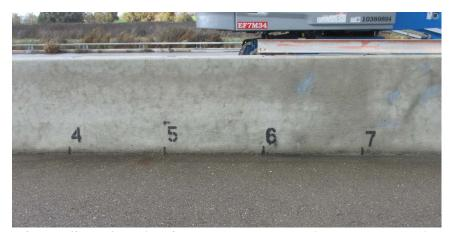
Figure 5-2 Type 60 Barrier Point of Impact (I-beam on barrier was removed prior to test)
