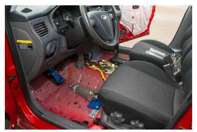
Figure 7-4 Brake Pedal Actuator
