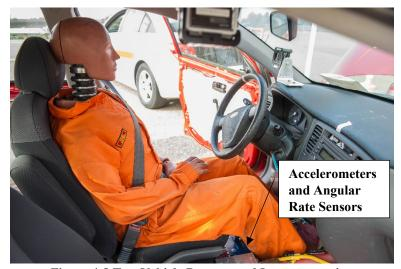
Figure 4-8 Test Vehicle Dummy and Instrumentation
