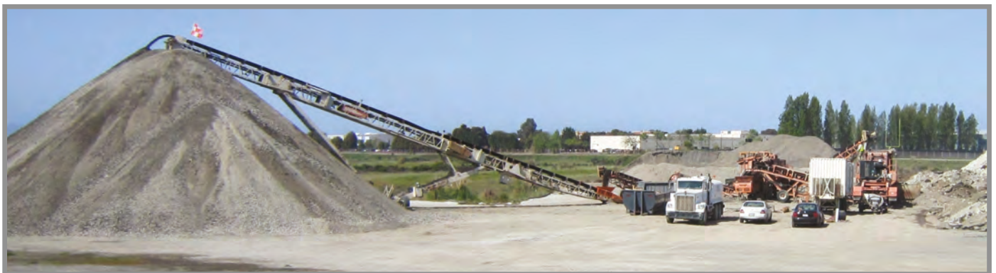
Stockpiles of recycled pavement materials
