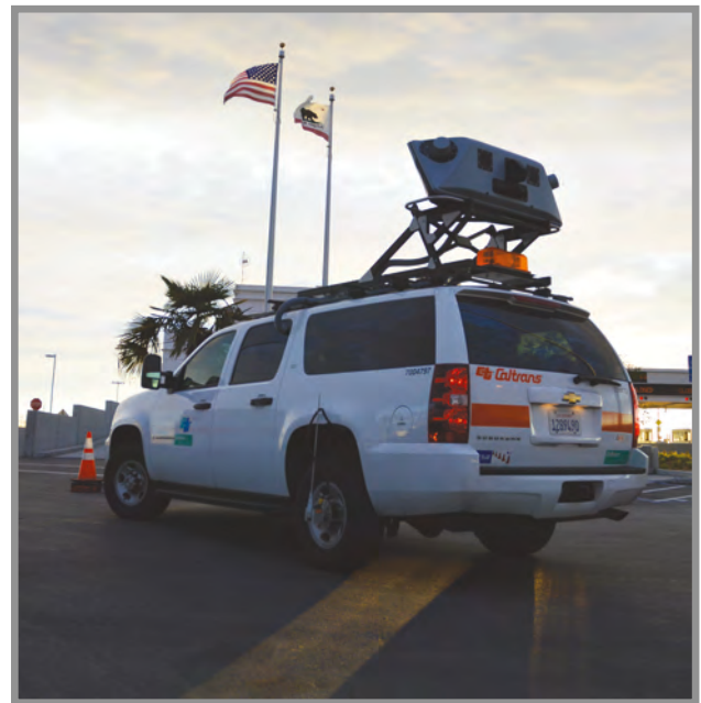
Caltrans Trimble MX8 MTLs vehicle
