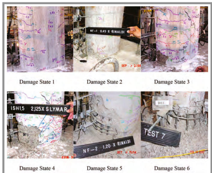
Possible apparent damage states of bridge columns
