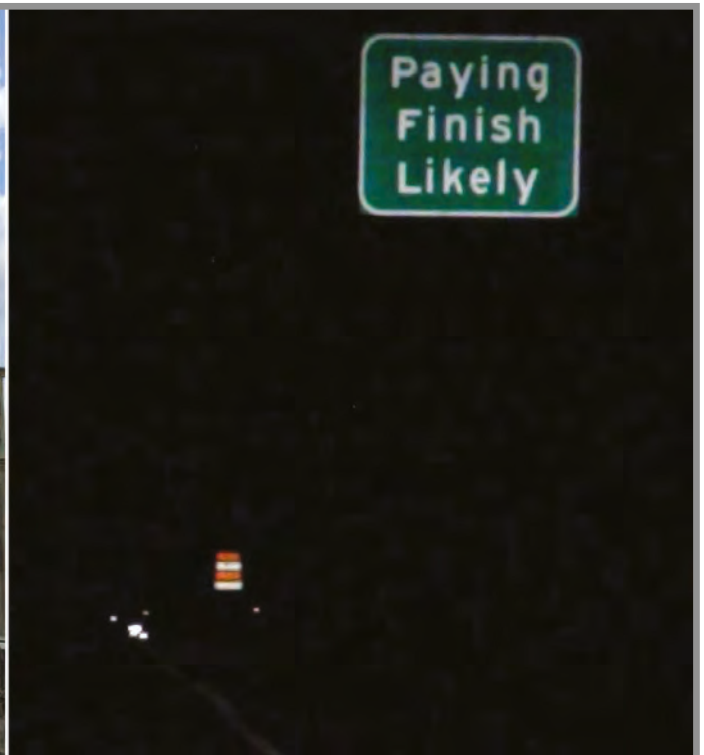
Testing overhead guide signs in the daytime and nighttime using specific letters for spacing and legibility
