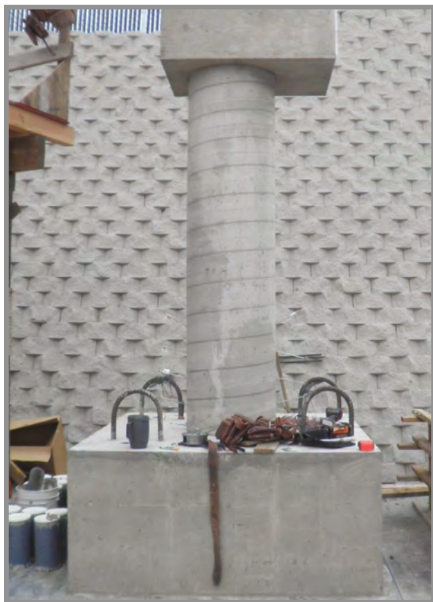
Completed cast-in-place column model
