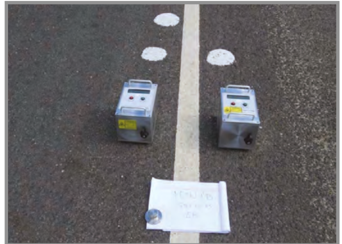
Measuring the pavement macrotexture with a laser texture scanner
