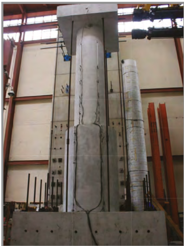
Column-shaft assembly instrumented
