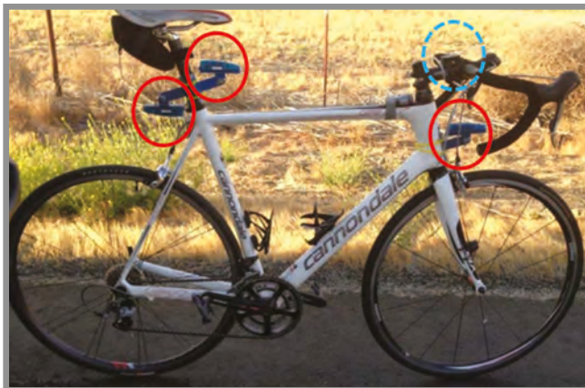
Bicycle instrumented with accelerometers
