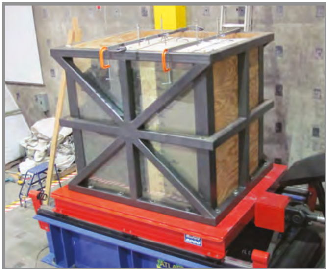
Shake table test of an MSE wall
