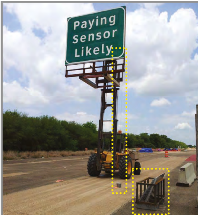
Testing overhead guide signs in the daytime and nighttime using specific letters for spacing and legibility
