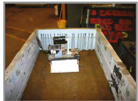
Construction of level ground model: soil mixing and cantilever wall on north end
