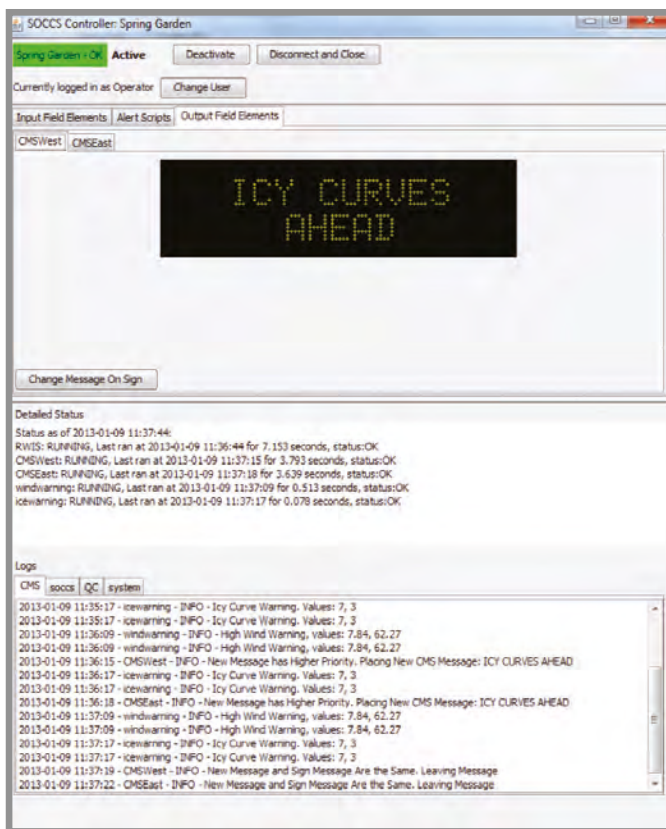
Operator's interface to the ASWSC
