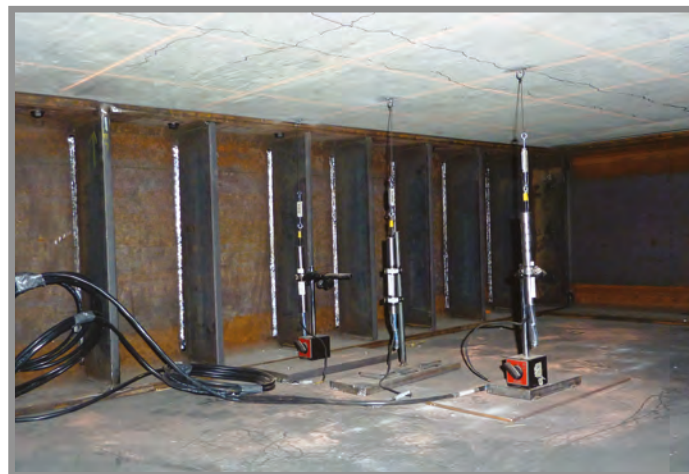
LCPE Instruments recording deflection
