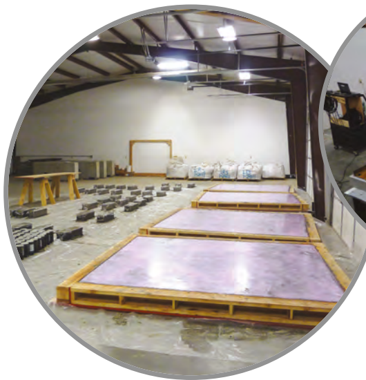
Full-scale decks cast to Caltrans specifications
