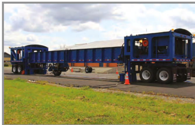
Testing hot mix and warm mix asphalt pavements
