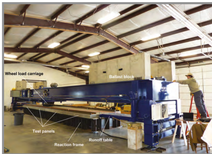
Testing being performed with a 20,000 pound rolling load
