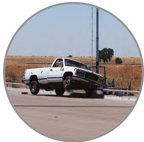
Crash-testing the barrier
