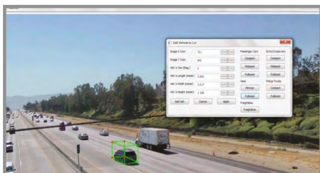
Lane change data extracted from video footage using a software tool developed in this research
