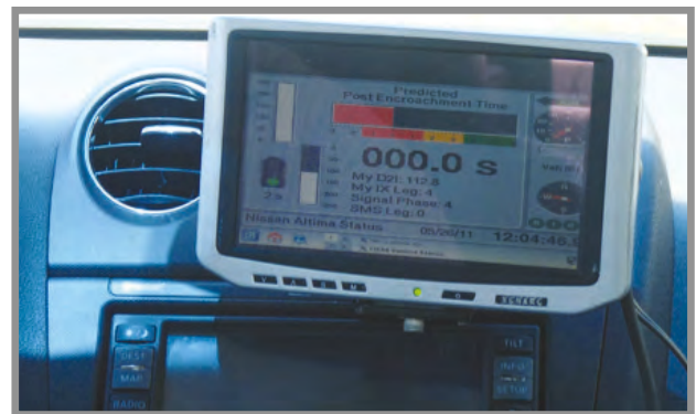
Prototype driver-vehicle interface in an instrumented test vehicle
