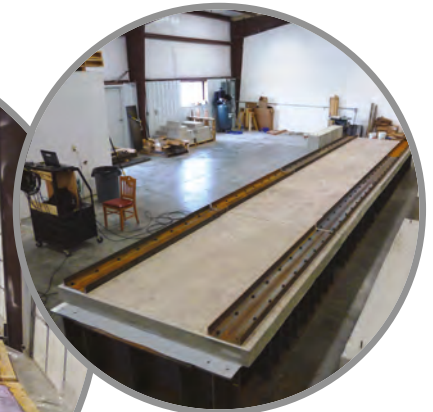
Edge of decks clamped to tester to simulate box girder frame
