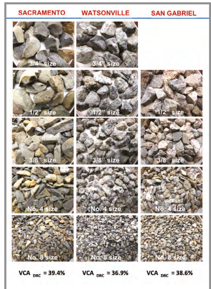
Aggregate samples from northern (left), central (middle), and southern (right) California
