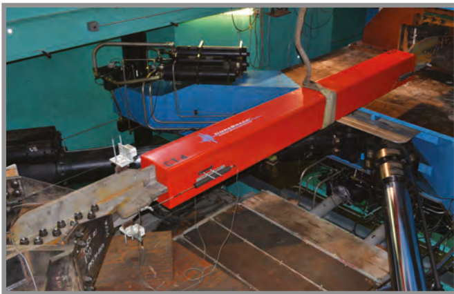
Left and right: Lab testing BRBs
