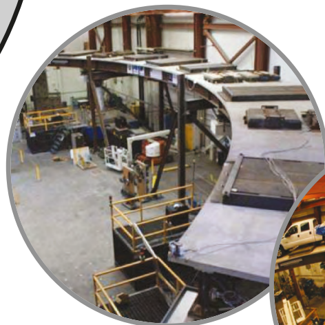
Left: Added weight on deck of instrumented bridge model
