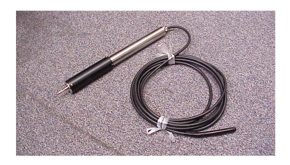
Figure 3.3.22 Displacement Sensor
