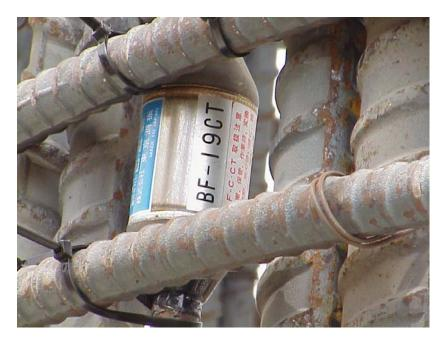
(b) LVDT Type Strain Meter Installed in the Column
