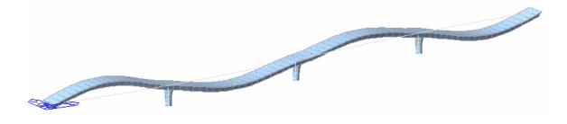
(a) The first mode shape (frequency: 2.085 Hz)
