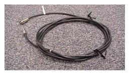
(a)Thermocouple Sensor head
