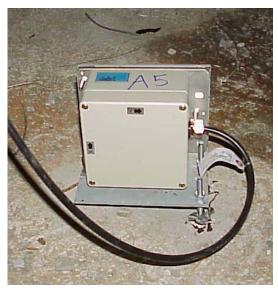
(b) A bi-axial accelerometer mounted in boxgirder with a bracket to adjust the sensor orientations
