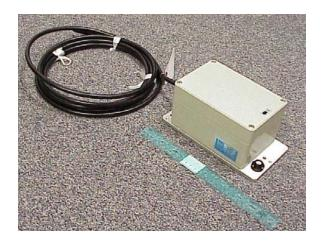
Figure 3.3.7 Picture of a Uni-axial Accelerometer
