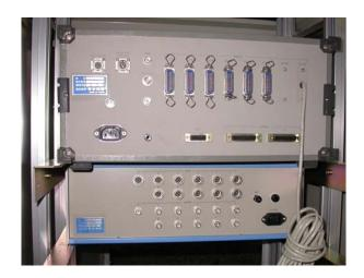
Figure 3.3.12 Data-logger and the Strain Meter Conditioner in the Container
