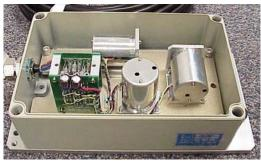
Figure 3.3.9 Pictures of a Tri-axial Accelerometer
