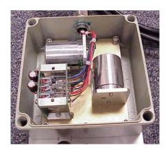
Figure 3.3.8 Pictures of a Bi-axial Accelerometer
