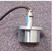
Figure 3.3.20 Soil Pressure Sensor
