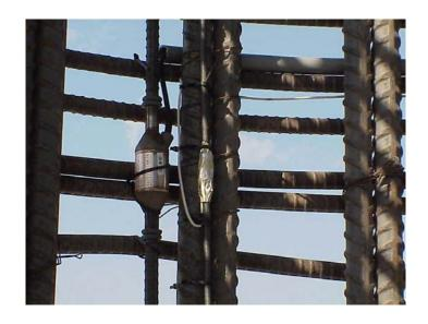
Figure 3.3.17 Conventional Strain Gauge and LVDT Strain Meter Installed in Column 3
