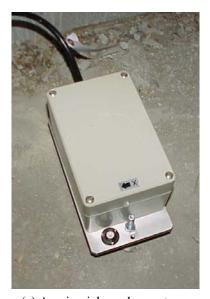
(a) A uni-axial accelerometer mounted in box-girder without bracket
