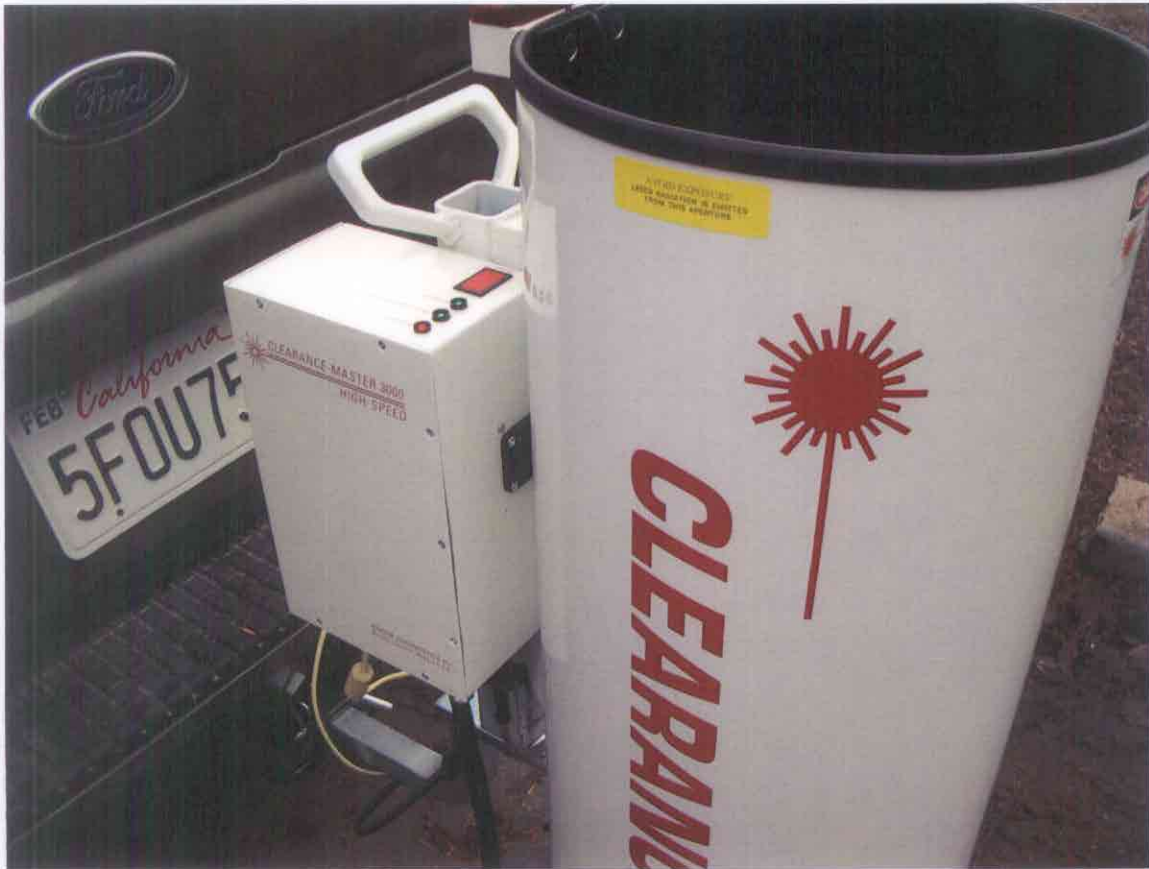
Bridge Measuring Device Ready for use
