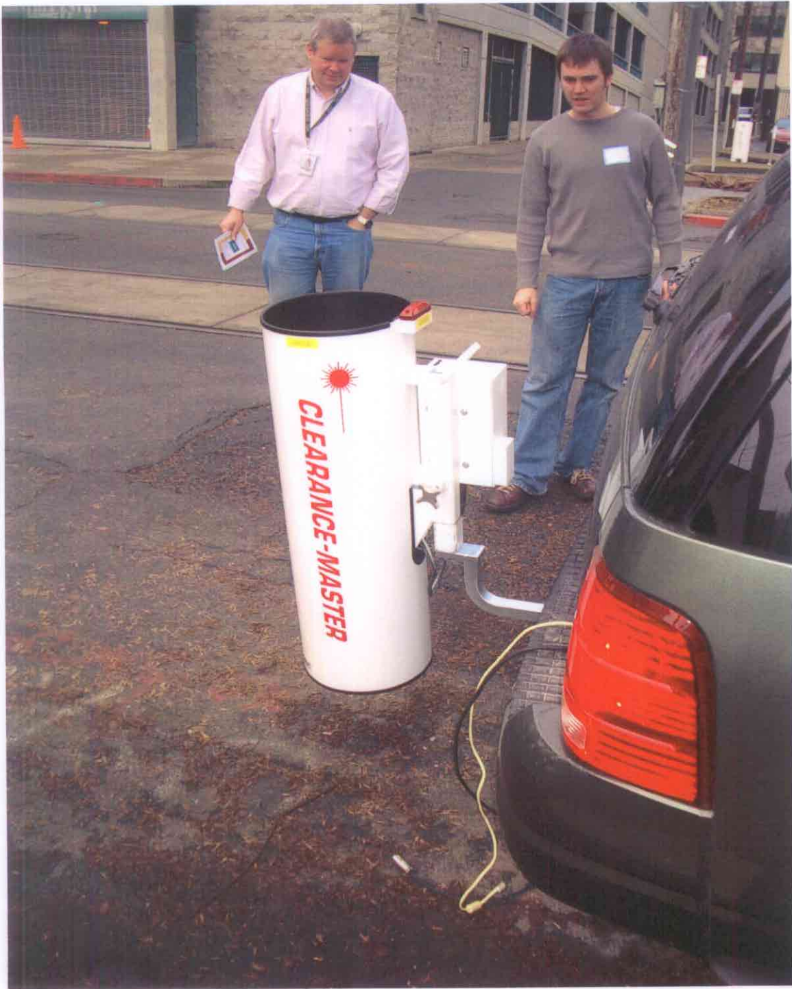
Installed Bridge Measuring Device
