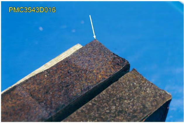
Figure 8: Mating fracture faces at the outer edge of the eye bar. Fracture origin at arrow location.
