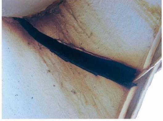
Fig. 4 Cracked eye bar.
