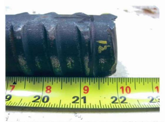
Fig. 3 As received failed support rod from east span. 12 O'clock position, fracture origin.
