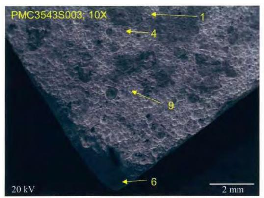
Fig. 45 S.E.M photo of eye bar fracture surface at fracture origin. 10X.
