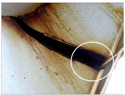
Figure 3: Failure initiation location is circled above and highlighted in following figures.
