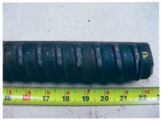
Fig. 4 As received failed support rod from east span. 12 O'clock position, fracture origin.
