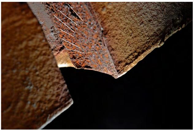
Figure 5: Close up of fracture showing radial ridges pointing to location of crack initiation
