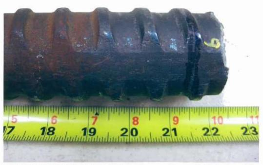
Fig. 9 As received failed support rod from east span. 9 O'clock position.
