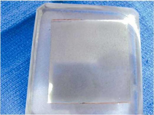
Fig. 86 Microsection made perpindicular to fracture surface at location 5 in fig. 20.
