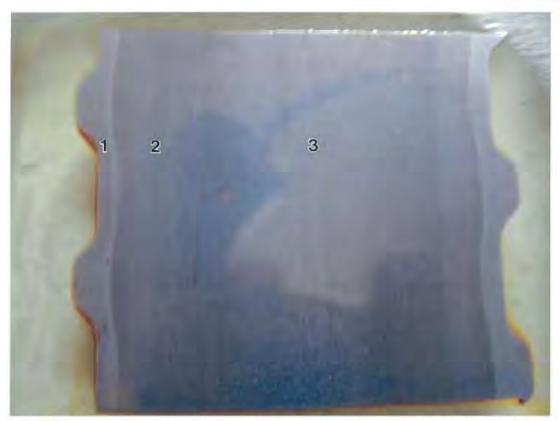
Fig. 43 Longitudinal cross-section of failed support rod from east span. Section taken out below fracture origin shown in fig. 15.
