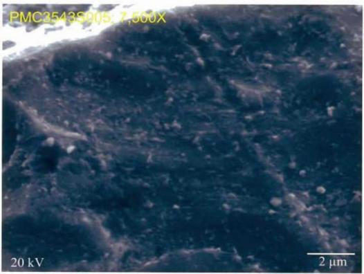
Fig. 54 S.E.M photo of eye bar fracture surface at fracture origin, in fig. 53. 7,500X.
