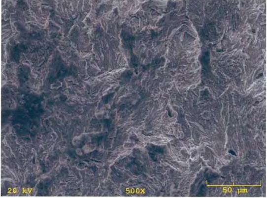
Fig. 36 S.E.M photo of failed support rod from east span at fracture surface. Fatigue. Zone 2. 500X.
