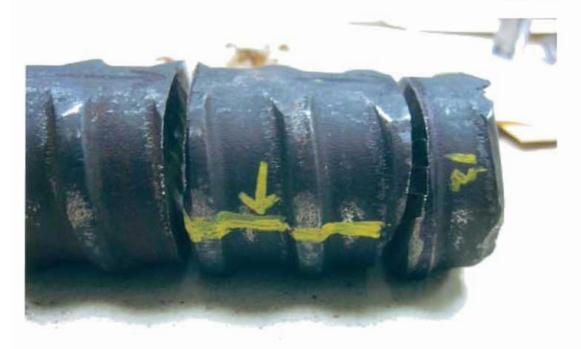
Fig. 15 As received failed support rod from east span. Location where longitudinal microsection was made.
