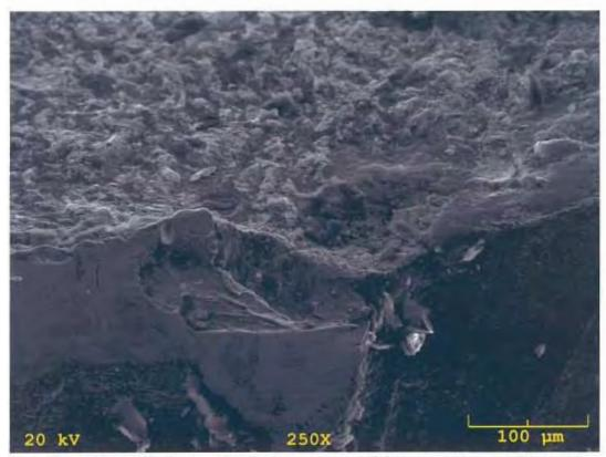
Fig. 27 S.E.M photo of failed support rod from east span. Edge, at fracture origin. 250X.
