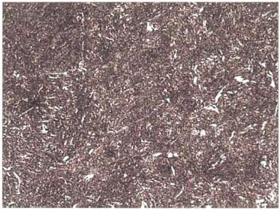
Fig. 44 Longitudinal cross-section of failed support rod from east span. Microstructure at location 1 in fig. 43. 500X. Etched.
