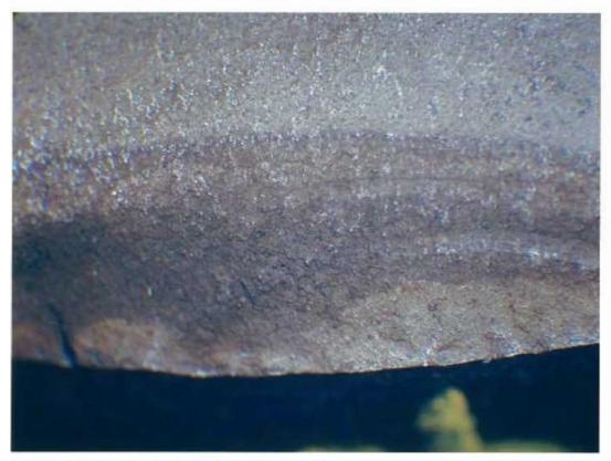
Fig. 19 As received failed support rod from east span. Fracture origin.
