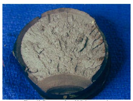
Figure 12: Fracture surface of failed support rod.
