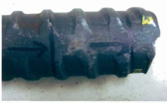
Fig. 14 As received failed support rod from east span. Location where longitudinal microsection was made.
