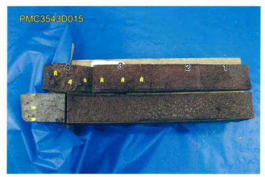
Fig. 35 Mating fracture faces.
