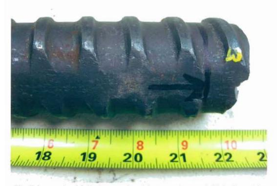
Fig. 7 As received failed support rod from east span. 3 O'clock position.
