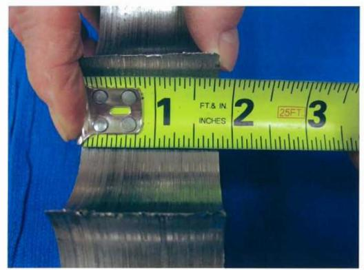
Fig. 17 Thickness of eye bar.
