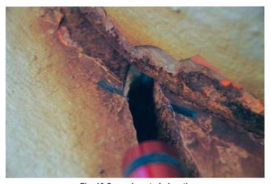
Fig. 10 Corrosion at pin location.
