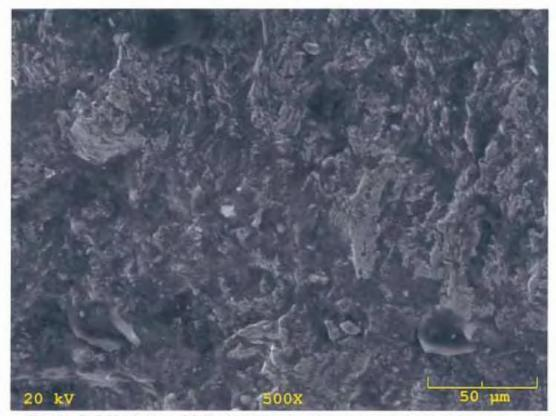
Fig. 29 S.E.M photo of failed support rod from east span at fracture origin. 500X.
