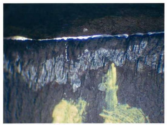
Fig. 21 As received failed support rod from east span. Fracture origin.
