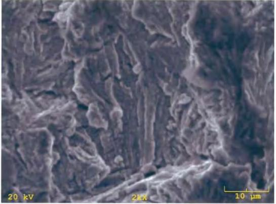
Fig. 38 S.E.M photo of failed support rod from east span at fracture surface. Fatigue. Zone 2. 2000X.
