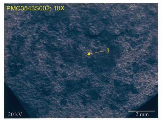
Fig. 55 S.E.M photo of eye bar fracture surface at fracture origin, location 1 in fig. 45. 10X.
