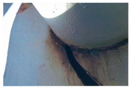
Fig. 9 Fracture at sleeve location.
