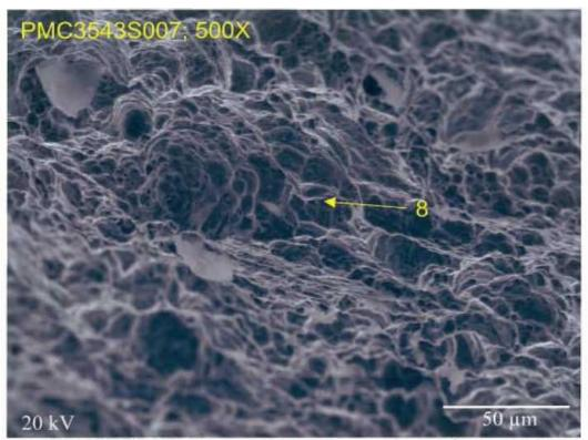
Fig. 47 S.E.M photo of eye bar fracture surface at fracture origin, in fig. 46. 500X.
