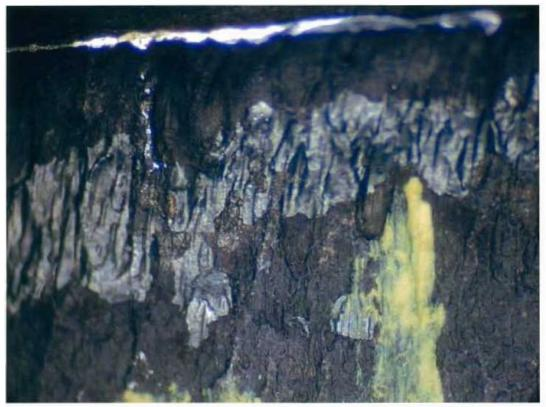
Fig. 22 As received failed support rod from east span. Fracture origin.
