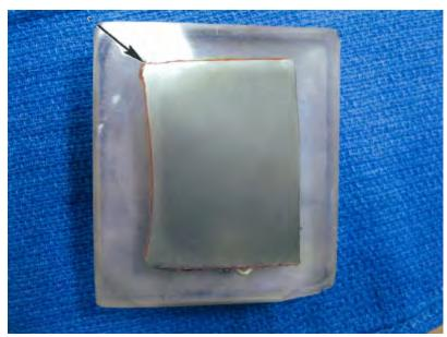
Figure 6: Microsection made below fracture surface. Arrow points to fracture initiation location.
