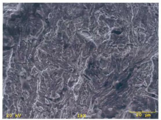
Fig. 37 S.E.M photo of failed support rod from east span at fracture surface. Fatigue. Zone 2. 1000X.
