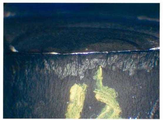
Fig. 20 As received failed support rod from east span. Fracture origin.
