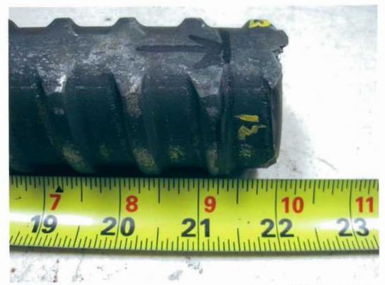
Fig. 2 As received failed support rod from east span. 12 O'clock position, fracture origin.
