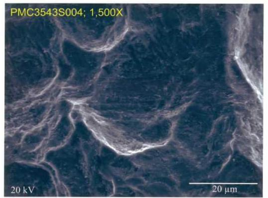
Fig. 53 S.E.M photo of eye bar fracture surface at fracture origin, location 4 in fig. 45. 1,500X.
