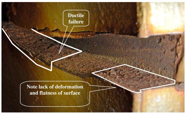
Figure 4: Close-up of the outer edge of the fracture
