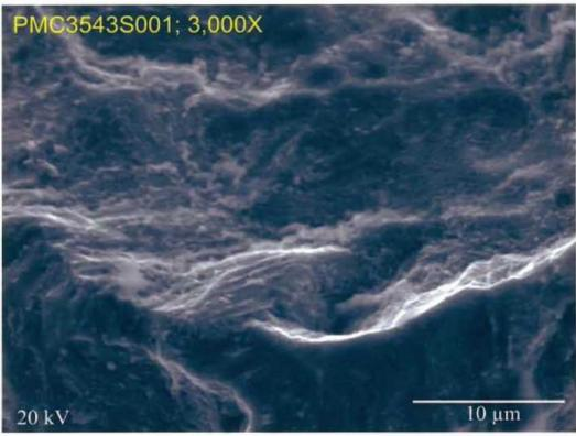
Fig. 56 S.E.M photo of eye bar fracture surface at fracture origin, location 1 in fig. 55. 3,000X.
