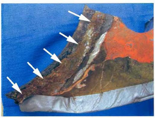
Fig. 12 Corrosion and wear at sleeve location.
