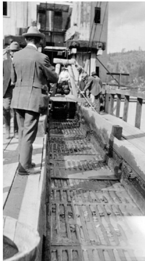
Figure 32: Trinity Dredge, Trinity County, 1922. View of sluice and manganese cast grid plates over Hungarian Riffles (used with permission, California Department of Conservation, California Geological Survey).
