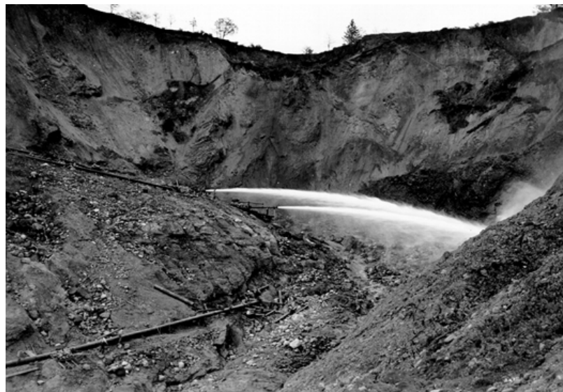
Figure 3: Hydraulic Mining at La Grange Mine, Trinity County, ca. 1940 (used with permission, California Department of Conservation, California Geological Survey).
