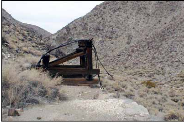
Figure 60: Tramway Header, Star of the West Mine, Inyo County (Courtesy JRP Historical Consulting Services).
