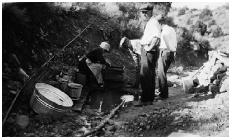
Figure 38: Woman using a Rocker, Kendon Pit, Mono County, 1930 (used with permission, California Department of Conservation, California Geological Survey).
