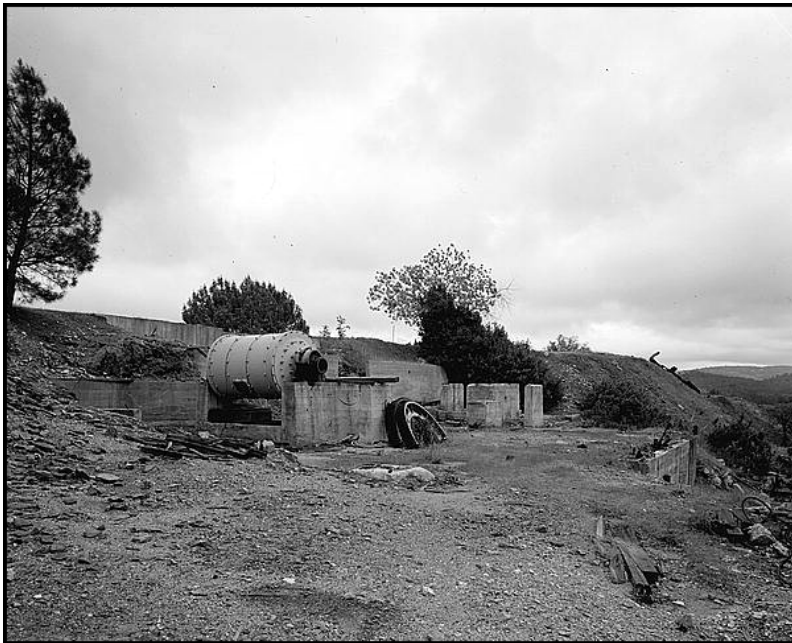
Figure 58: Hendy Ball Mill at Mountain King Mine (Library of Congress, HAER Photo by Alice Olmstead).
