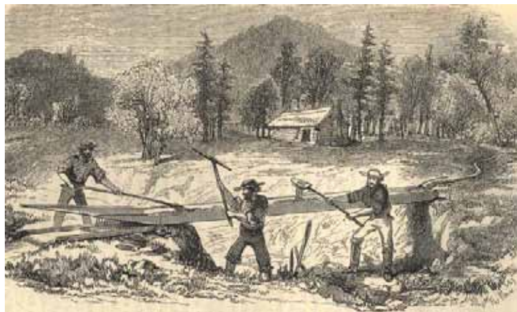
Figure 20: Working Gold Placers with a Long Tom or Sluice near Murphy's, Calaveras County, early 1850s (Courtesy George Wheeldon).
