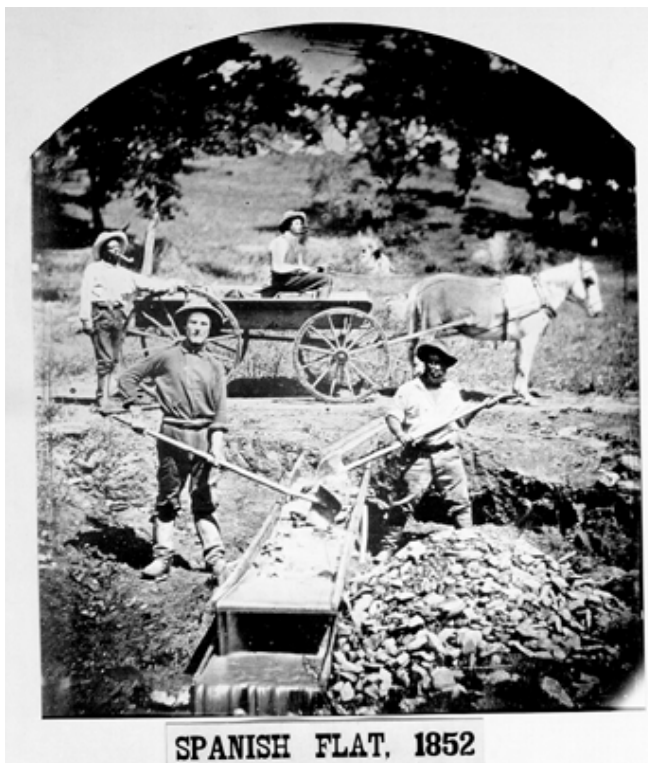
Figure 15: Gold Miners Running a Long Tom Sluice at Spanish Flat, El Dorado County (used with permission, California Department of Conservation, California Geological Survey).
