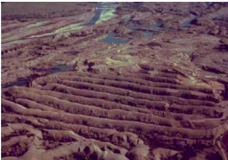
Figure 48: Bucket-line Dredge Tailings, Yuba River (courtesy Jim Woodward and Judith D. Tordoff).
