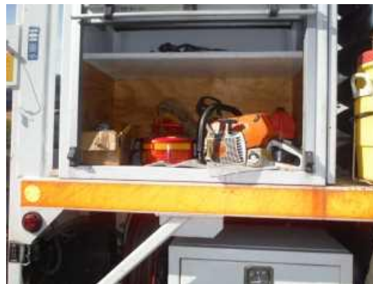
Drip pad under fuel can and tools used at pump house
