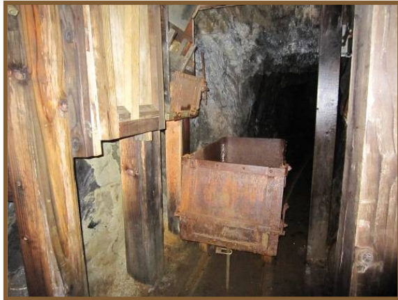
Figure 5-15: Ore car, tracks, and loading chute.
