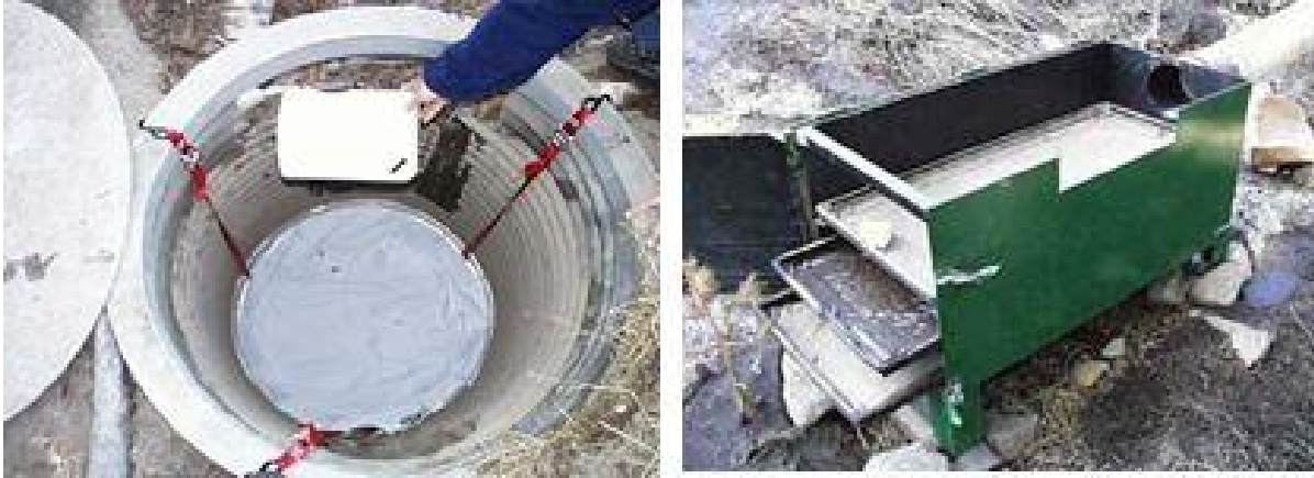
Figure 16-3 Barrel with Filter Bag (Left) and Trays (Right)
