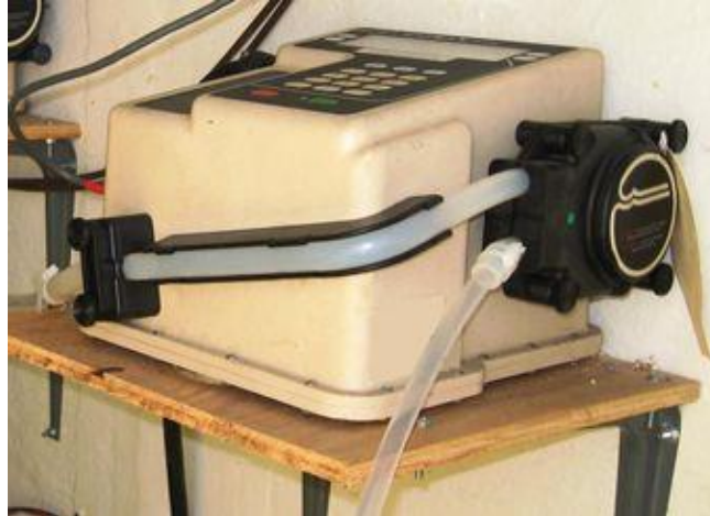
Figure 4-2 Automatic Sampler - Peristaltic Pump
