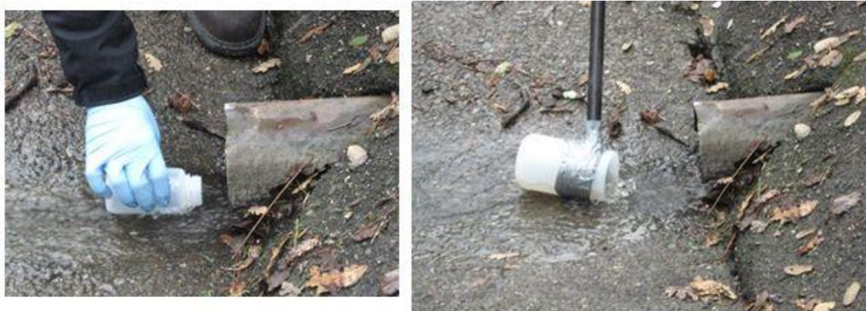
Figure 11-1 Collection of a Grab Sample by Hand (Left) and Using a Bailer (Right)
