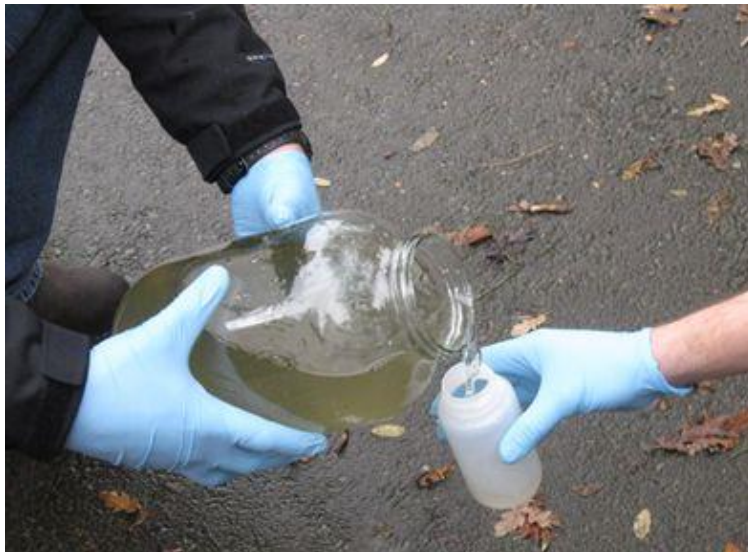
Figure 11-3 Sample Transfer from Intermediary Container to a Sample Bottle
