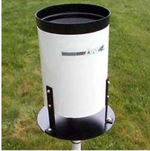
Figure 4-9 Tipping Bucket Rain Gauge
