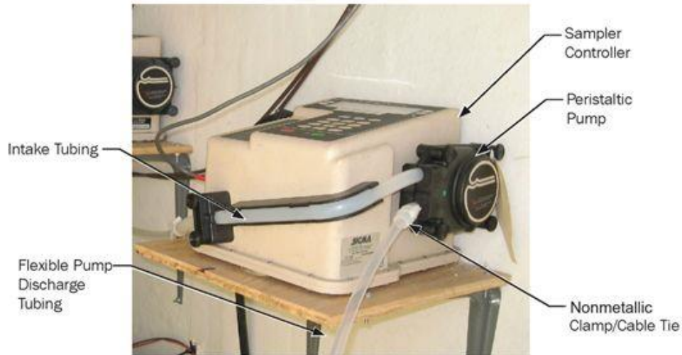
Figure 8-4 Autosampler with Tubing
