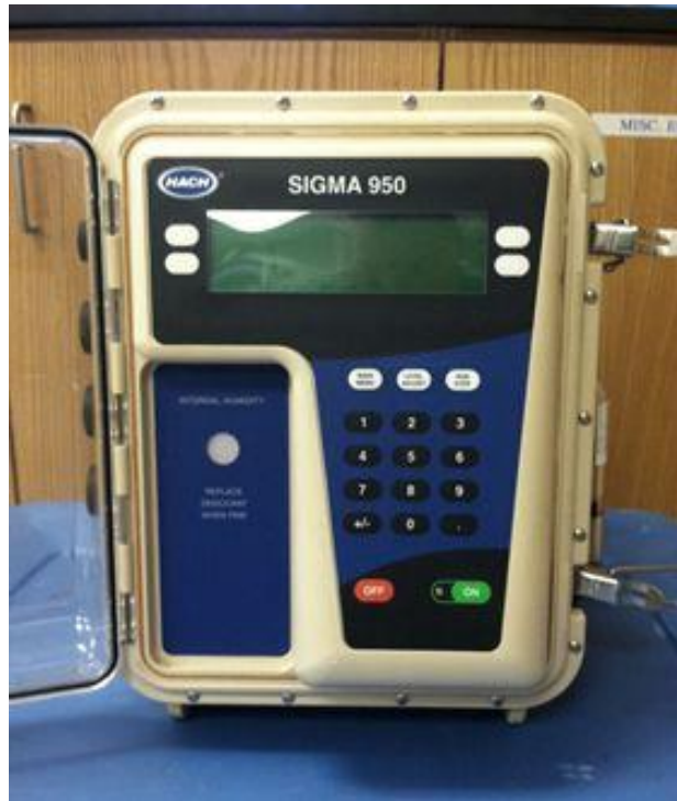
Figure 4-7 Flow Meter/Data Logger
