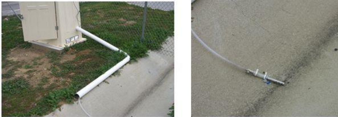
Figure 8-7 Sample Intake Tubing Running from Inside a Protective Enclosure to the Invert of a Stormwater Conveyance
