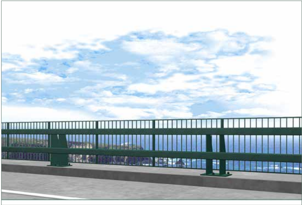
Rendering of California ST-10 Bridge Rail with sidewalk and steel pedestrian handrail at Noyo River Bridge on State Route 1 at Fort Bragg in Mendocino County. This is the barrier rail and pedestrian railing alternative that was ultimately chosen for the Noyo River Bridge. (01-MEN-001-PM 060.2)
