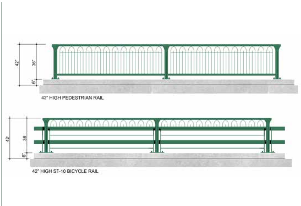
Renderings of decorative pedestrian rail for use on outside of bridge (top) and 42-inch-high vehicular/bicycle rail for use between sidewalk and roadway (bottom).
