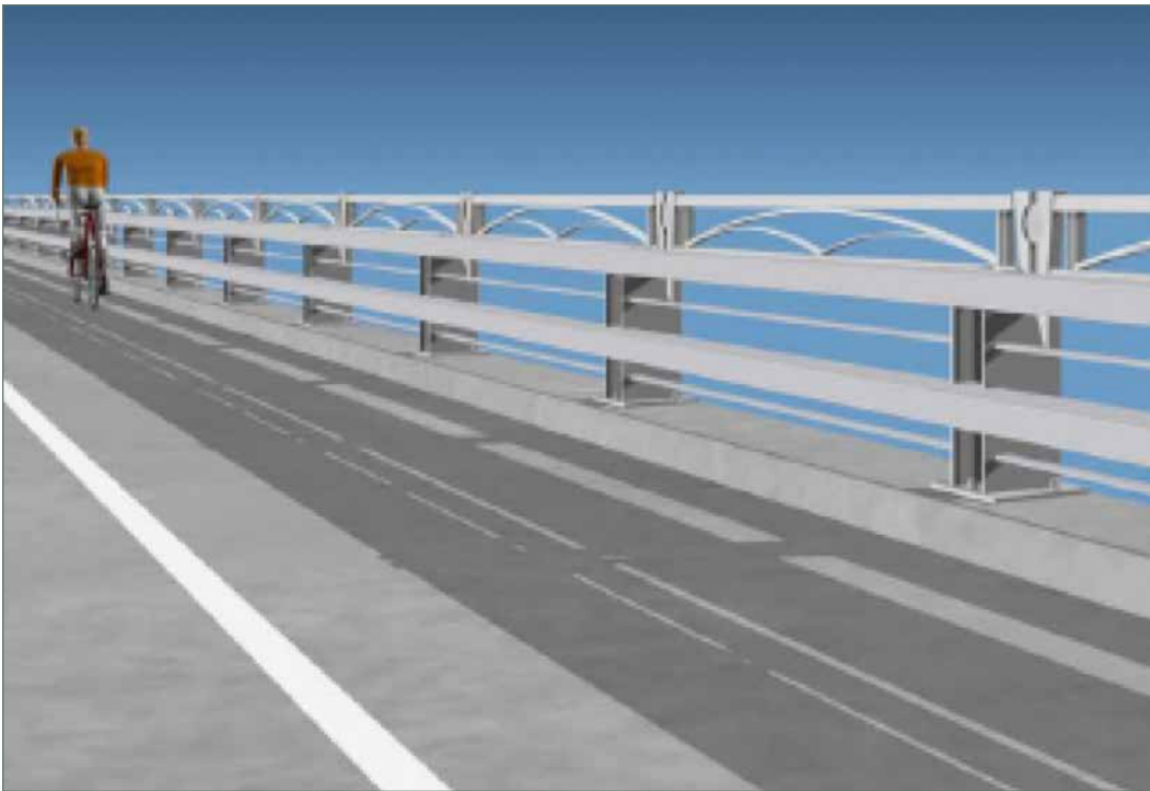
Rendering of 42-inch-high California ST-10 Bicycle Rail with decorative double arch option. Note cables added to reduce clear openings between ST-10 rails as required when bicycle traffic is expected. This is the bicycle rail alternative design that was ultimately chosen for the Ten Mile River Bridge in Mendocino County. (01-MEN-001-PM 069.7)
