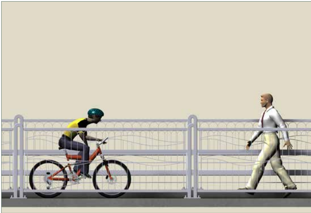
Looking east from ocean toward U.S. 101 in Ventura County. Rendering of 48-inch-high pedestrian rail / walkway-bikeway / California ST-10 Bridge Rail with 54-inch-high access control rail. La Conchita project (07-VEN/SB-101).
