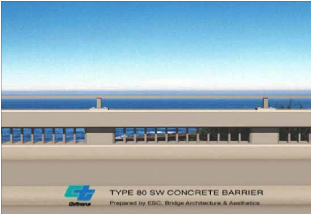
Rendering of a proposed alternative Concrete Barrier Type 80SW on the Noyo River Bridge in Mendocino County. (01-MEN-001-PM 60.2)
