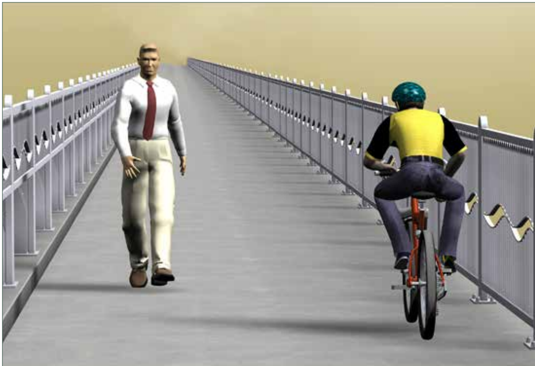
Looking south along combination walkway-bikeway (ocean side of U.S. 101 in Ventura County). Rendering of 48-inch-high pedestrian-bicycle rail on the right and California ST-10 Bridge Rail with 54-inch-high access control rail on the left. La Conchita Project (07-VEN/SB-101).
