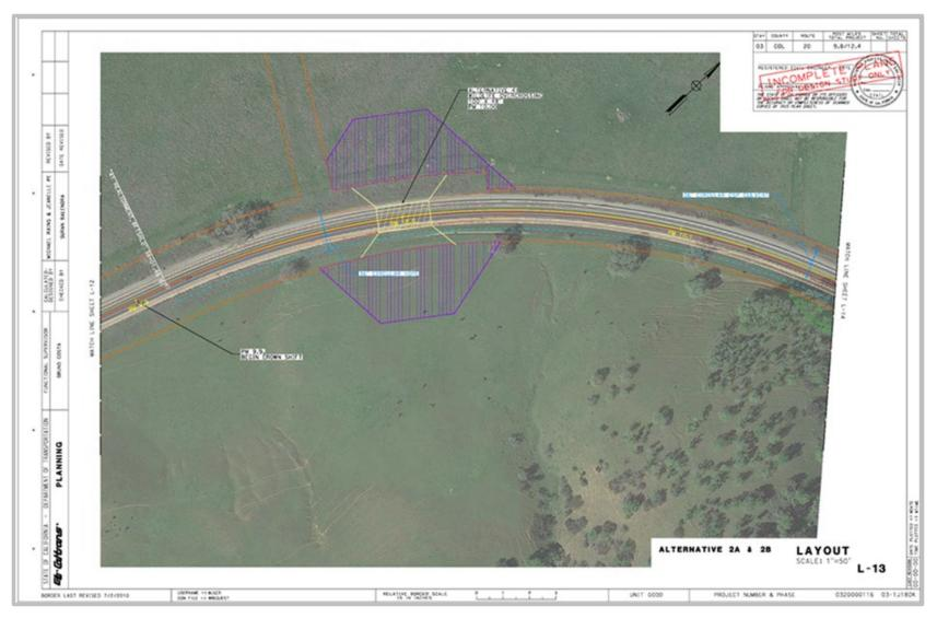
**Appendix Figure 1.** Preliminary scoping map used at the beginning of the design phase. This shows the initial placement of the overcrossing to be used by Caltrans Structures & Design Team as a rough estimate location.
