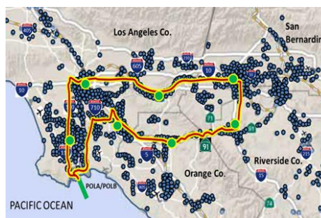
137-Mile Freight Pipeline Route. Pipeline feeder terminals are the Green dots. Blue dots show port related consolidation warehouse clusters.
