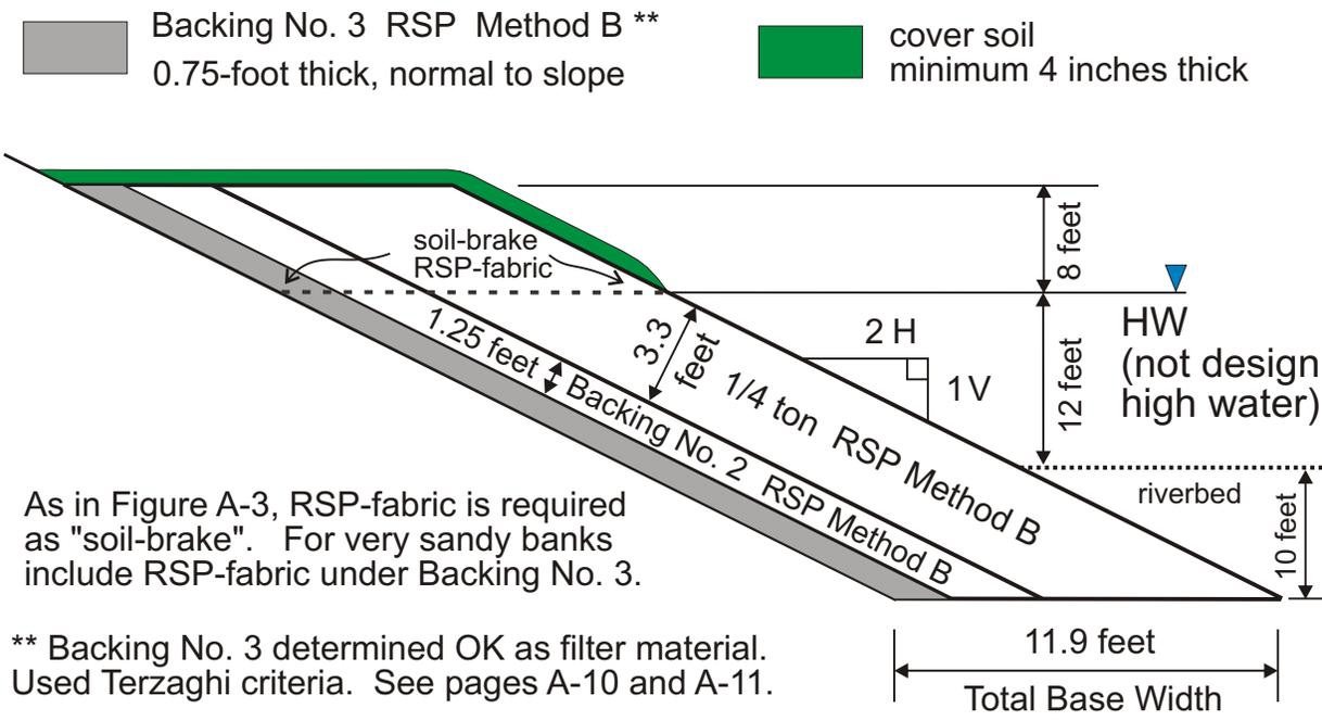
**Figure A-7. CA Layered RSP with EMBEDDED Toe** Cross-section No Scale US units Not a Standard Plan
