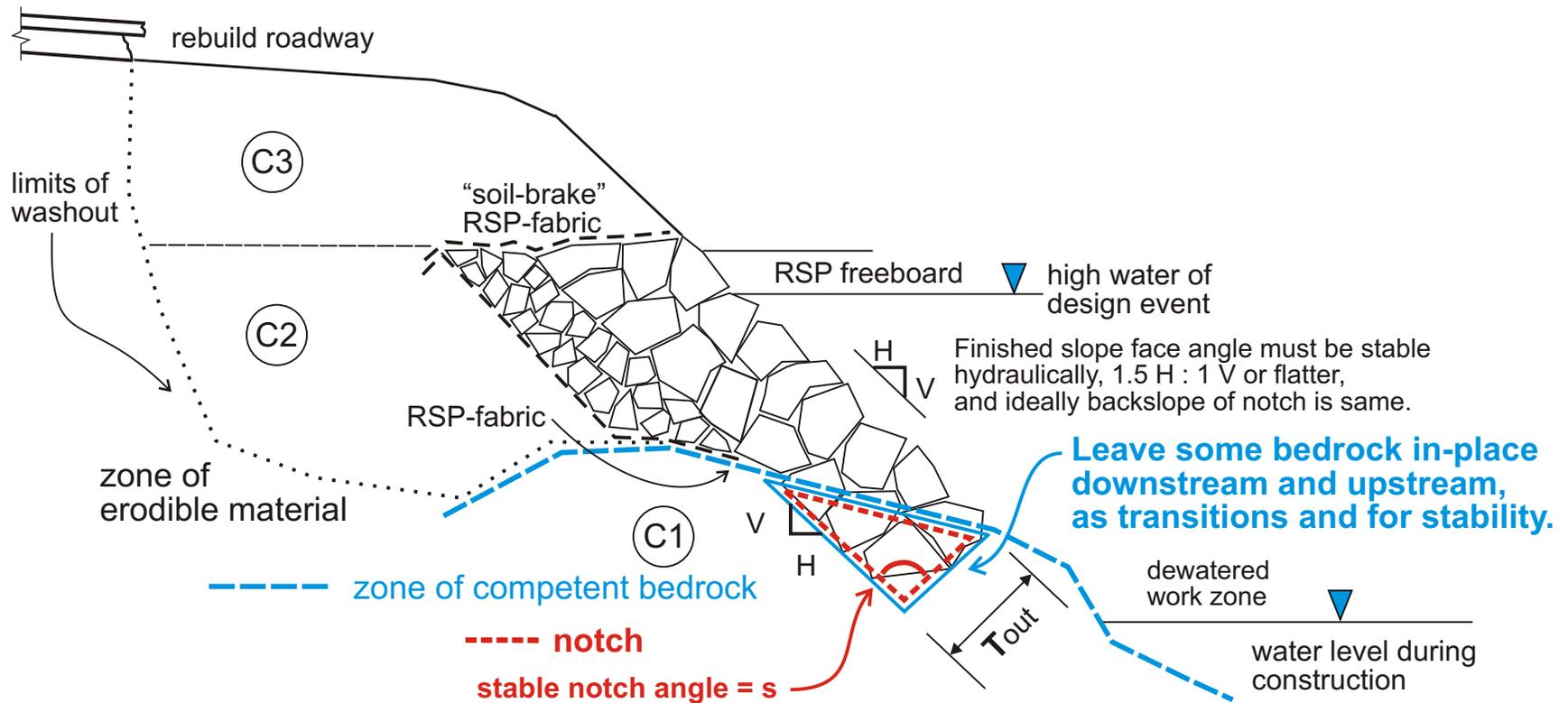
1. When bedrock dips toward stream, construct notch for stable RSP toe in zone of competent bedrock C1.
