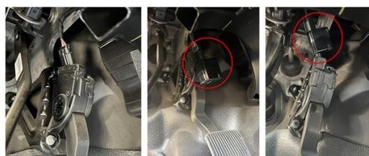
Image 2: Left to right: Electronic accelerator pedal without SmartPedal™ installed, SmartPedal™ connected to accelerator pedal wire harness connection, SmartPedal™ installed inline between accelerator pedal and accelerator pedal wire harness connection.
