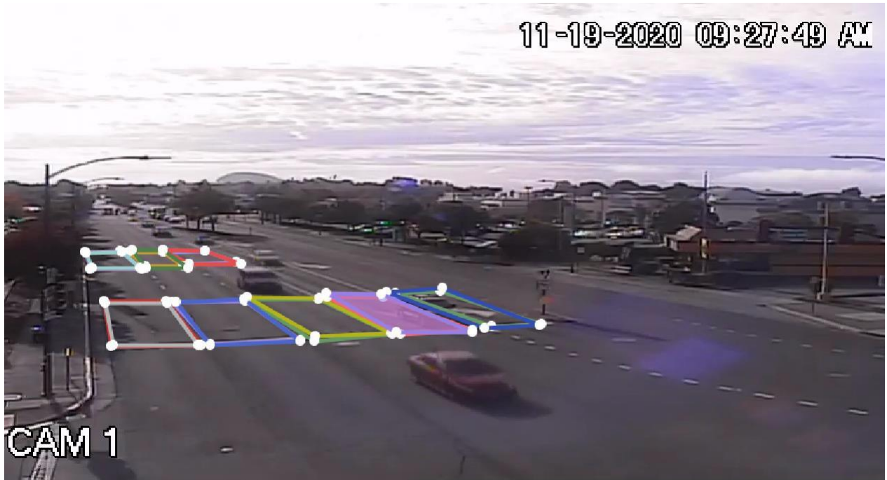
Figure 6 - Northbound approach of intersection with detection zones
