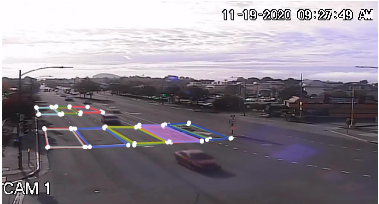
Figure 31 - Traffic video of the signalized intersection with detection zones in VideoSync
