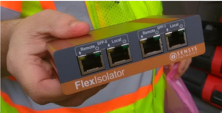
Figure 21 - Sensys Flex isolator unit
