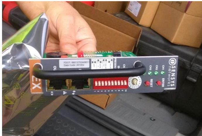
Figure 23 - Sensys contact closure card
