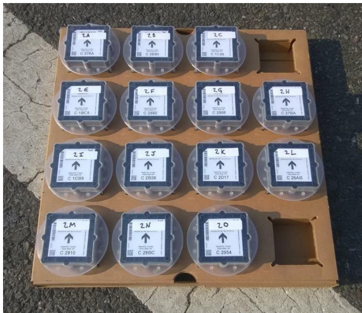
Figure 9 - Sensys wireless magnetometers ready for installation
