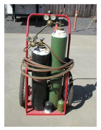
Figure 3-10. Oxyacetylene Torch Setup
