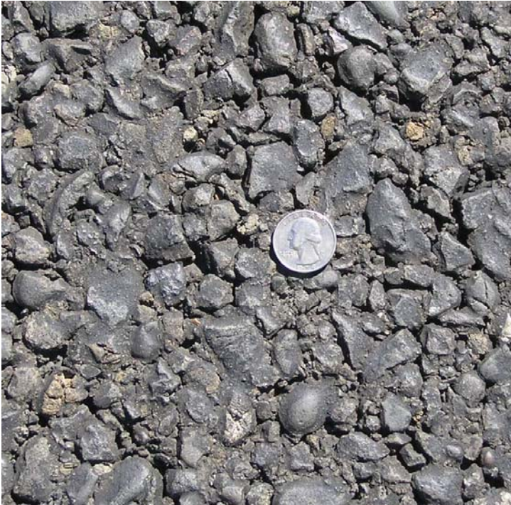
Figure 14: Rubberized open-graded asphalt concrete F-mix (RAC-O F-mix).
