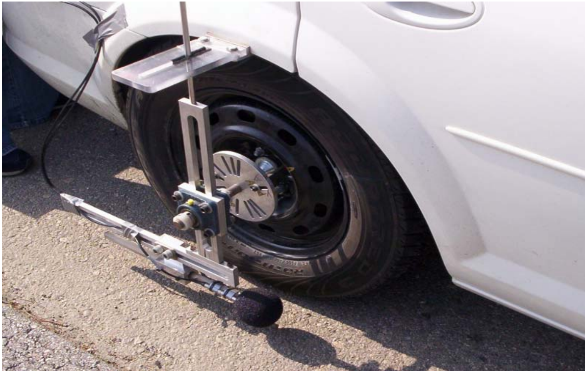
Figure 21: On-board sound intensity (OBSI) microphone setup.
