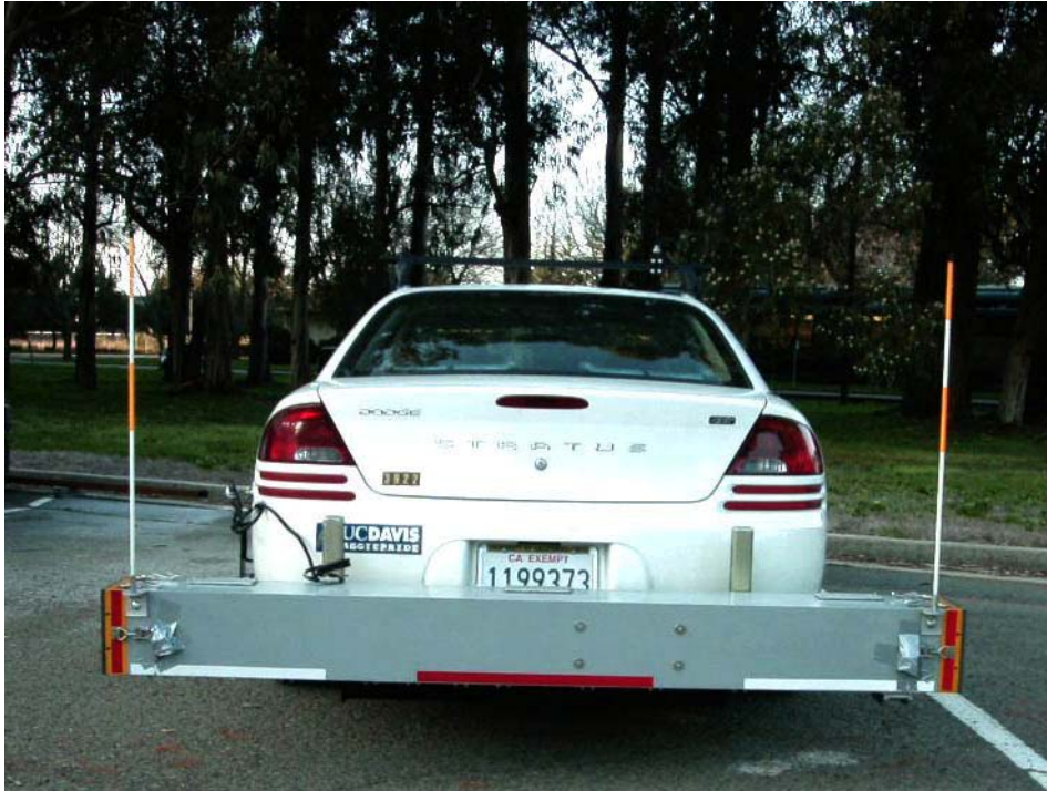
Figure 22: Laser profilometer beam.
