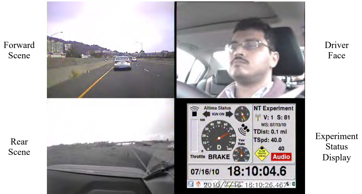
Figure 3.2: Video Acquisition System Output Image.
