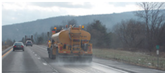
Image 2: Brine tank truck spreading salt brine on roadway
