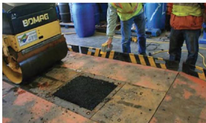
Figure 1: HMA materials being compacted in the laboratory for testing
