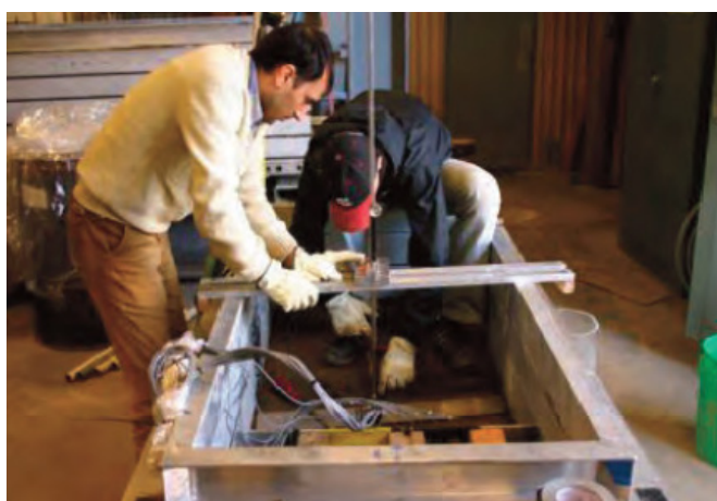
Figure 2: Construction of sloping backfill model
