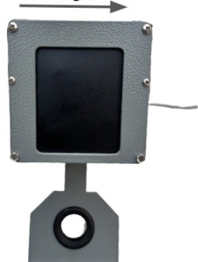
Image 4: MS Sedco Smartwalk XM pedestrian detector as mounted for testing
