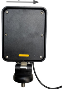
Image 3: AGD 326 pedestrian detector as mounted for testing
