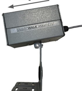
Image 4: MS Sedco Smartwalk XM pedestrian detector as mounted for testing
