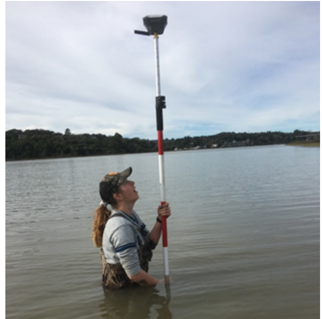
Image 1: Determining precise elevation of pressure sensors deployed.
