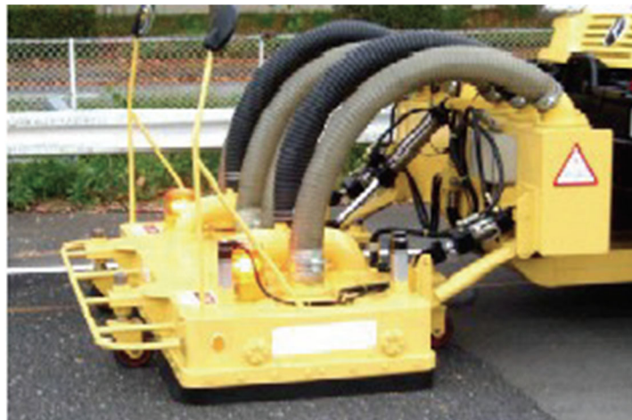
Figure 5.5: High-pressure air with vacuuming equipment used to remove clogging of OGFC surface pavements in Japan. (Source: Nielsen 2005)
