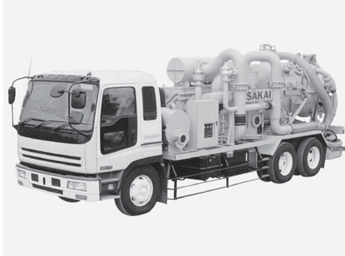
Figure 5.4: Truck-mounted high-pressure water washing and vacuuming equipment used for OGFC cleaning in Japan. (Source: Nielsen 2005)
