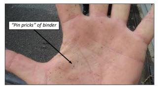
Figure 6.45: Good dispersion of foamed asphalt.
