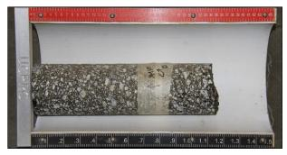
Figure 2.49: Core from digout showing 1.15-ft thick asphalt concrete layer.
