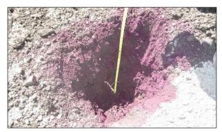
Figure 6.47: Checking cement mixing depth on an FDR-C project (note crimson color).
