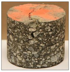
Figure 2.41: Top-down thermal crack.
