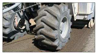
Figure 6.39: Normal tire condition when nozzles are functioning correctly (FDR).
