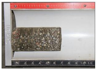
Figure 2.40: Core measurement.
