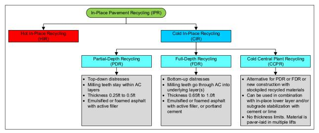
Figure 1.1: Hierarchy of in-place pavement recycling terminology.
