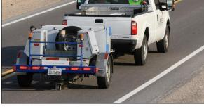
Figure 2.53: Falling weight deflectometer, vehicle mounted.
