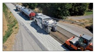
Figure 1.5: Full-depth recycling train (wheel).
