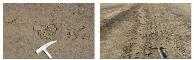
Figure 6.102: Delamination after blading thin lifts of material during grading (FDR).
