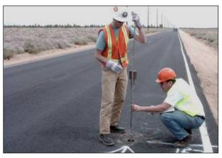
Figure 2.52: DCP test.
