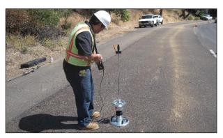
Figure 6.116: Checking stiffness reduction with a light weight deflectometer.
