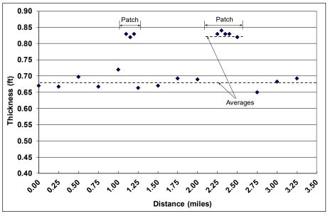
Figure 2.51: Example layer thickness analysis from cores.
