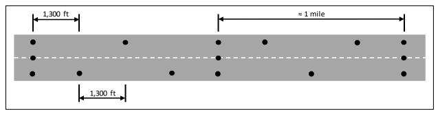
Figure 2.39: Suggested minimum coring plan (example for 2-mile section of a 2-lane project).
