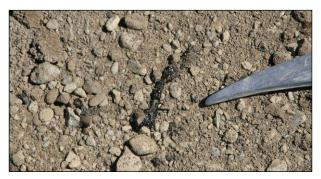
Figure 6.42: Unfoamed binder in recycled material on an FDR-FA project.
