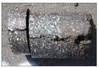
Figure 2.42: Bottom-up fatigue/reflected crack.
