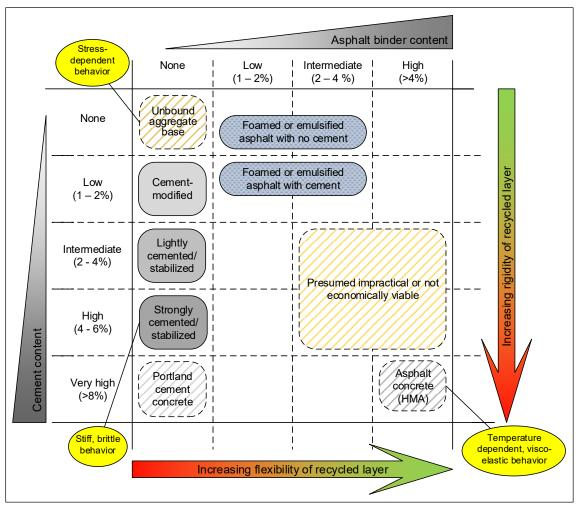
Figure 3.10: Basic characteristics of in-place recycled pavement materials (18).
