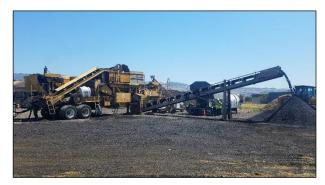
Figure 6.11: Cold central plant using processing unit from a multi-unit recycling train.
