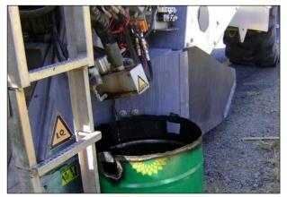
Figure 6.26: Nozzle for checking binder foaming characteristics.
