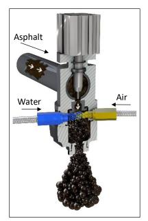
Figure 5.1: Recycler foam nozzle.
