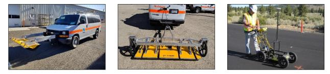
Figure 2.55: Ground penetrating radar systems.
