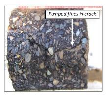
Figure 2.47: Pumping of fines through cracks.
