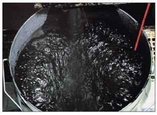
Figure 5.5: Determining expansion ratio and halflife of asphalt binder.
