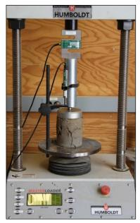
Figure 5.9: Unconfined compressive strength test.
