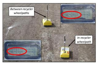
Figure 6.90: Density measurements in and between recycler wheelpaths (FDR).
