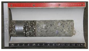
Figure 2.44: Asphalt on cement-treated base.
