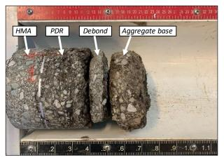
Figure 2.46: Thin debonded layer below PDR layer.
