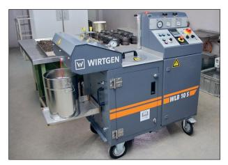
Figure 5.4: Laboratory foaming equipment.
