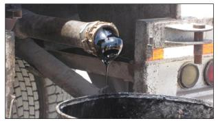
Figure 6.48: Cold plug in the asphalt feed connection of a binder tanker.
