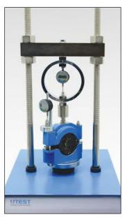
Figure 5.2: Marshall Stability Test.
