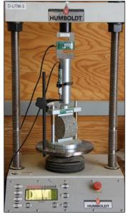
Figure 5.3: Indirect Tensile Strength Test.
