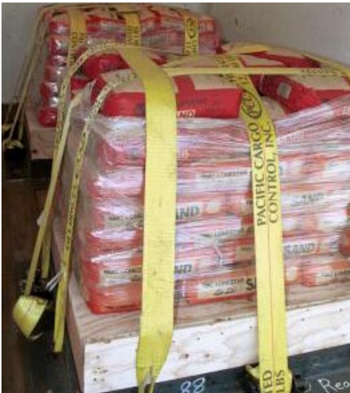
Figure 2-20 Ballast strapped down in cargo bed of test vehicle after Test 572
