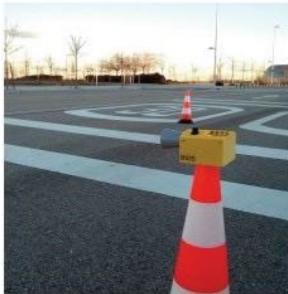
Figure A.3 Photo of WSN Sensor Node During Closed Track Testing (Source: Martin et al., 2016)
