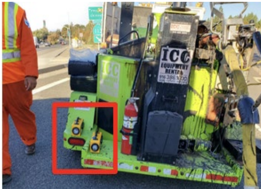
Figure 5.41 Placement of WAS Alarm Units on Rear of Equipment Vehicle
