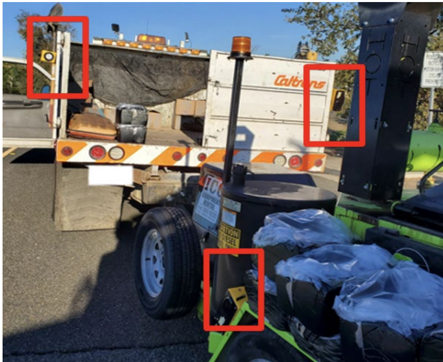
Figure 5.40 Placement of WAS Alarm Units on Side of Equipment Vehicle
