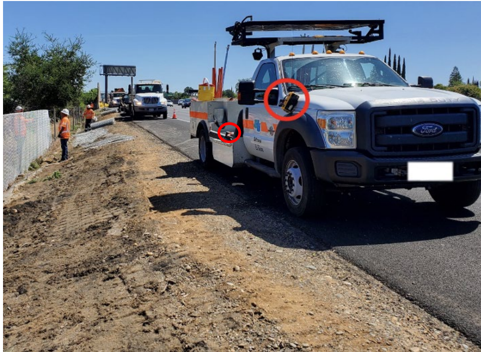
Figure 5.3 Location of WAS Alarm Units on Vehicles Near Activity Area
