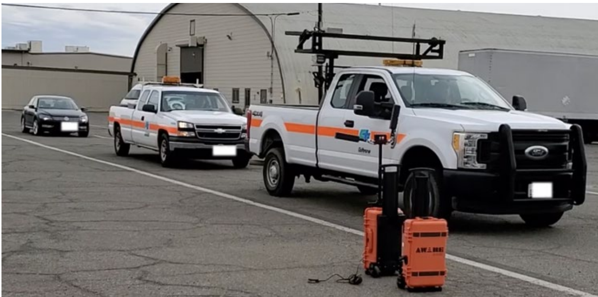
Figure 4.7 AWARE Sentry Setup and Vehicle Out of Queue Test
