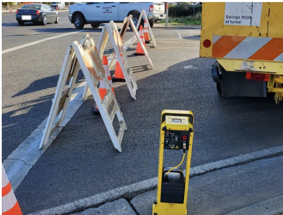
Figure 5.33 Deployment Location of Single Sentry Beam Unit Behind Shadow Truck
