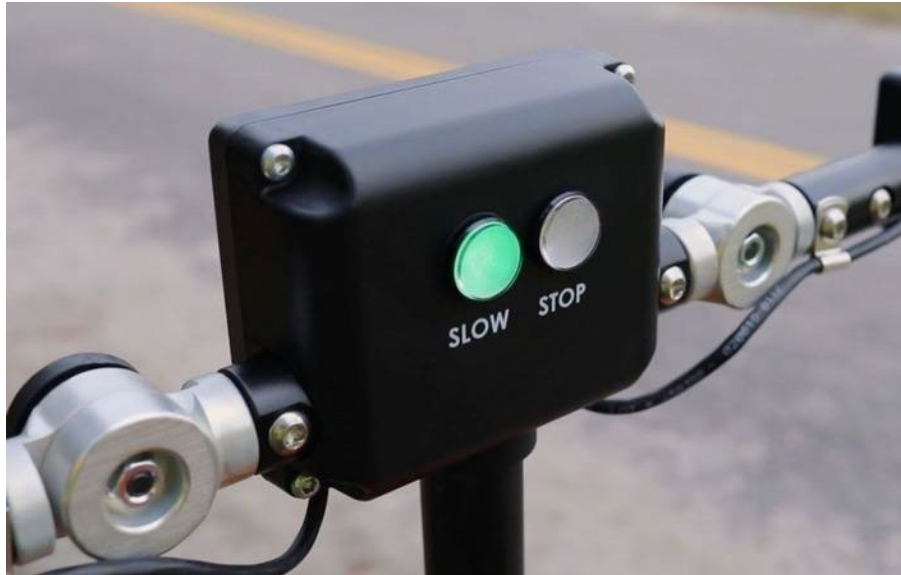
Figure E.18 Back View of AWARE Sentry Device When Pedal is Pressed
