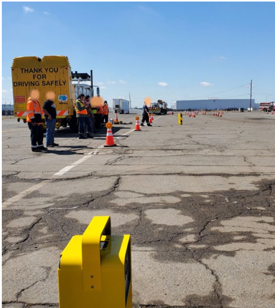
Figure 4.4 Single Sentry Beam Detection Range Test
