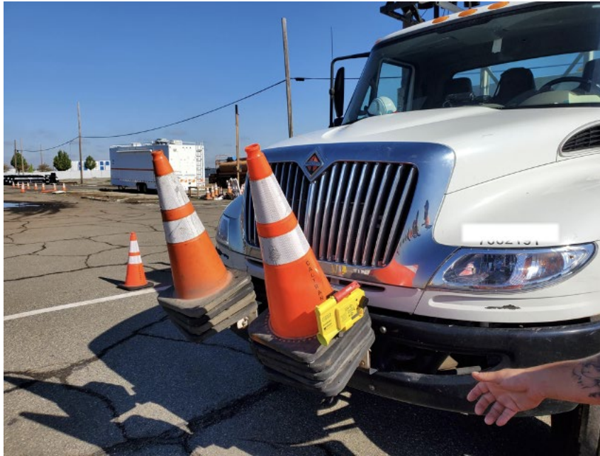
Figure 4.6 SonoBlaster Cone Stacking and Deployment from Shadow Truck
