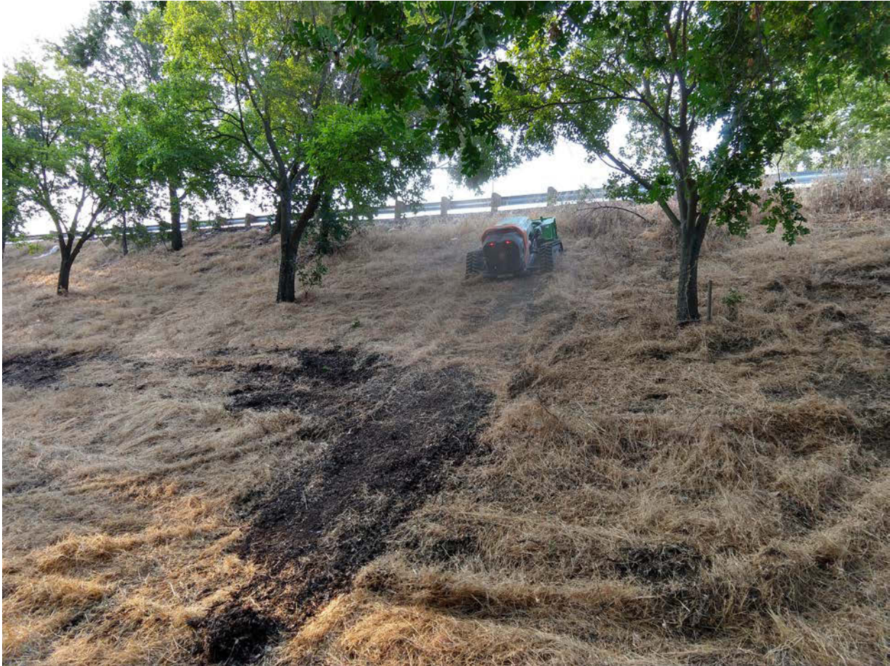
Figure 5.5: LV600 tested by researchers on 2:1 (27°) slope
