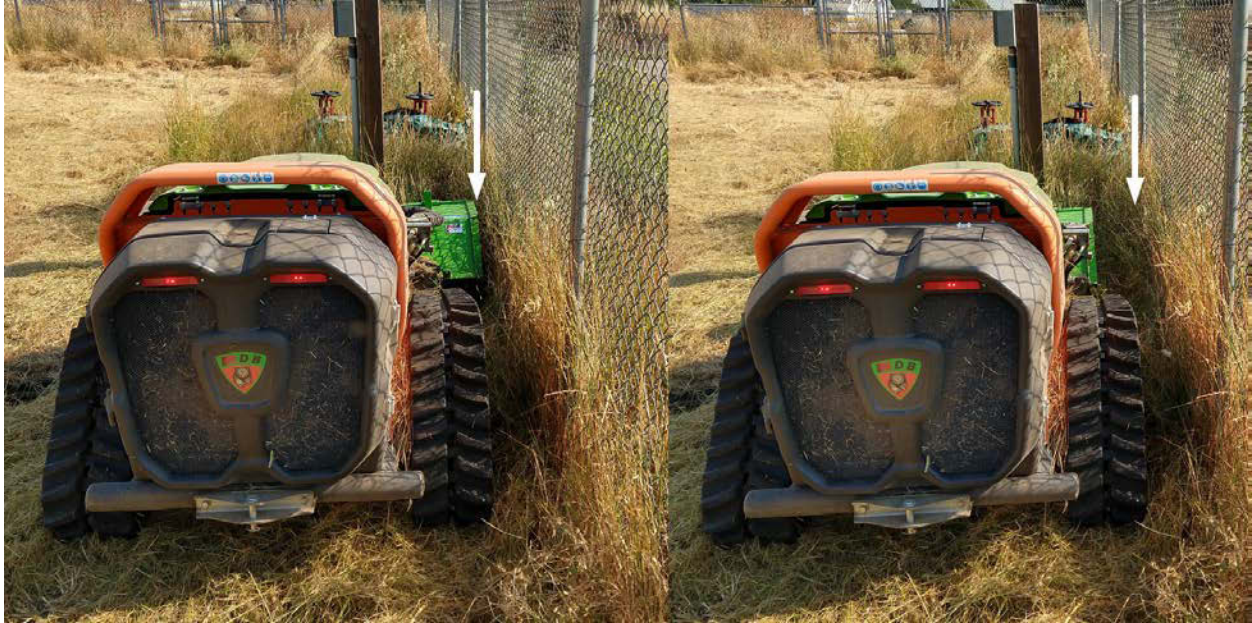
Figure 5.3: LV600 cutter head shift function
