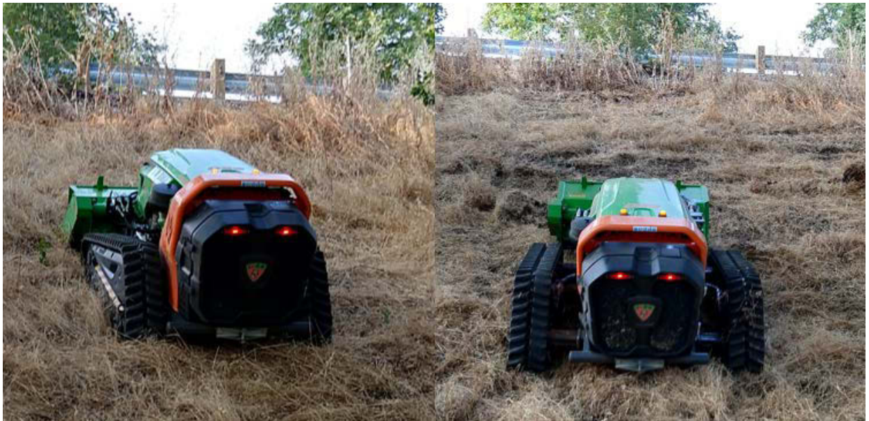
Figure 5.4: LV600 track widening function
