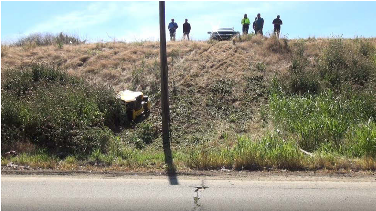
Figure 5.11: Spider mower tethered to truck at top of levee
