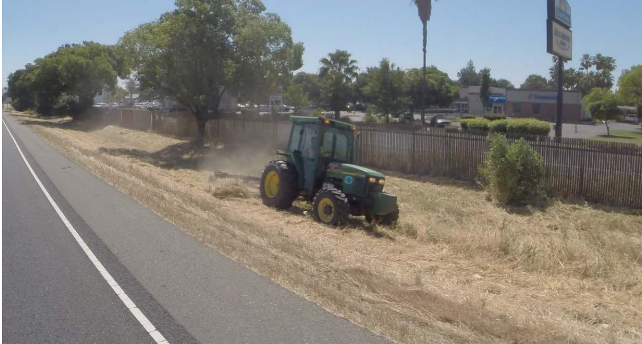
Figure 4.6: Tractor pulling a 9-ft-wide mower
