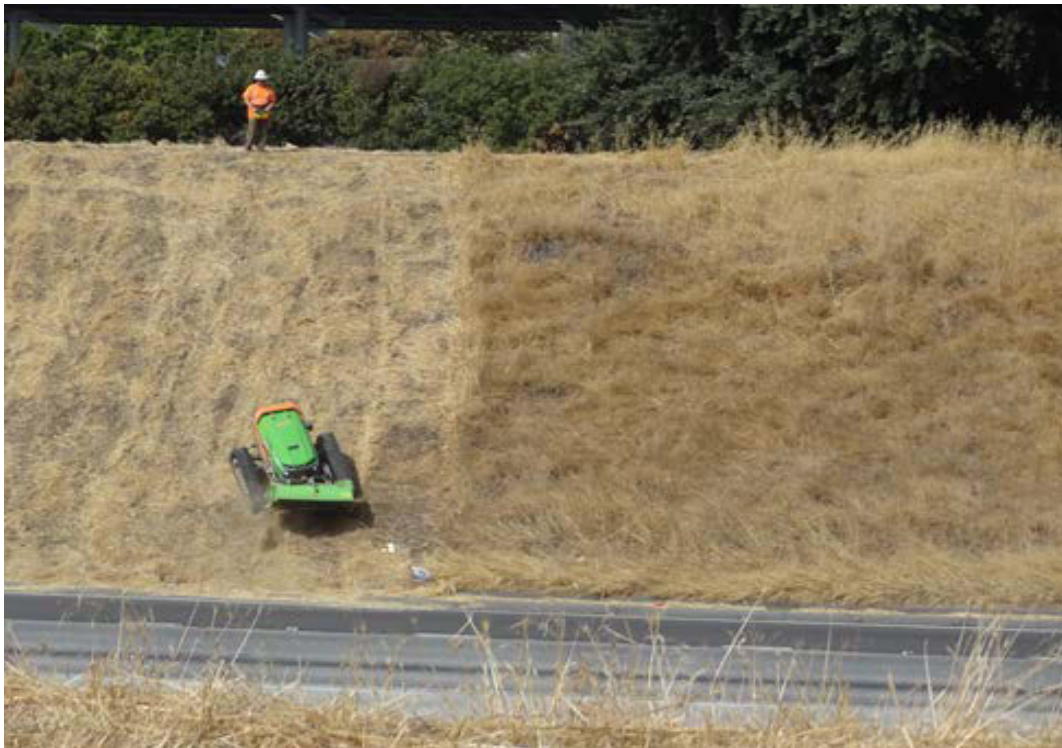
Figure 5.9: Backing up the slope with cutter head raised
