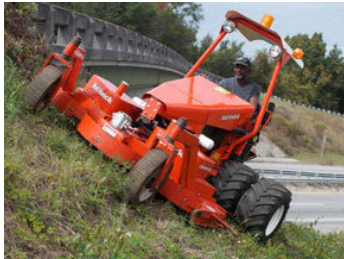
Figure 2.2: Kut Kwick Slope Master manned mower
