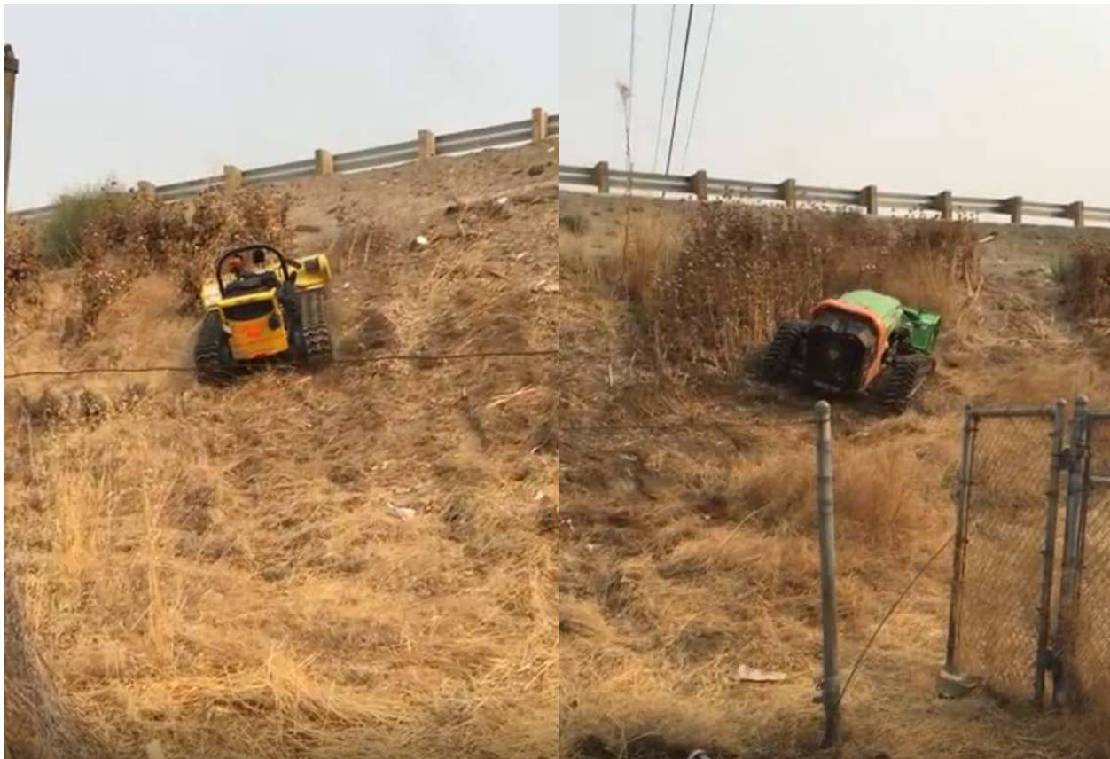
Figure 5.10: Traxx and LV600 operated in same area by one operator
