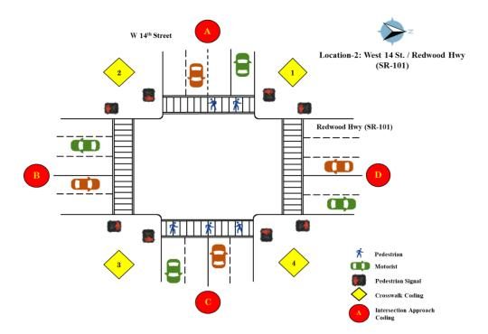
Figure 15: Schematic Coding of Location 2: West 14 St. / Redwood Hwy, Eureka for Data Recording
