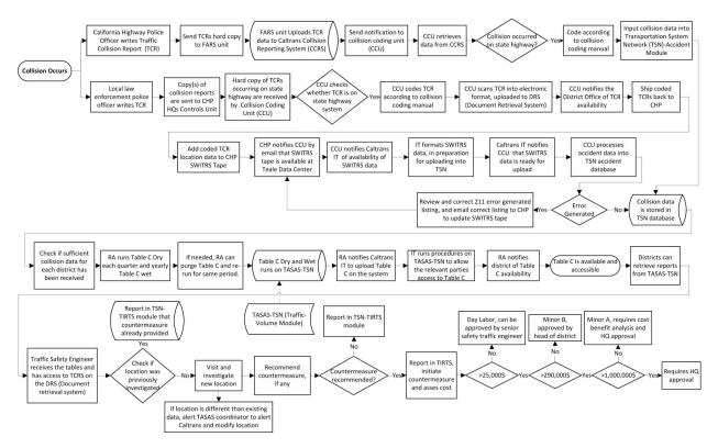
Figure 3.6 Flowchart map developed for Table C production
