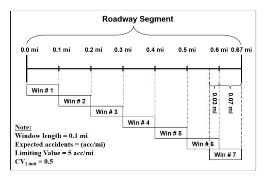
Figure 4.4 Schematic diagram of the Peak Searching approach
