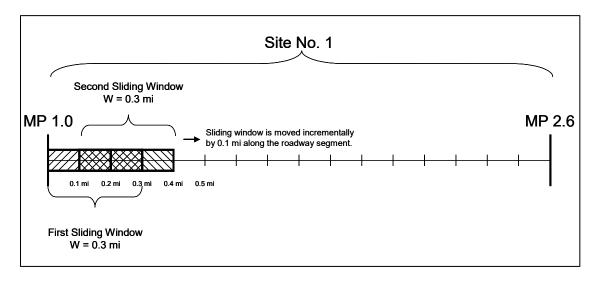
Figure 4.3 Schematic diagram of the Sliding Window approach
