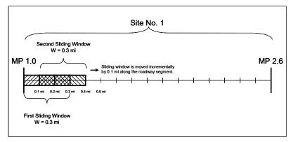
Figure 2.3 Schematic diagram of the sliding window method of network screening
