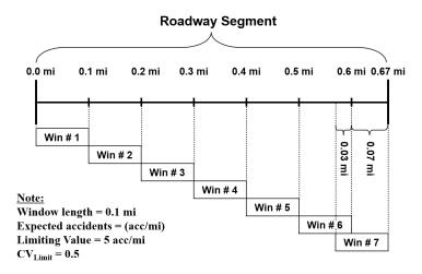
Figure 2.4 Schematic diagram of the peak searching method
