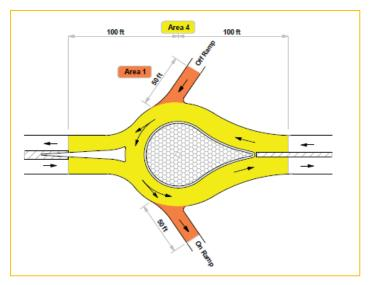
Figure C.4. Ramp location code for roundabouts.
