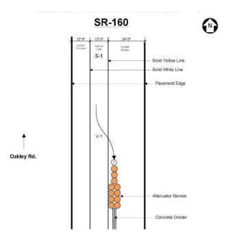
Figure B.4: Example of complexity in lane identification when objects are on the highway.
