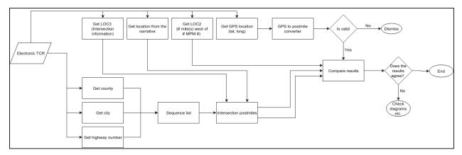
Figure C.7. Flow chart of retrieving specific fields of data needed to calculate post-mile data.
