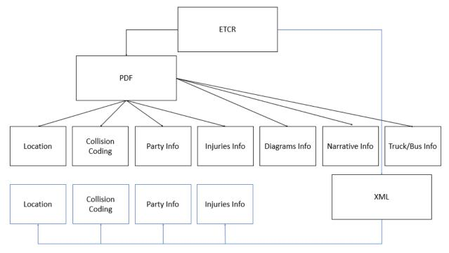
Figure C.9. ETCR data extraction method; XML file is only used to verify field data.
